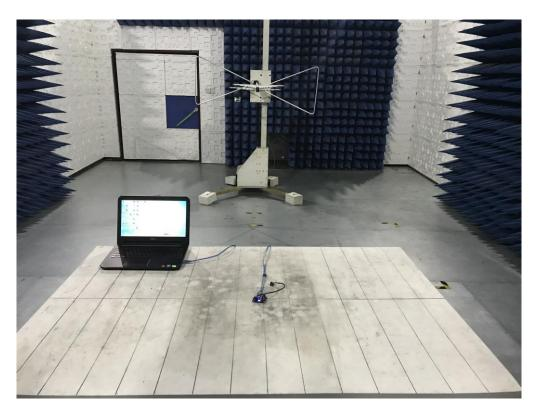
FCC RADIATED EMISSION TEST SETUP ABOVE 1GHZ
