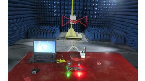
RADIATED EMISSION TEST
