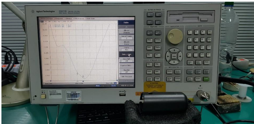
Figure 4.2.1 Test by network analyzer
