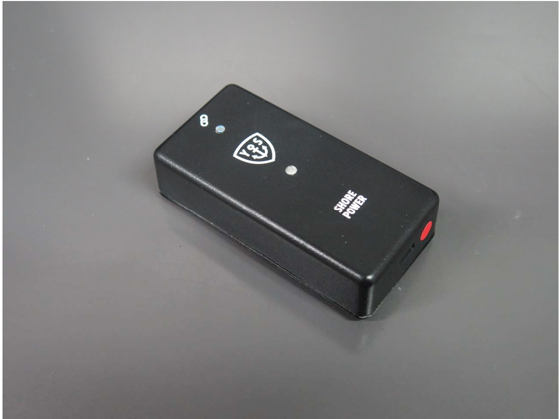
Shore Power Sensor
