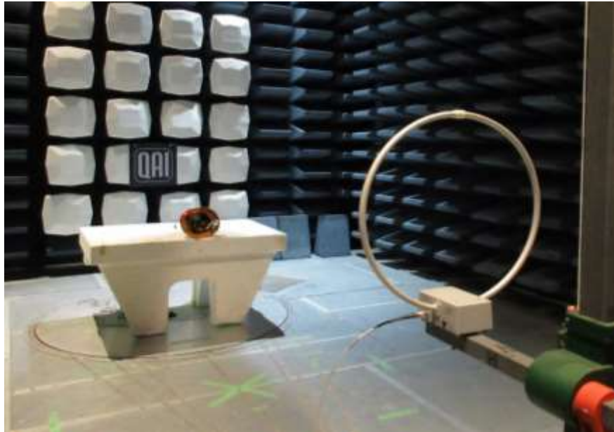
Figure 1: Radiated Emissions (150kHz – 30 MHz) performed at the SAC Test Setup
