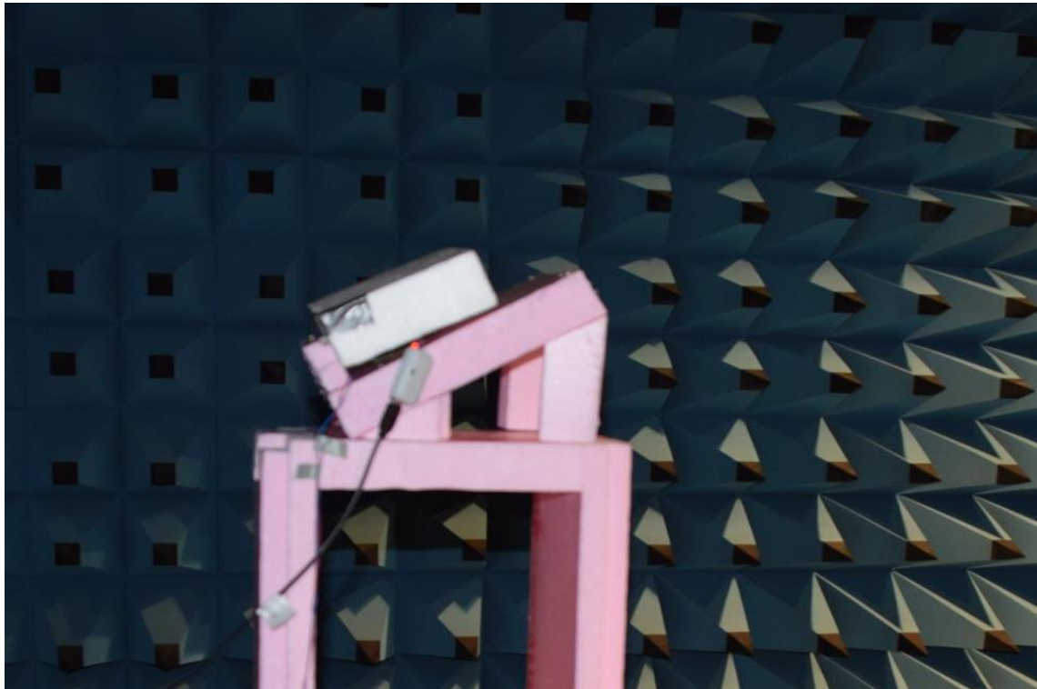
Picture 11: EUT 30° (150°) elevation for the measurements in the 960 MHz to 40 GHz range
