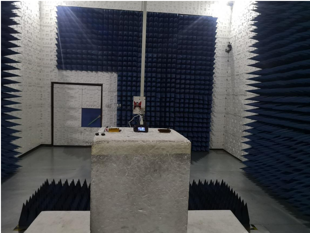
RADIATED EMISSION TEST SETUP ABOVE 1G
