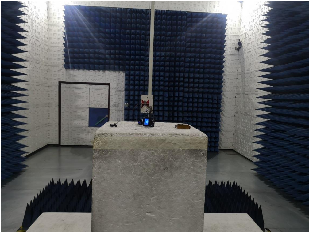
RADIATED EMISSION TEST SETUP ABOVE 1G
