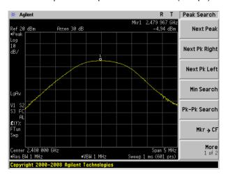
Peak output Power plot on channel 00 (2Mbps)
