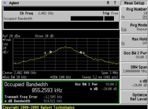
20dB Bandwidth plot on channel 39 (1Mbps)
