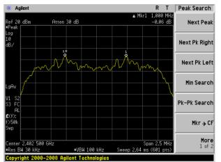
(1Mbps) Channel Separation plot on channel 39-40
