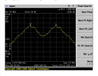
(2Mbps) Channel Separation plot on channel 77-78
