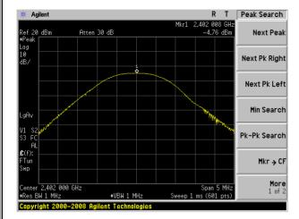
Peak output Power plot on channel 39 (1Mbps)
