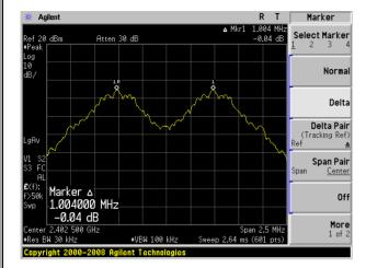
(2Mbps) Channel Separation plot on channel 00-01
