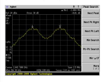
(2Mbps) Channel Separation plot on channel 39-40
