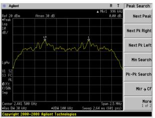
(1Mbps) Channel Separation plot on channel 77-78
