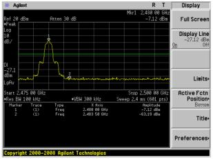
π /4-DQPSK: Band Edge-High Channel (Hopping Mode)
