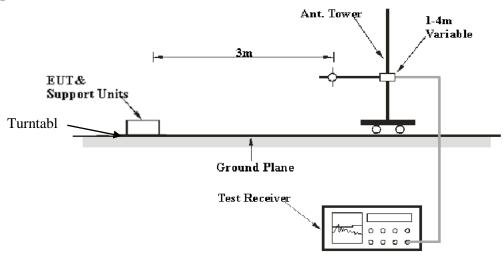
The radiated emission tests were performed in the 3-meter chamber test site, using the setup accordance with the ANSI C63.10-2013. The specification used was the FCC Part Subpart C limits.
