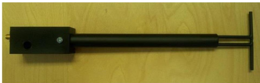
Figure 1 – MVG COMOSAR Validation Dipole
