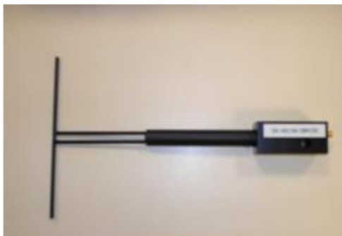
Figure 1 – Satimo COMOSAR Validation Dipole
