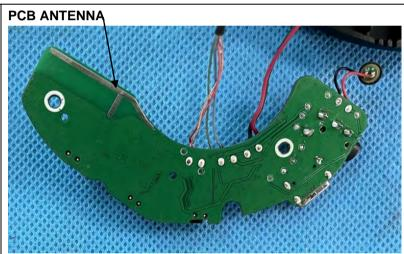
The antenna is integral antenna. The best case gain of the antenna is 0dBi.
