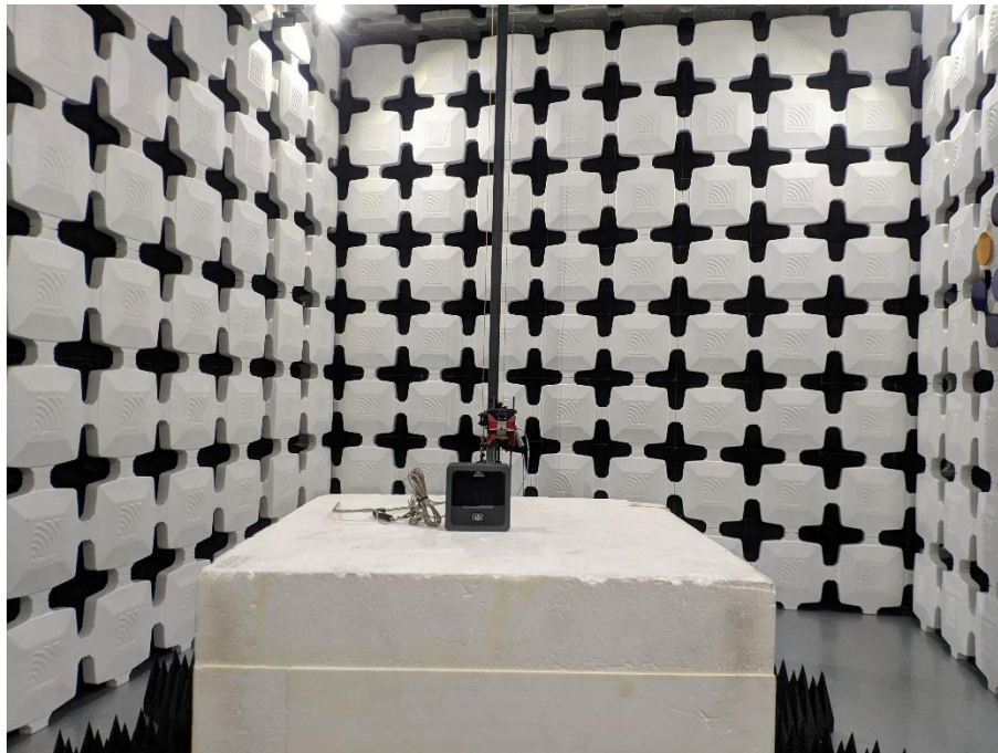
Radiated Emission test Above 1GHz
