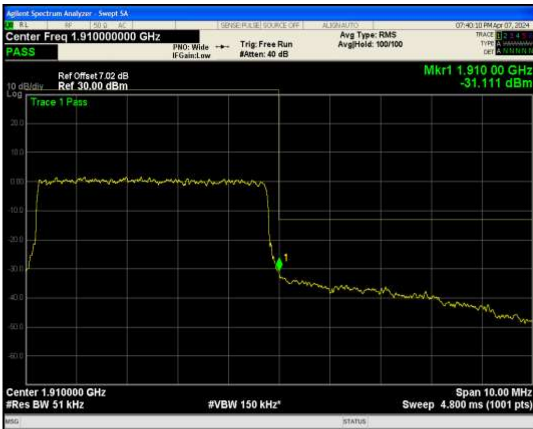
Band2 QPSK BW=10MHz Channel=18650 RB Size=50 Position=#0
