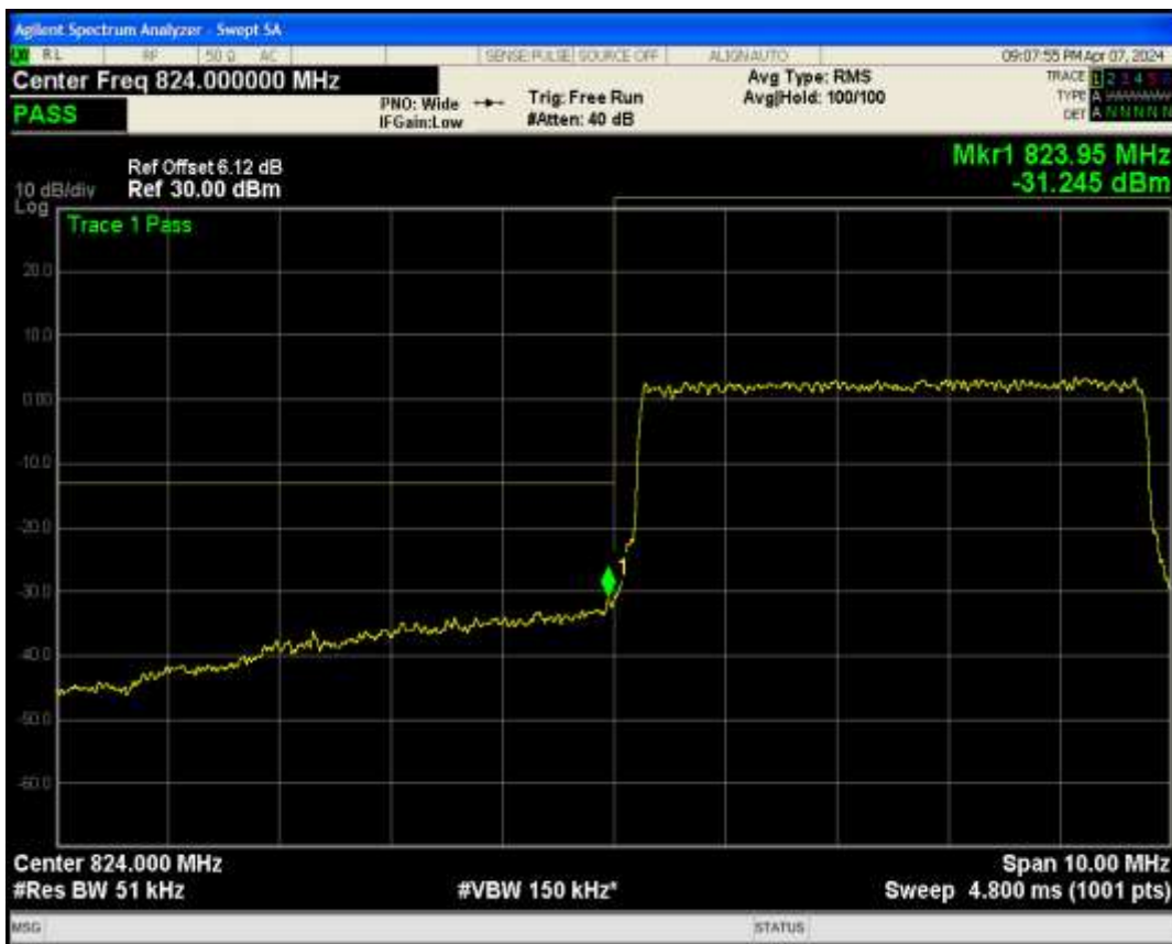
Band5 QPSK BW=5MHz Channel=20625 RB Size=25 Position=#0
