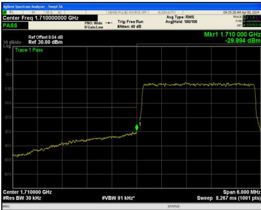
Band4 QPSK BW=3MHz Channel=20385 RB Size=15 Position=#0
