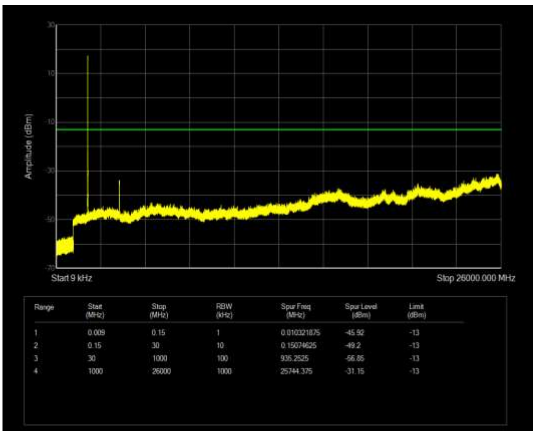
Band2 QAM16 BW=5MHz Channel=18625 RB Size=25 Position=#0
