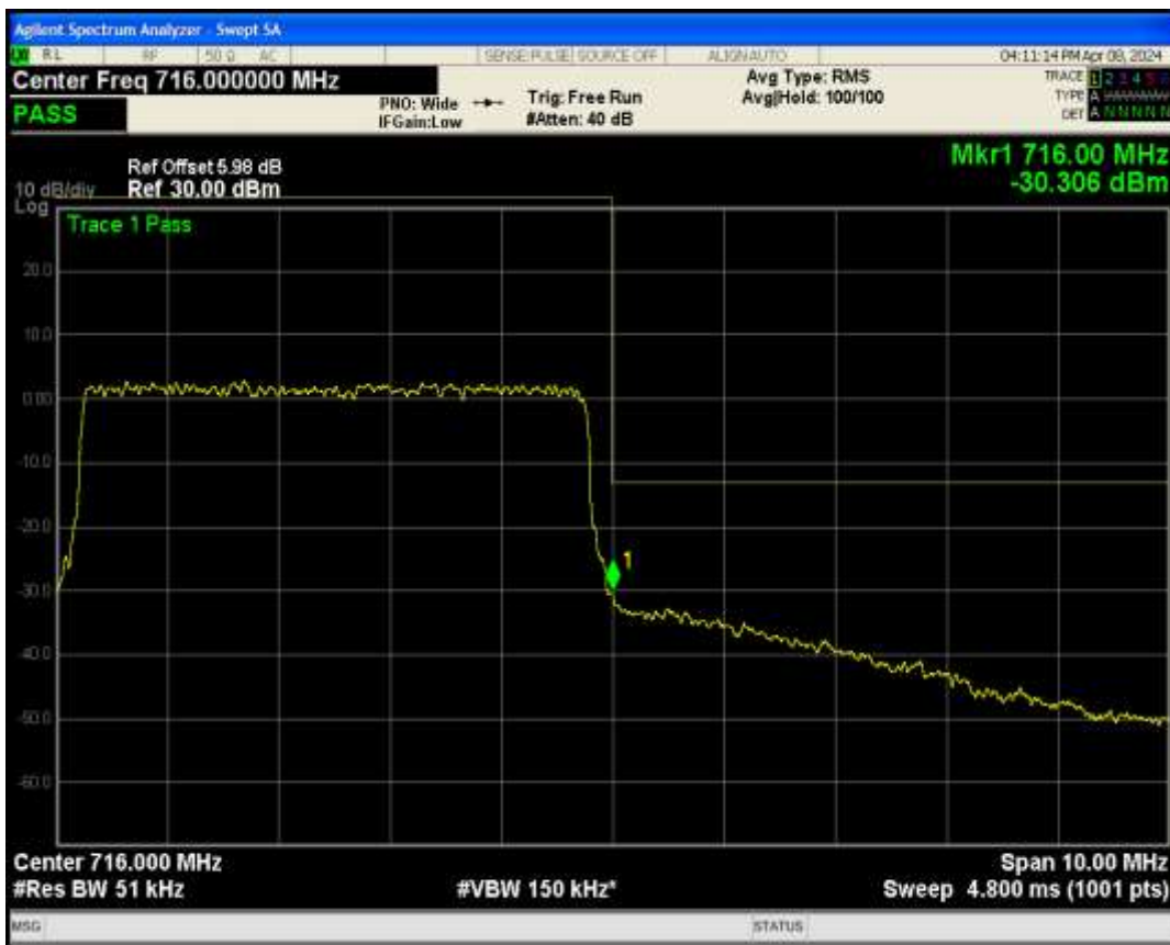
Band17 QPSK BW=10MHz Channel=23800 RB Size=50 Position=#0
