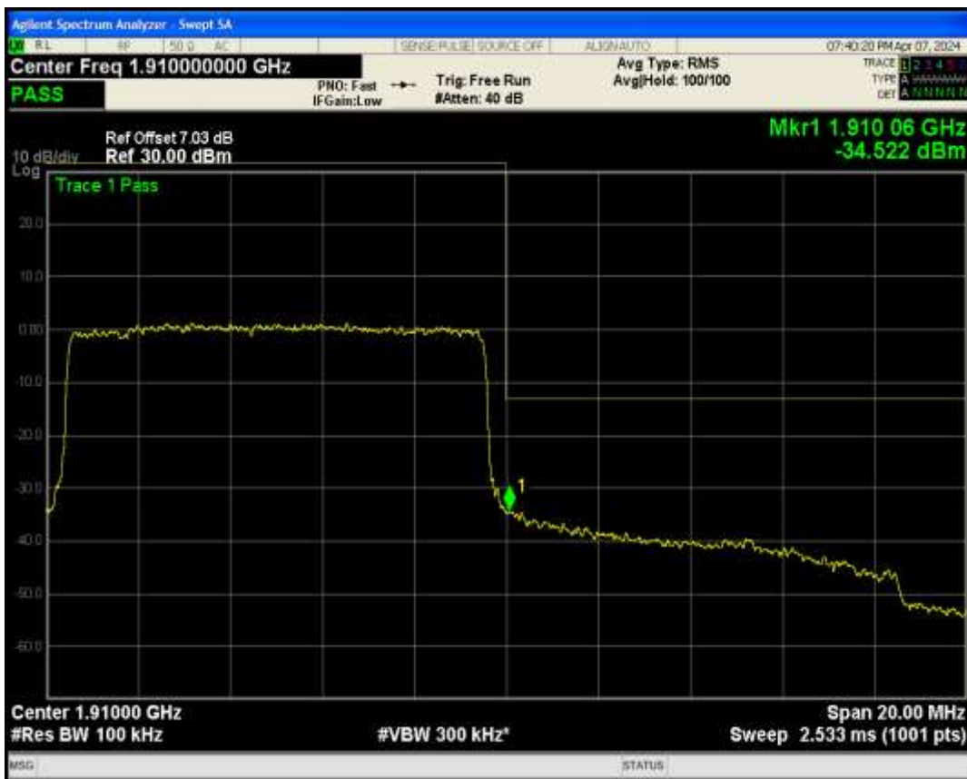
Band2 QPSK BW=15MHz Channel=18675 RB Size=75 Position=#0
