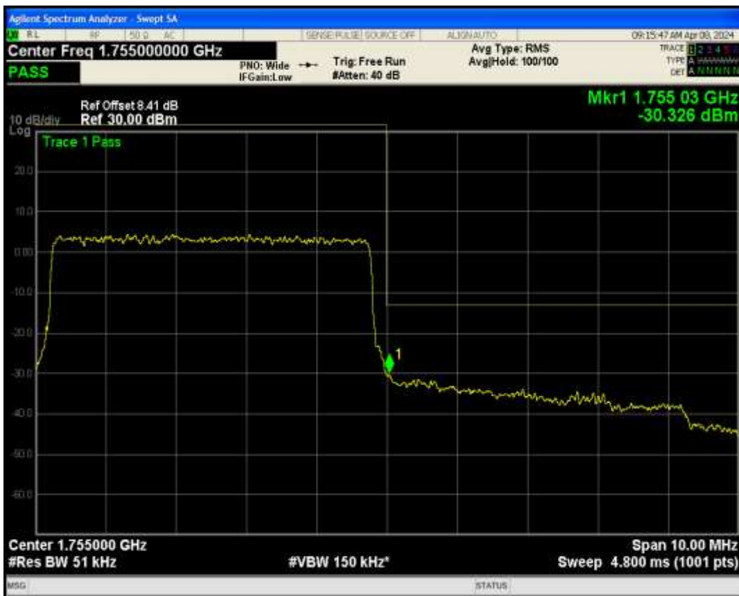
Band4 QAM16 BW=5MHz Channel=20375 RB Size=25 Position=#0
