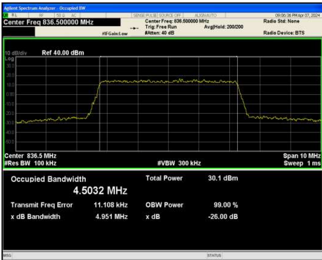
Band5 QPSK BW=10MHz Channel=20525 RB Size=50 Position=#0
