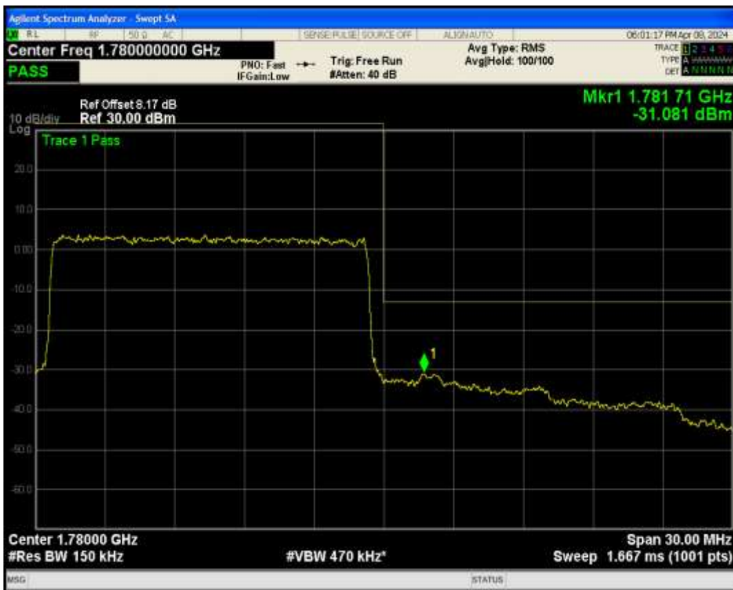
Band66 QPSK BW=20MHz Channel=132072 RB Size=100 Position=#0
