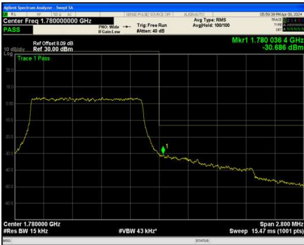
Band66 QAM16 BW=1.4MHz Channel=132665 RB Size=6 Position=#0
