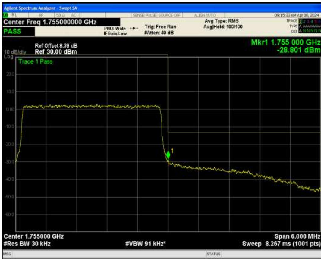
Band4 QPSK BW=5MHz Channel=19975 RB Size=25 Position=#0
