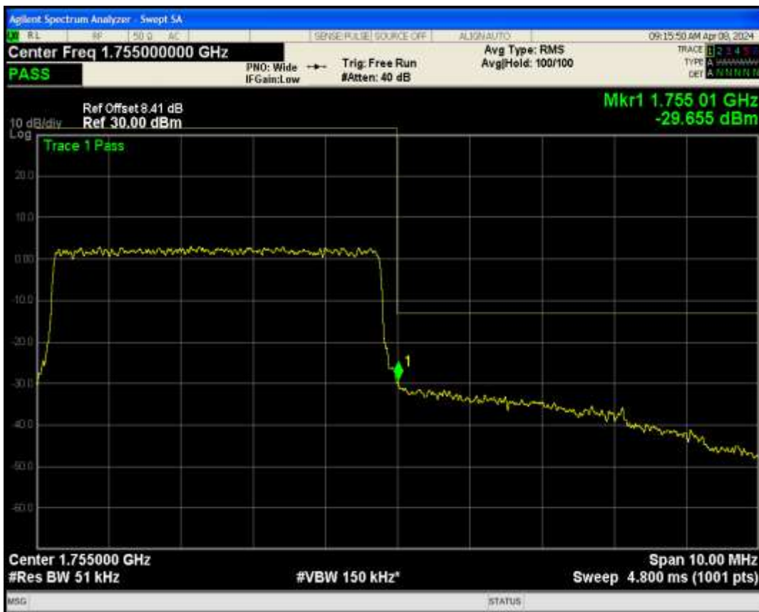
Band4 QPSK BW=10MHz Channel=20000 RB Size=50 Position=#0
