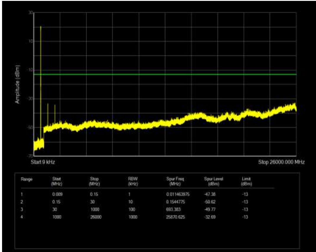
Band12 QAM16 BW=1.4MHz Channel=23017 RB Size=6 Position=#0
