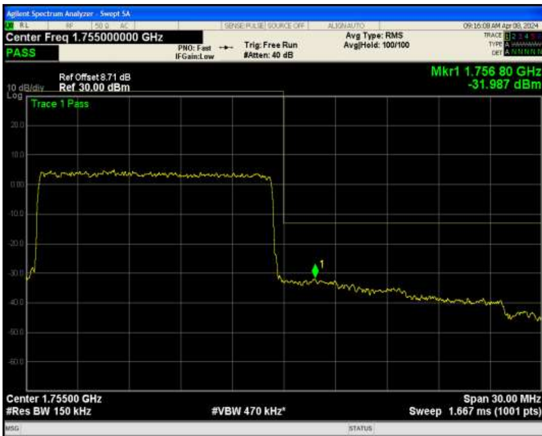
Band4 QPSK BW=20MHz Channel=20050 RB Size=100 Position=#0
