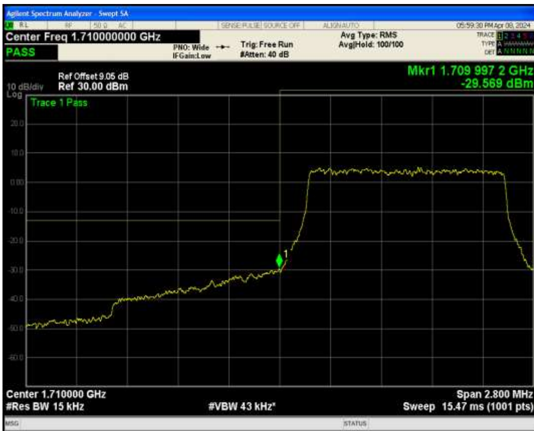
Band66 QAM16 BW=1.4MHz Channel=131979 RB Size=6 Position=#0
