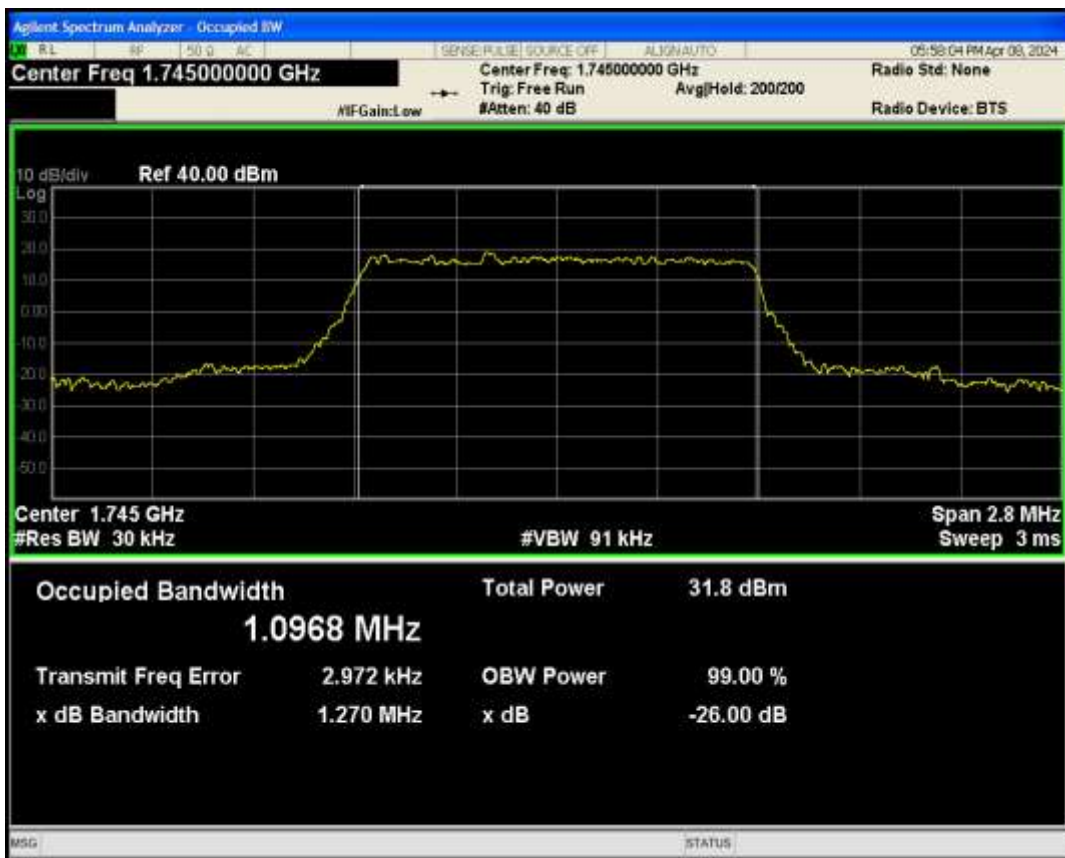
Band66 QPSK BW=3MHz Channel=132322 RB Size=15 Position=#0
