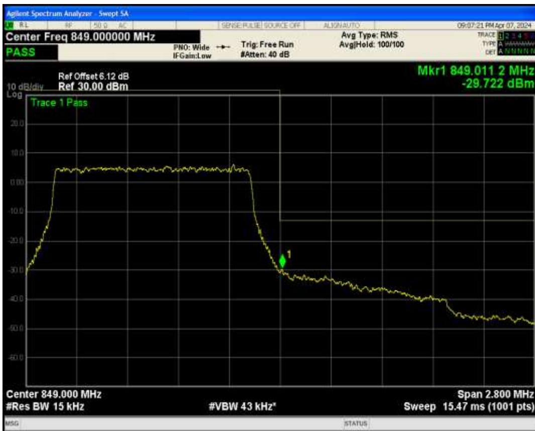
Band5 QAM16 BW=1.4MHz Channel=20643 RB Size=6 Position=#0
