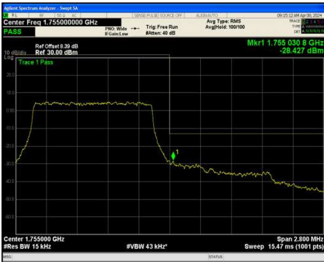
Band4 QAM16 BW=1.4MHz Channel=20393 RB Size=6 Position=#0
