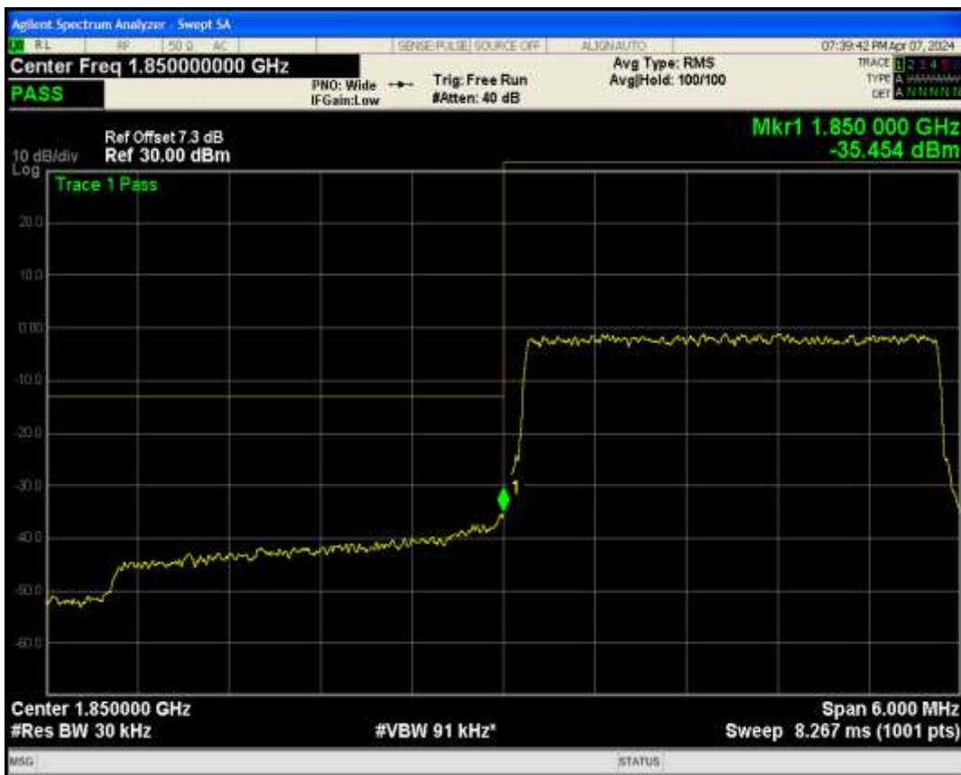
Band2 QAM16 BW=3MHz Channel=18615 RB Size=15 Position=#0
