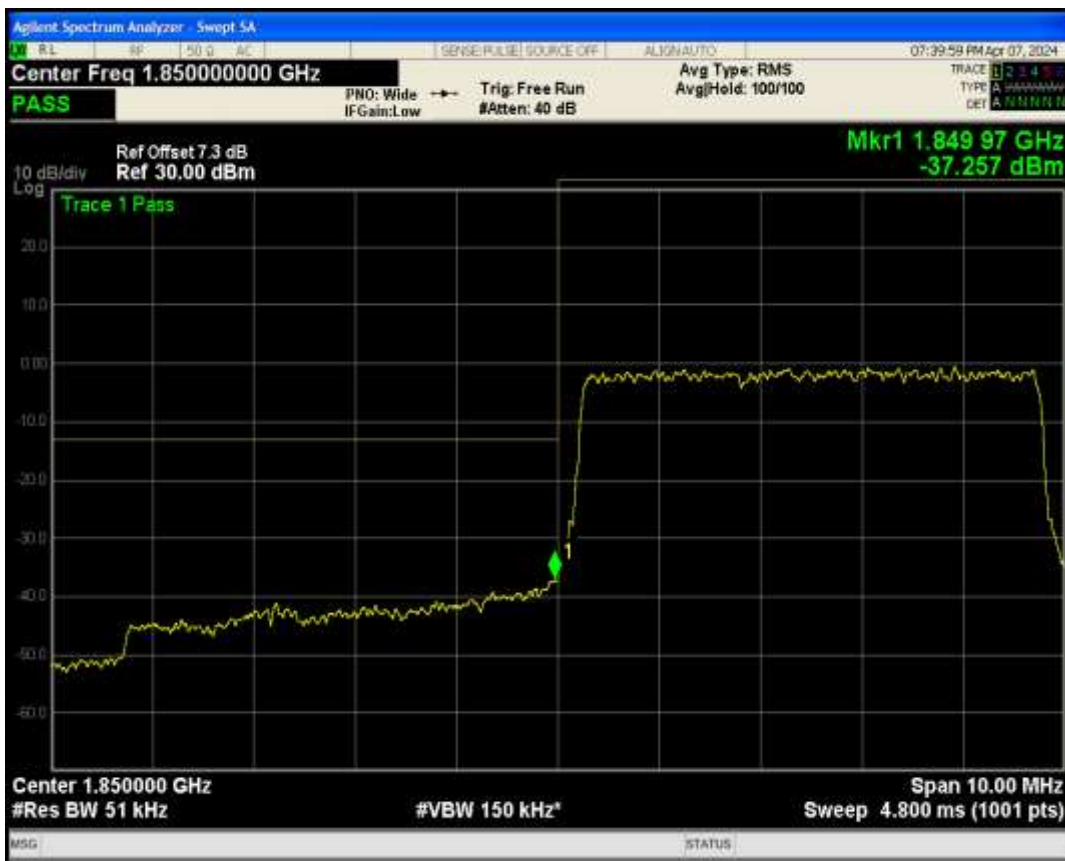
Band2 QAM16 BW=5MHz Channel=18625 RB Size=25 Position=#0
