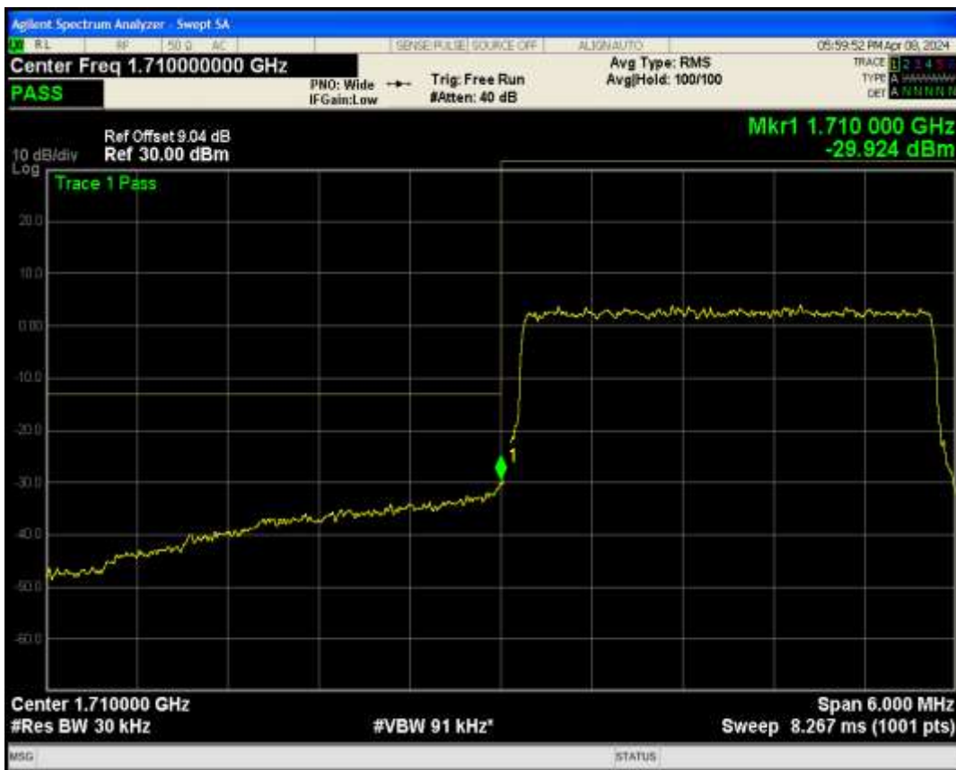
Band66 QPSK BW=3MHz Channel=132657 RB Size=15 Position=#0
