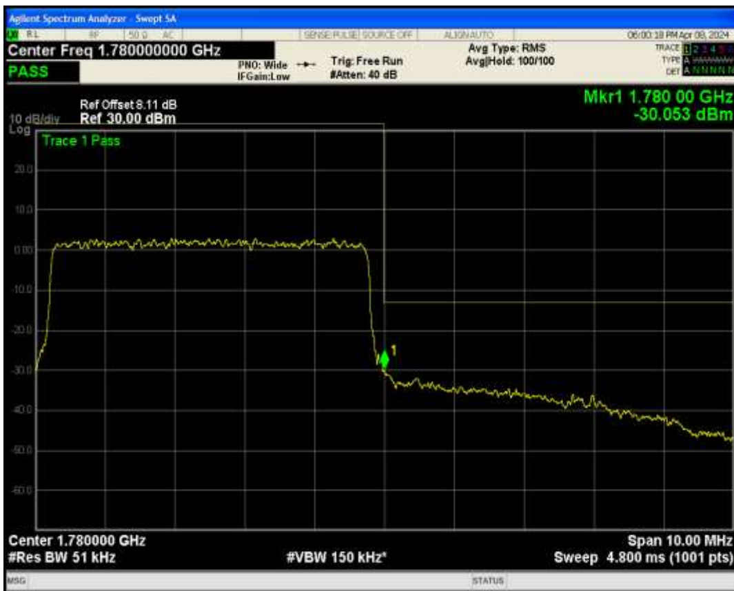
Band66 QPSK BW=10MHz Channel=132022 RB Size=50 Position=#0
