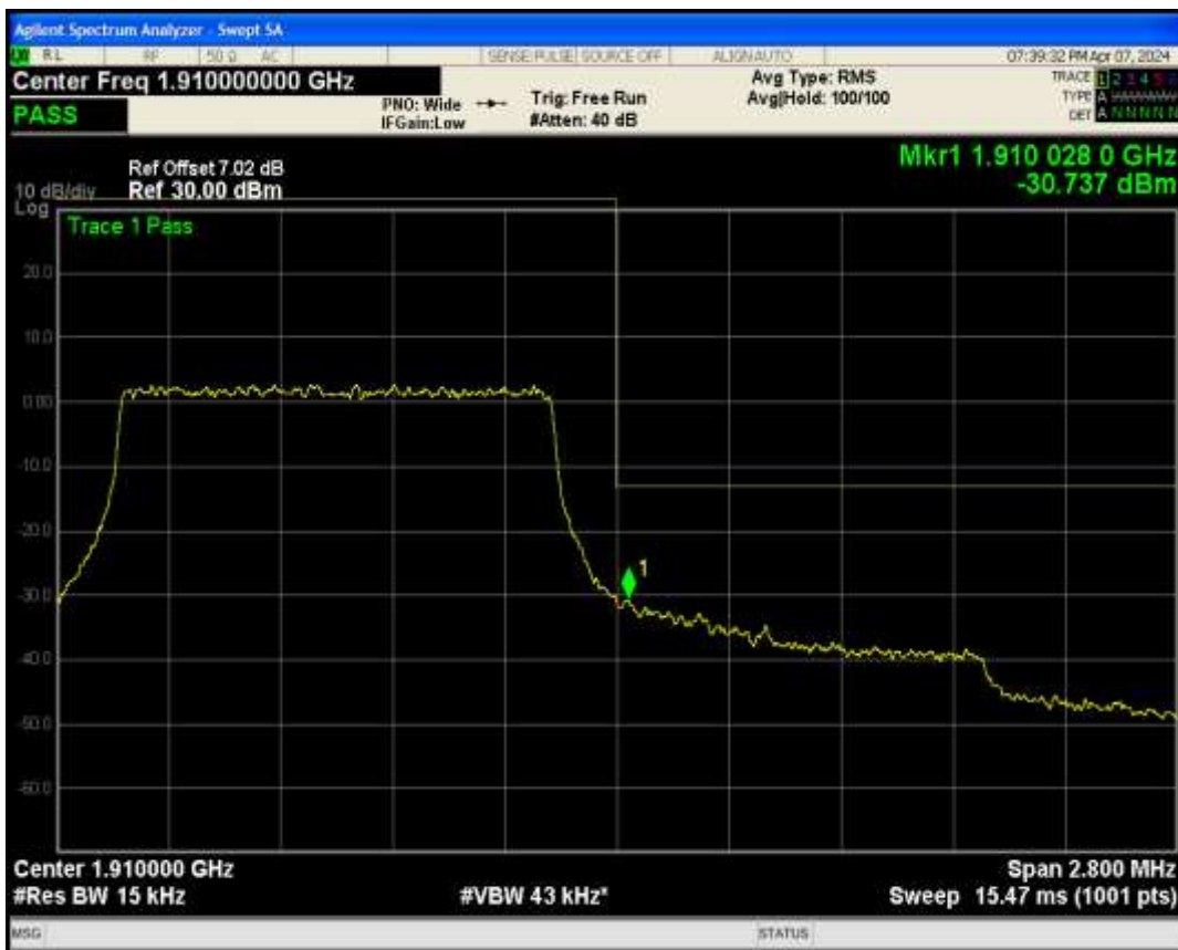
Band2 QAM16 BW=1.4MHz Channel=19193 RB Size=6 Position=#0
