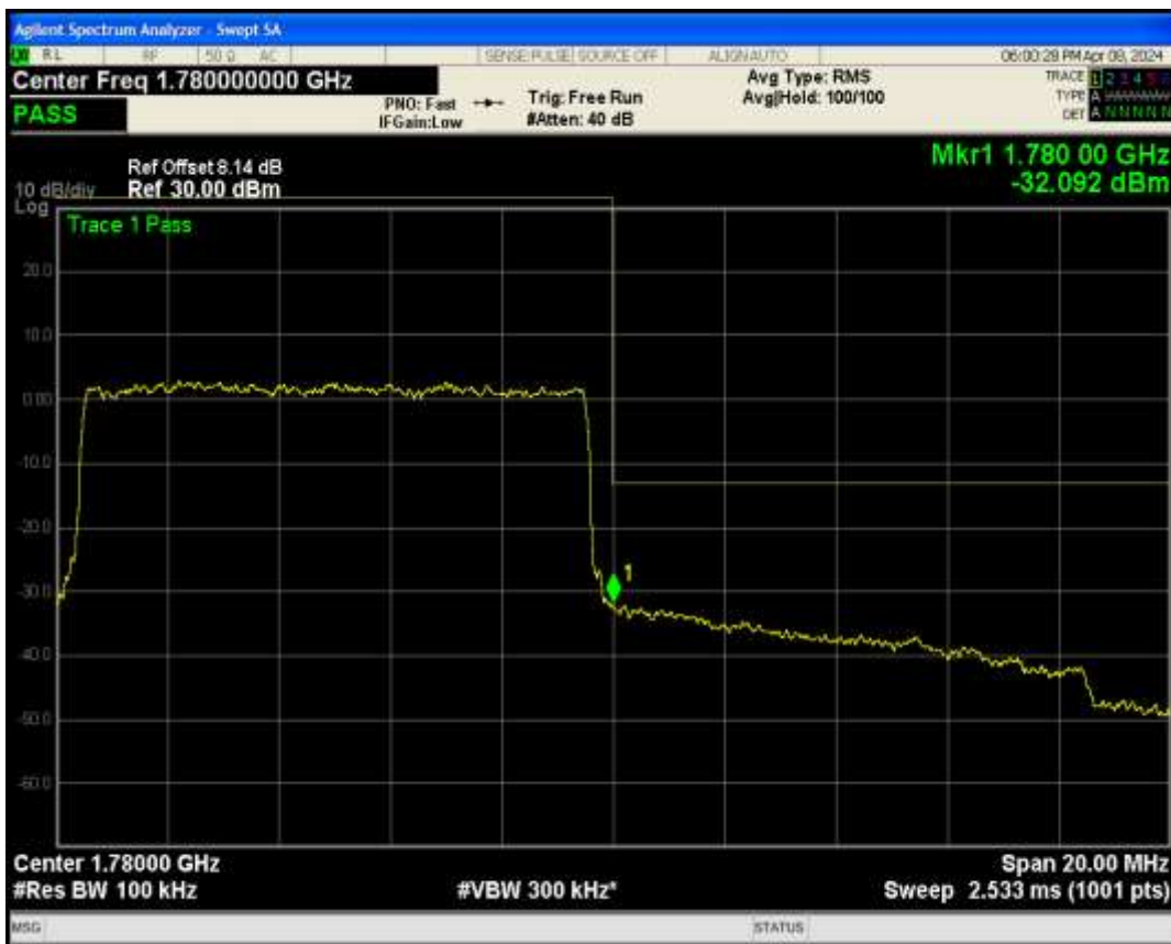
Band66 QPSK BW=15MHz Channel=132047 RB Size=75 Position=#0
