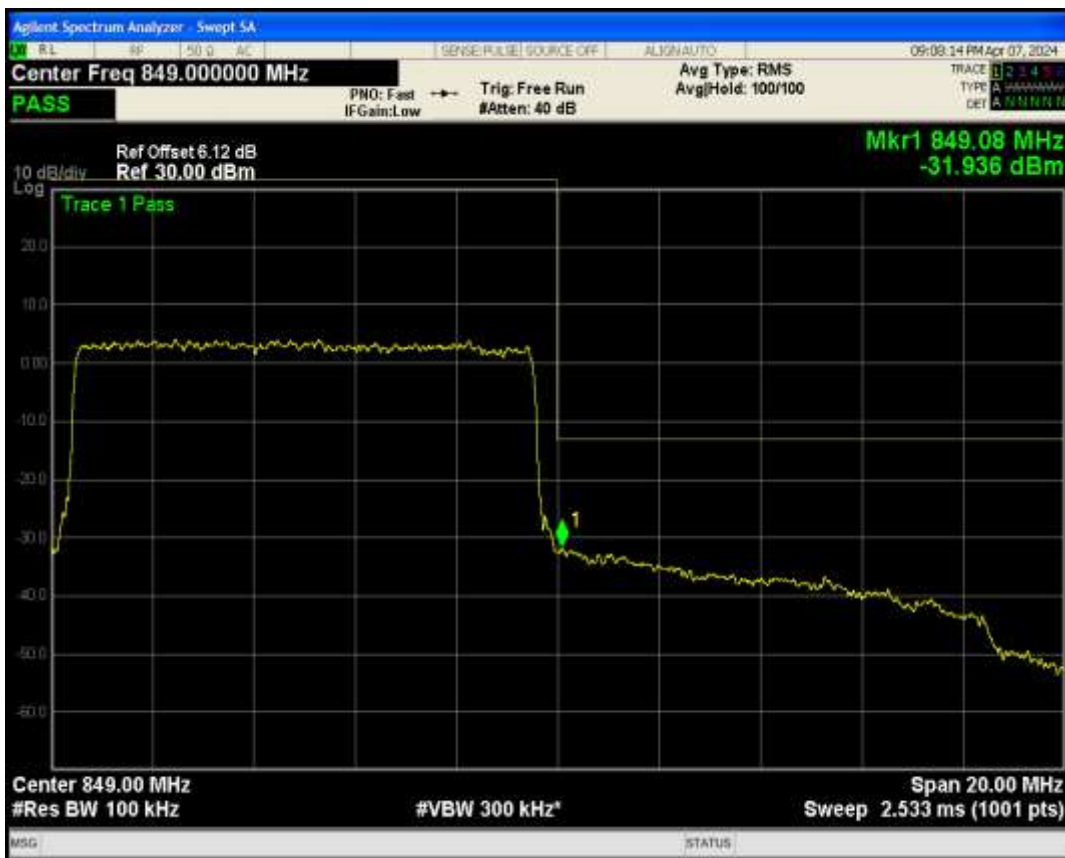
Band66 QPSK BW=1.4MHz Channel=131979 RB Size=6 Position=#0
