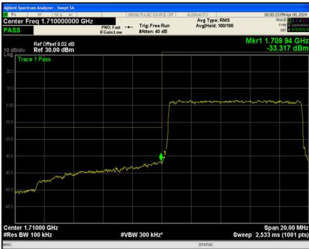
Band66 QPSK BW=10MHz Channel=132622 RB Size=50 Position=#0
