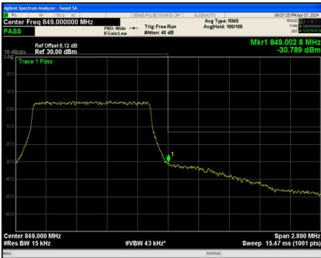
Band5 QPSK BW=3MHz Channel=20415 RB Size=15 Position=#0
