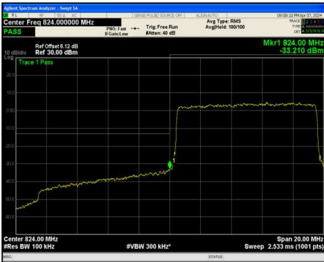
Band5 QPSK BW=10MHz Channel=20600 RB Size=50 Position=#0
