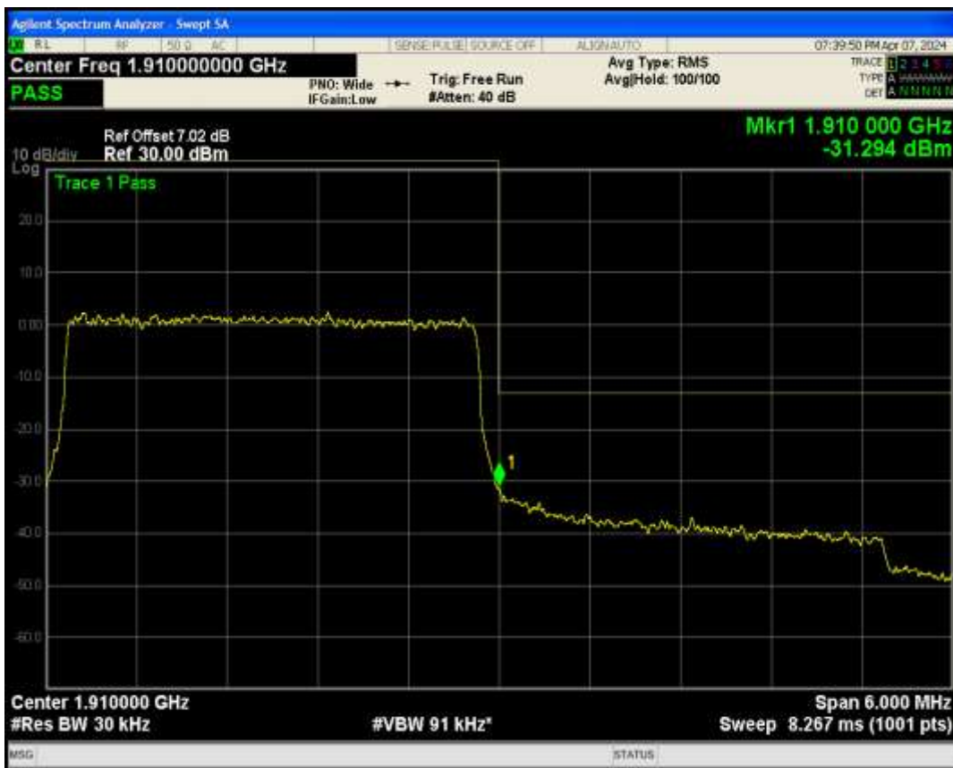
Band2 QAM16 BW=3MHz Channel=19185 RB Size=15 Position=#0
