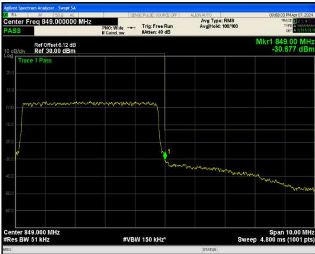
Band5 QPSK BW=10MHz Channel=20450 RB Size=50 Position=#0
