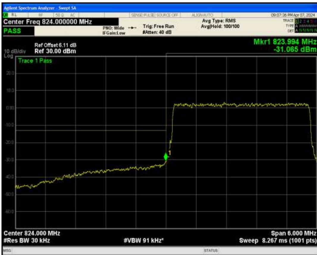
Band5 QPSK BW=3MHz Channel=20635 RB Size=15 Position=#0
