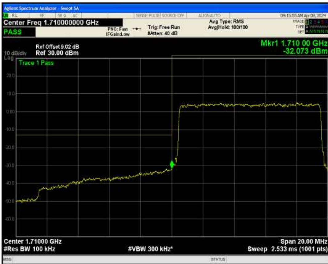
Band4 QPSK BW=10MHz Channel=20350 RB Size=50 Position=#0
