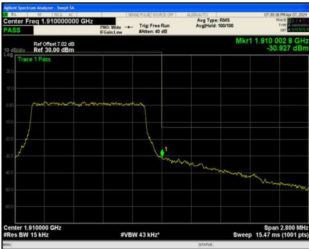
Band2 QPSK BW=3MHz Channel=18615 RB Size=15 Position=#0
