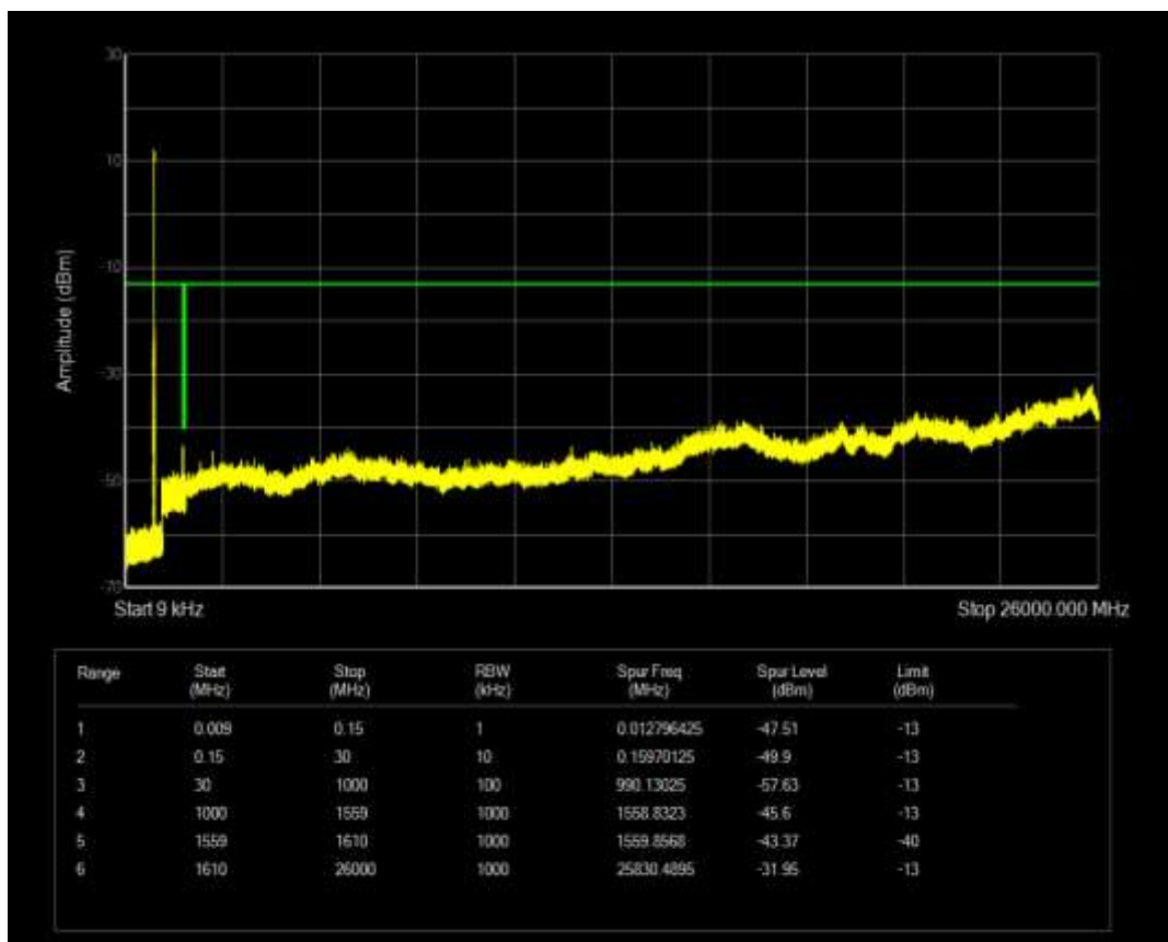
Band13 QPSK BW=5MHz Channel=23255 RB Size=25 Position=#0
