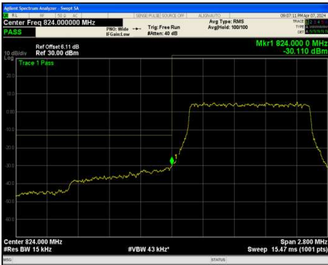
Band5 QAM16 BW=1.4MHz Channel=20407 RB Size=6 Position=#0
