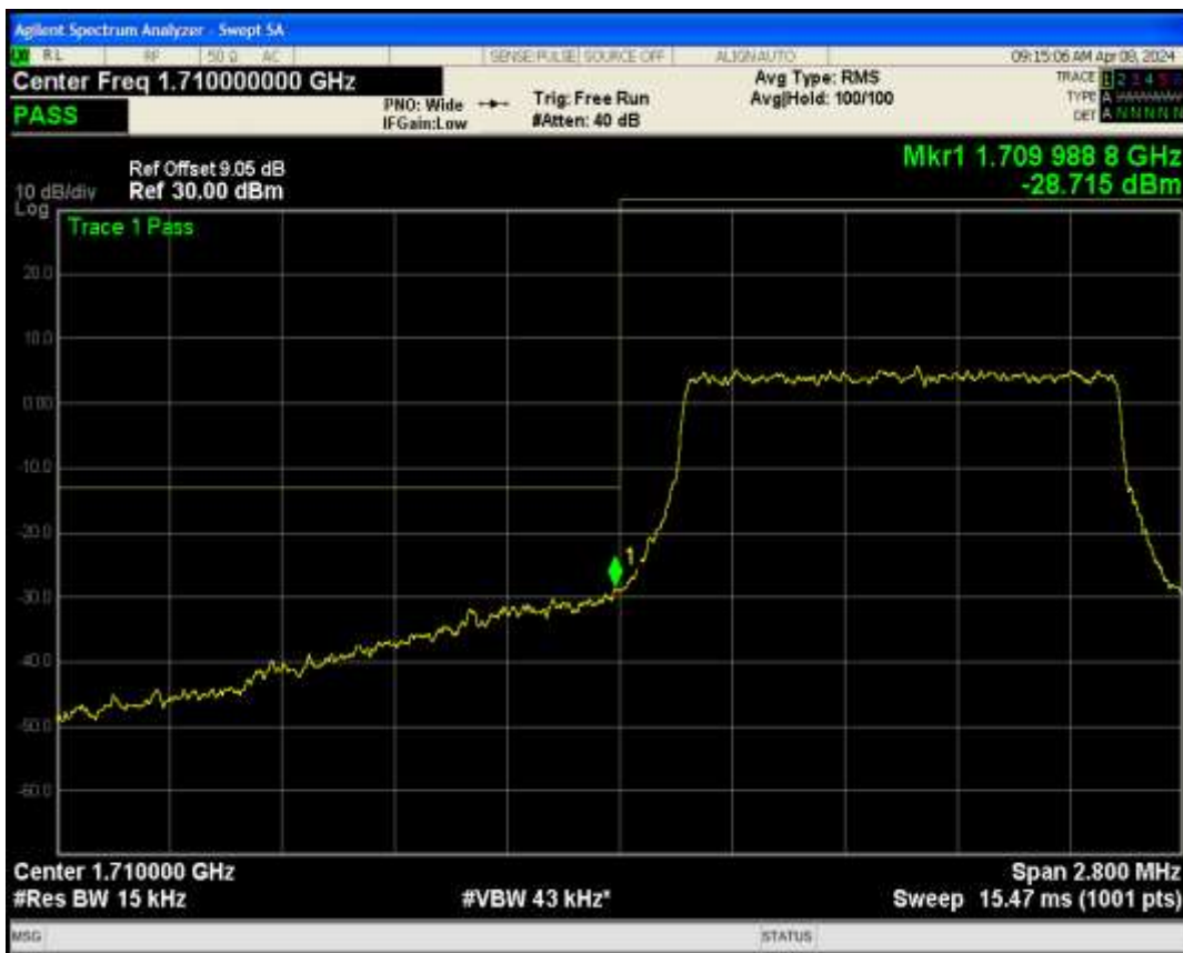
Band4 QPSK BW=1.4MHz Channel=20393 RB Size=6 Position=#0
