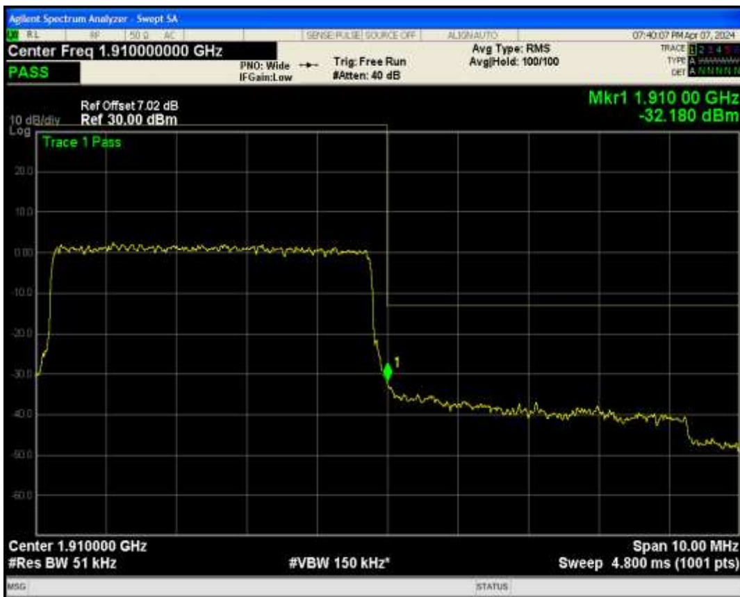
Band2 QAM16 BW=5MHz Channel=19175 RB Size=25 Position=#0
