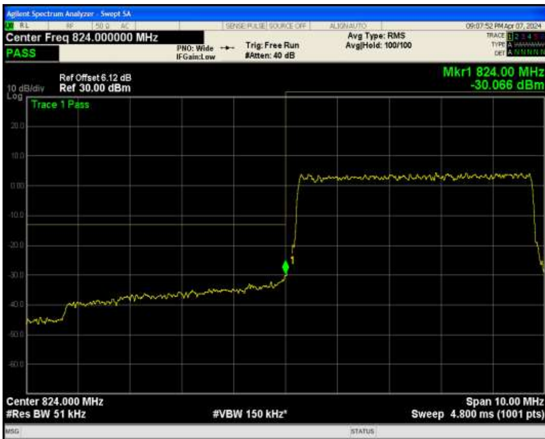
Band5 QAM16 BW=5MHz Channel=20425 RB Size=25 Position=#0
