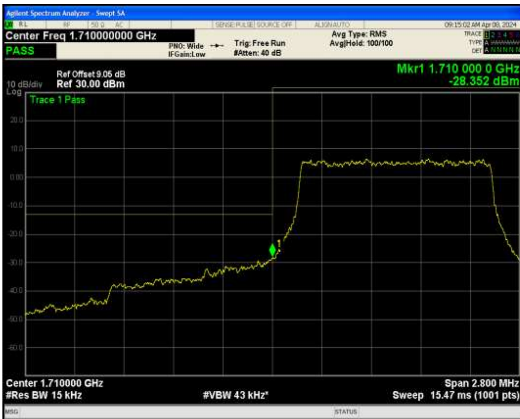
Band4 QAM16 BW=1.4MHz Channel=19957 RB Size=6 Position=#0
