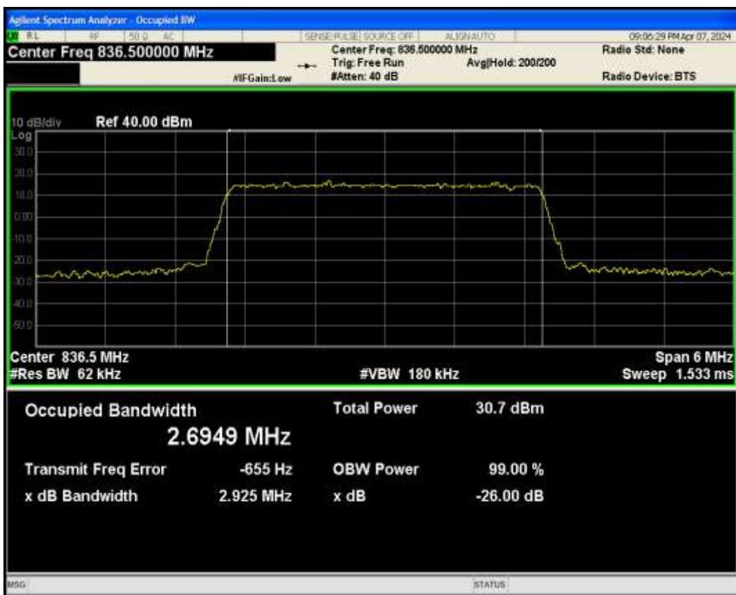
Band5 QPSK BW=5MHz Channel=20525 RB Size=25 Position=#0
