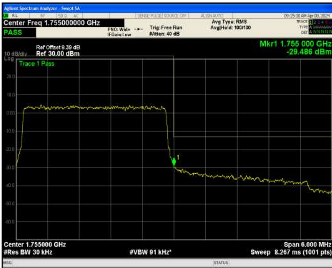
Band4 QAM16 BW=3MHz Channel=20385 RB Size=15 Position=#0
