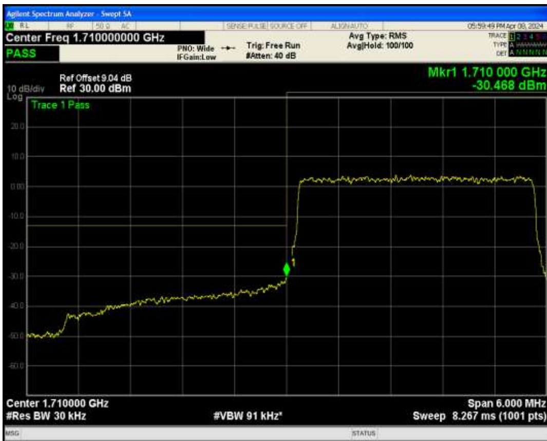
Band66 QAM16 BW=3MHz Channel=131987 RB Size=15 Position=#0
