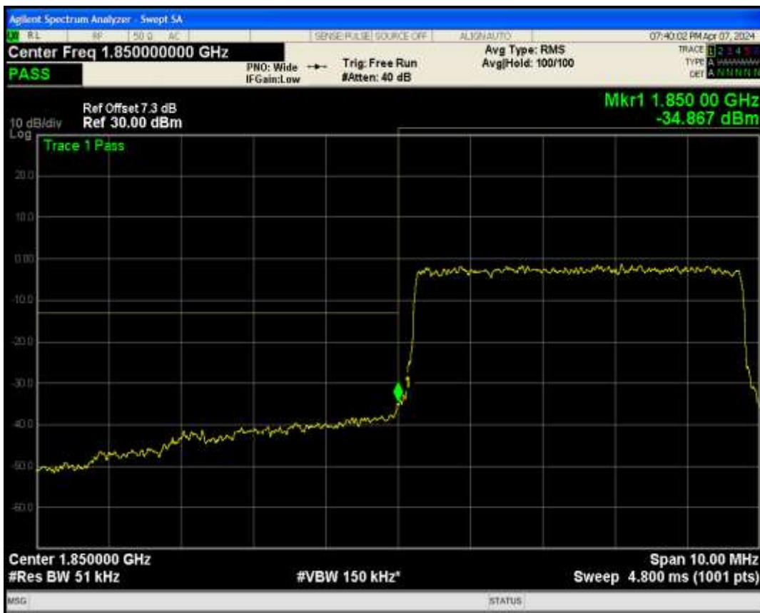
Band2 QPSK BW=5MHz Channel=19175 RB Size=25 Position=#0
