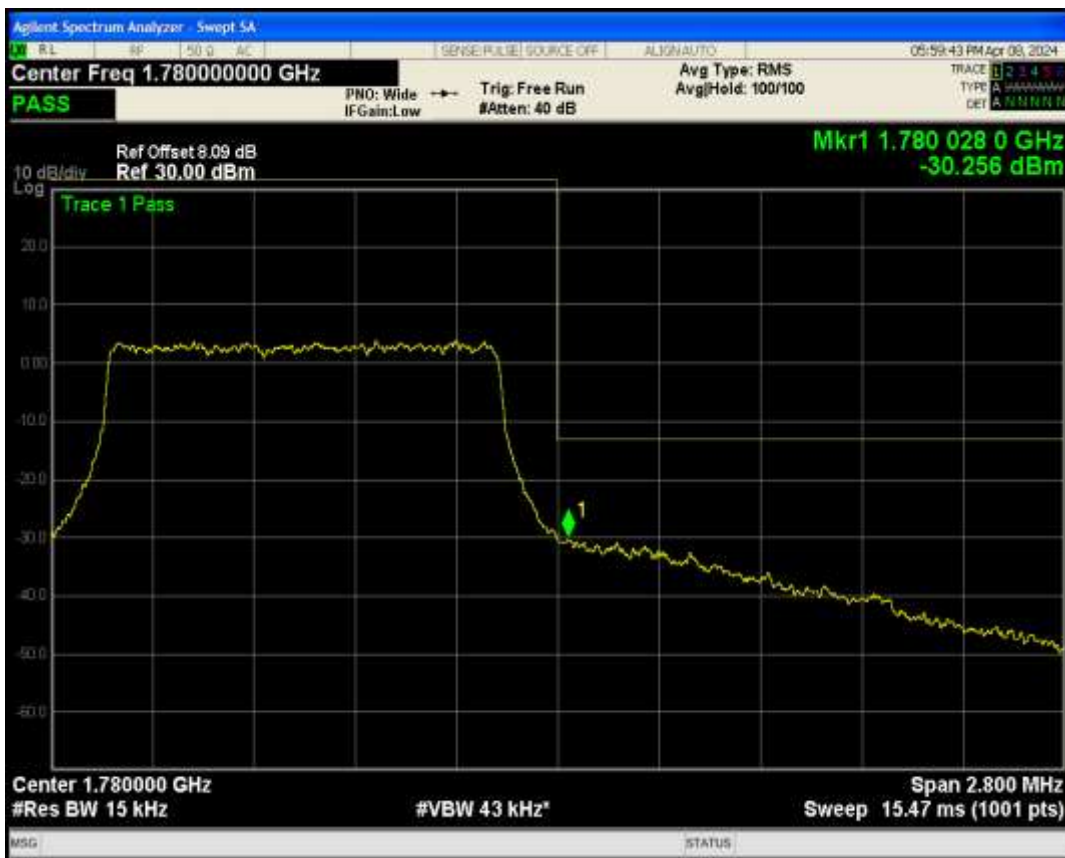
Band66 QPSK BW=3MHz Channel=131987 RB Size=15 Position=#0
