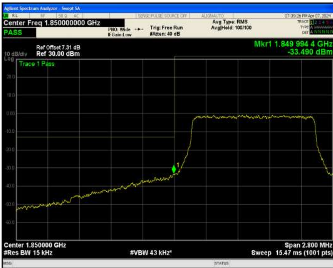
Band2 QPSK BW=1.4MHz Channel=19193 RB Size=6 Position=#0
