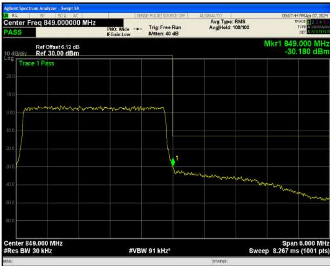
Band5 QPSK BW=5MHz Channel=20425 RB Size=25 Position=#0
