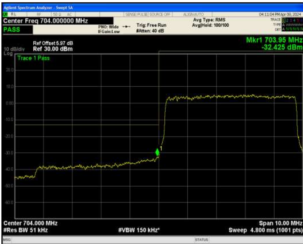
Band17 QAM16 BW=5MHz Channel=23755 RB Size=25 Position=#0
