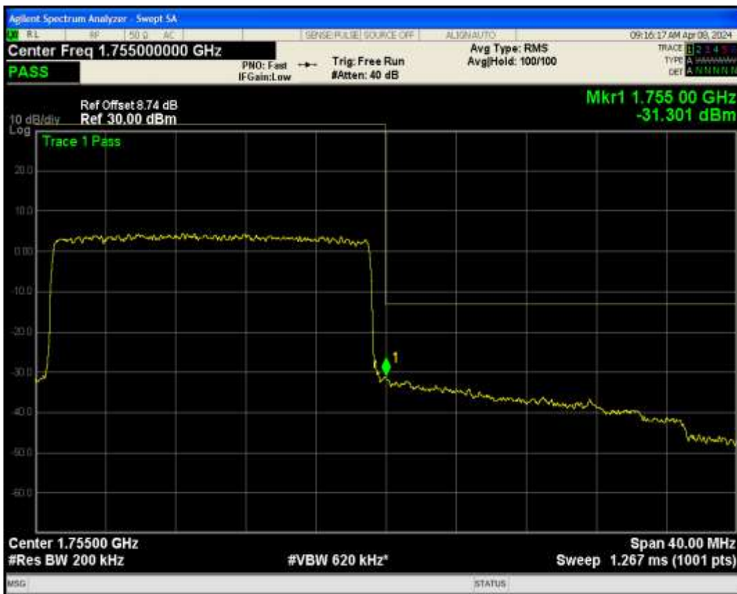
Band40a QPSK BW=5MHz Channel=38725 RB Size=25 Position=#0
