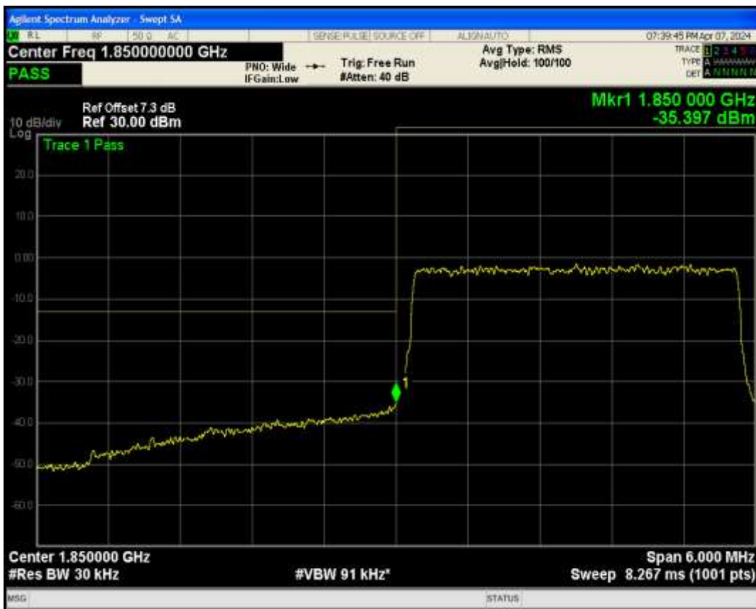
Band2 QPSK BW=3MHz Channel=19185 RB Size=15 Position=#0
