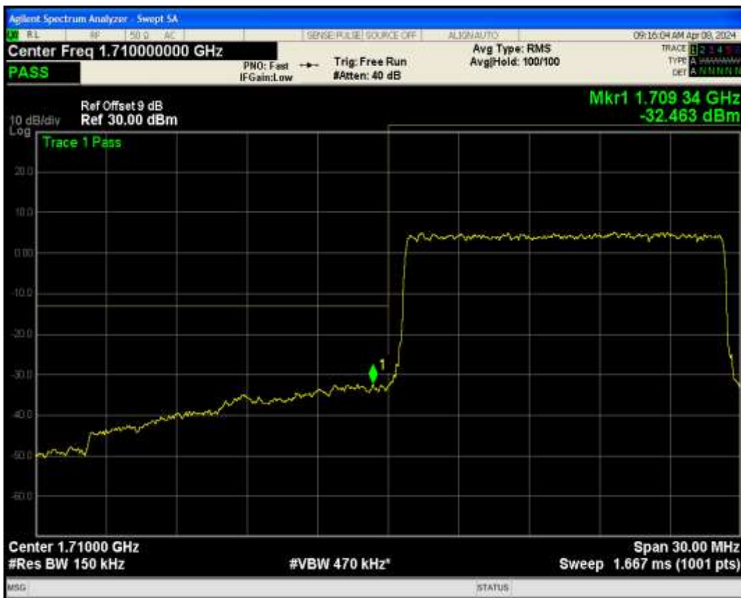
Band4 QPSK BW=15MHz Channel=20325 RB Size=75 Position=#0
