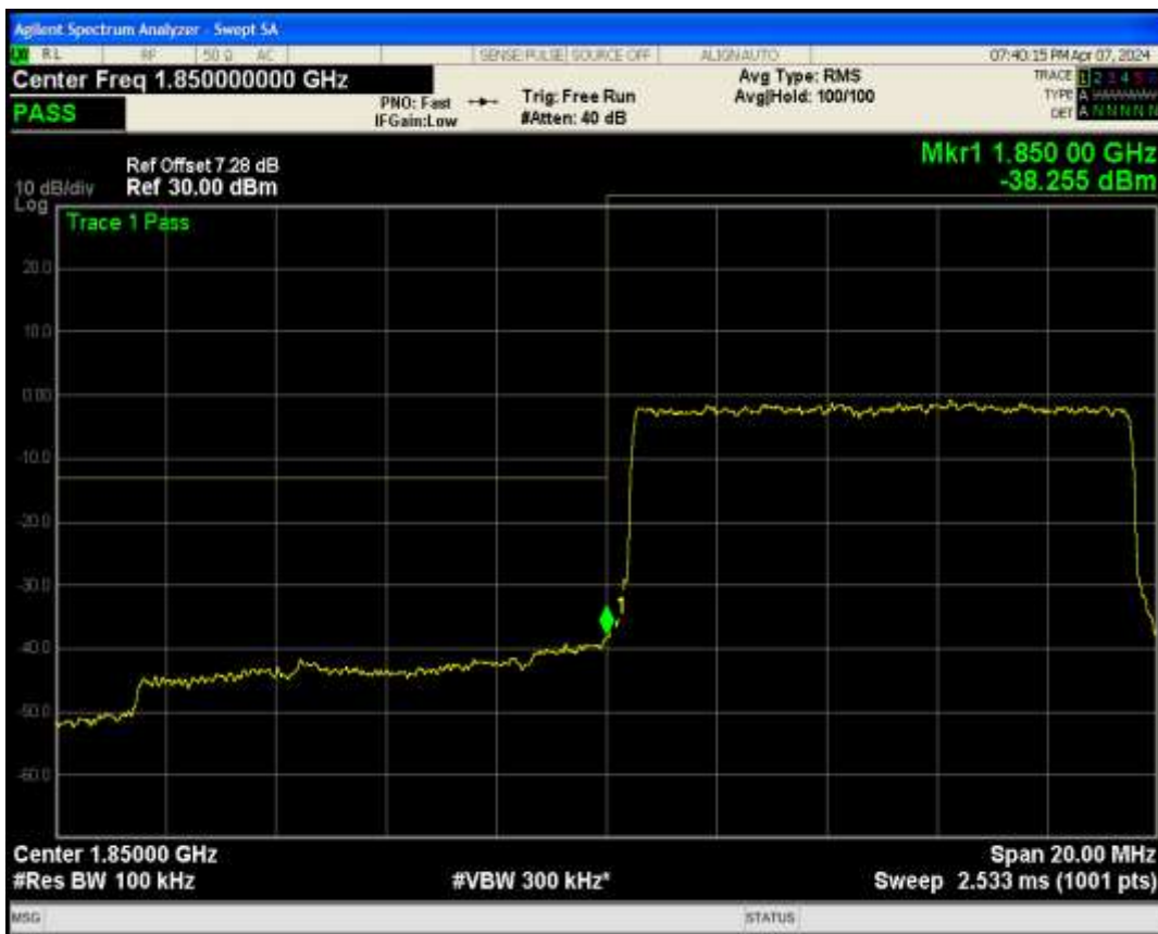
Band2 QPSK BW=10MHz Channel=19150 RB Size=50 Position=#0
