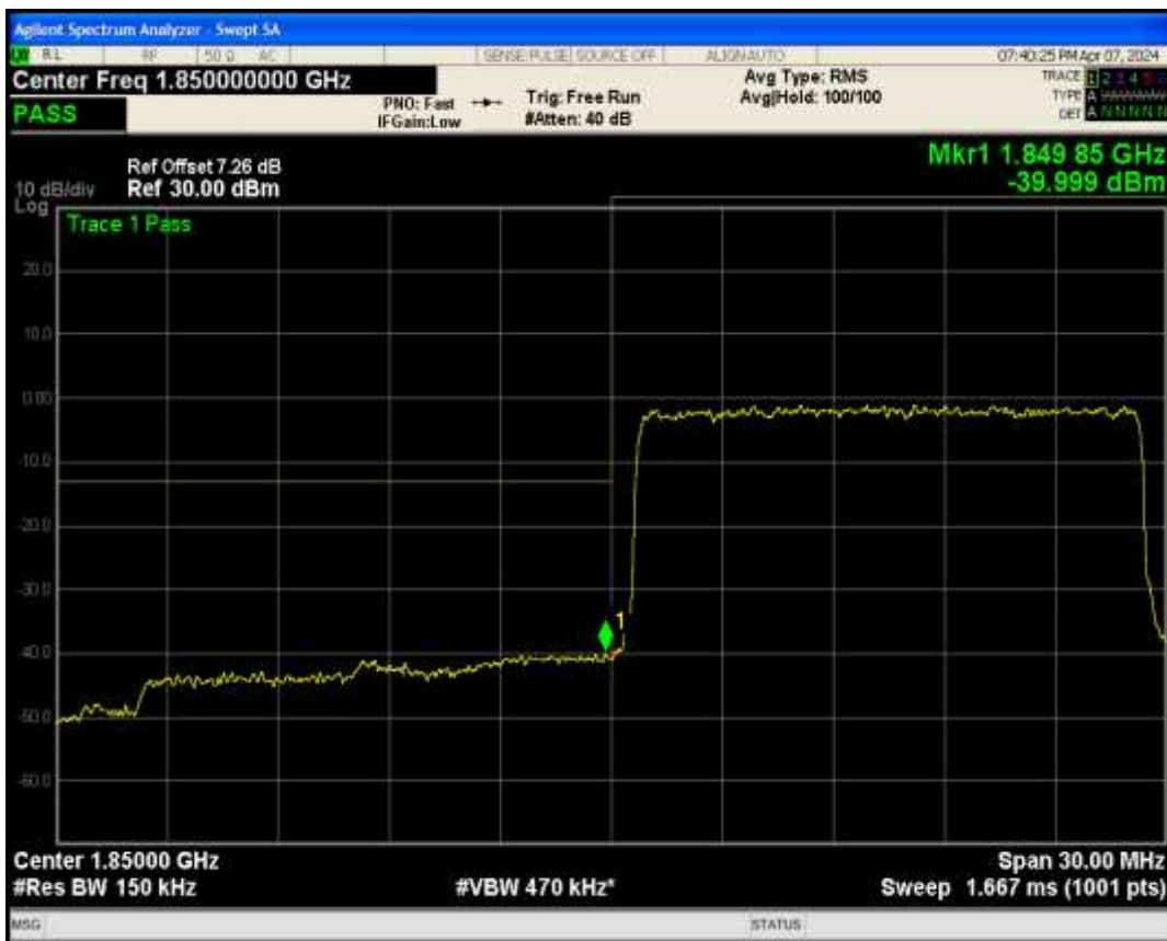
Band2 QPSK BW=15MHz Channel=19125 RB Size=75 Position=#0
