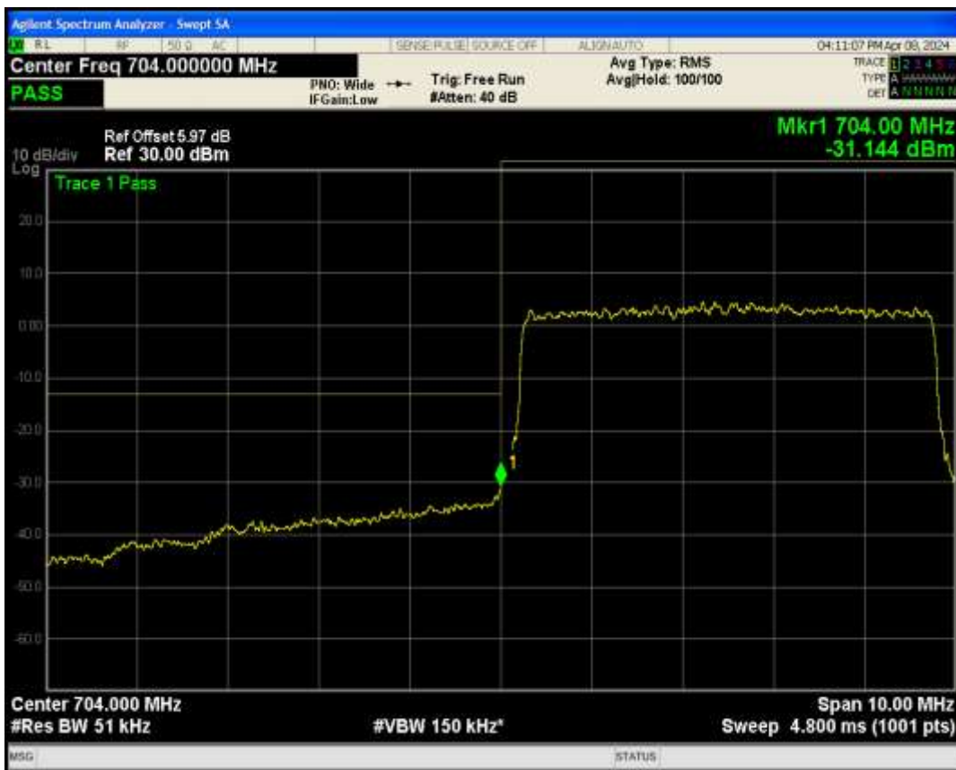
Band17 QPSK BW=5MHz Channel=23825 RB Size=25 Position=#0
