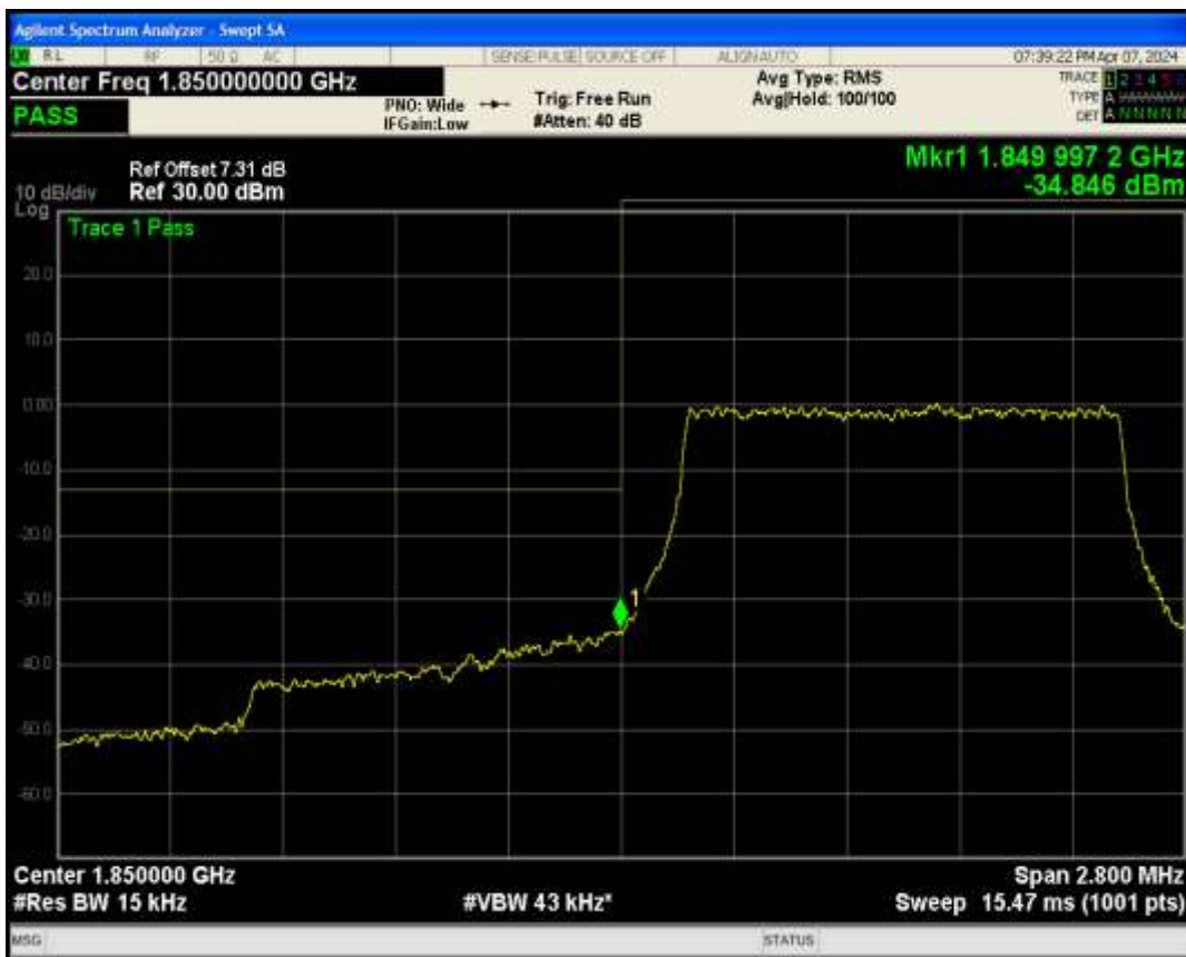
Band2 QAM16 BW=1.4MHz Channel=18607 RB Size=6 Position=#0
