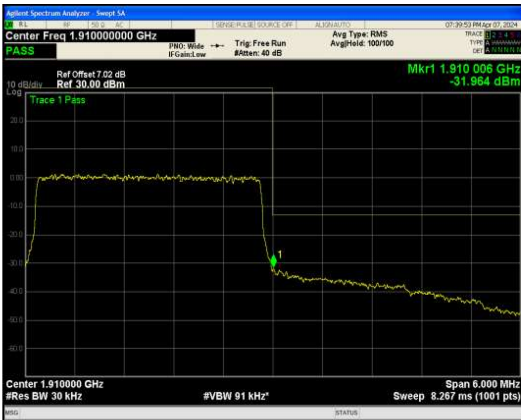
Band2 QPSK BW=5MHz Channel=18625 RB Size=25 Position=#0
