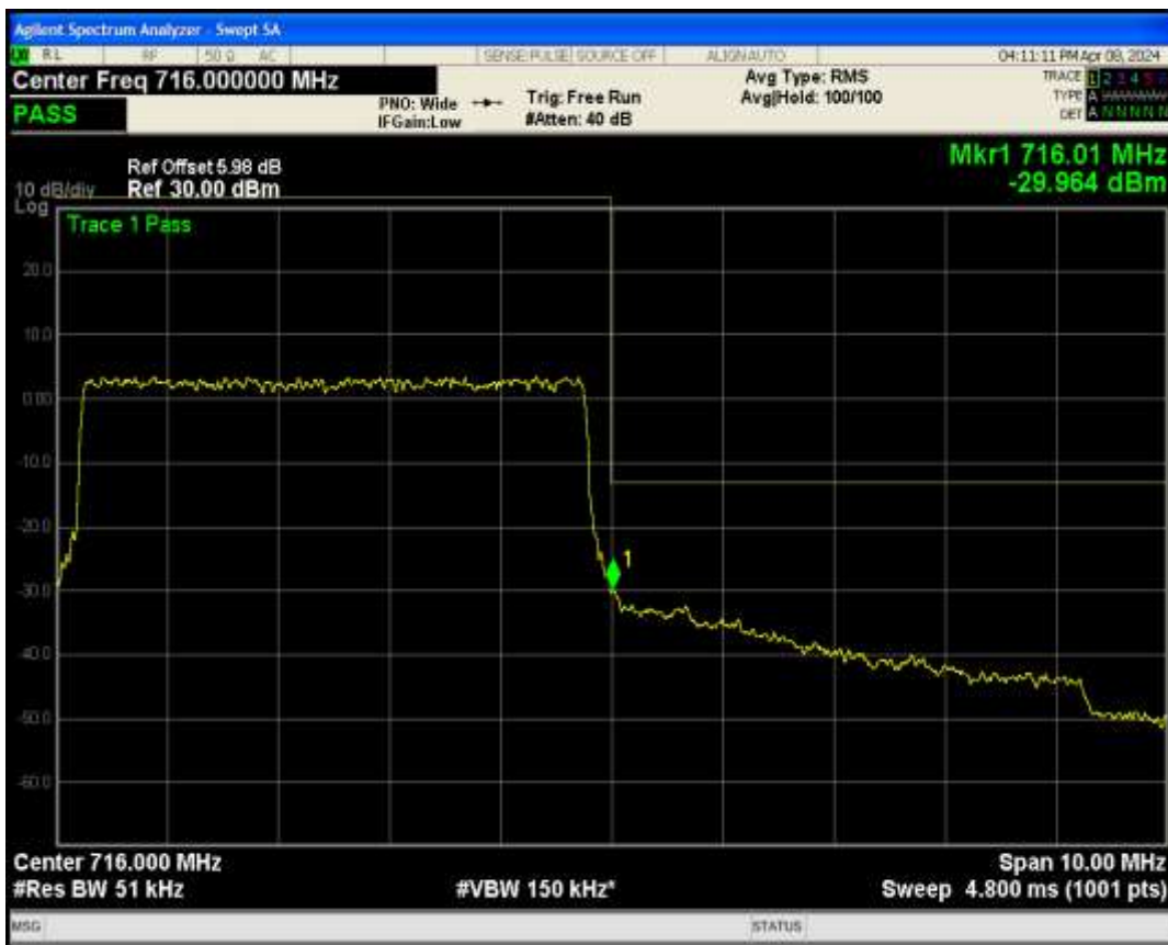
Band17 QPSK BW=10MHz Channel=23780 RB Size=50 Position=#0
