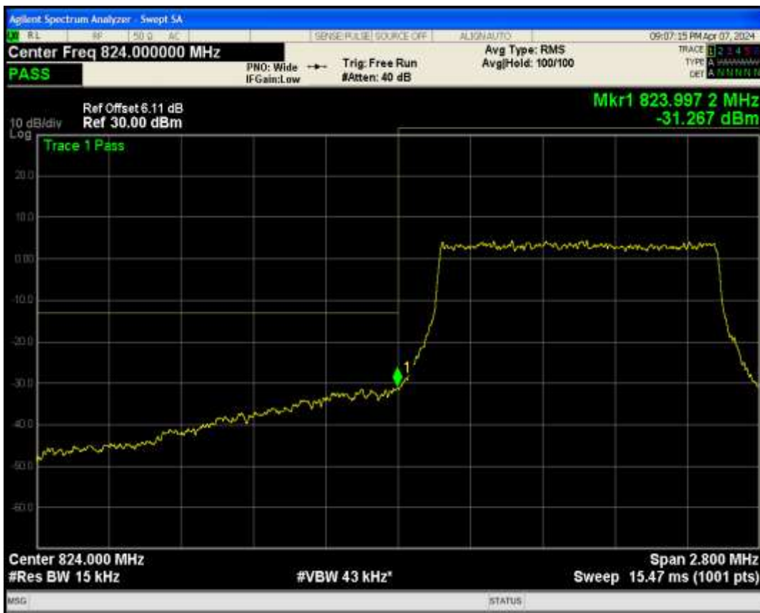
Band5 QPSK BW=1.4MHz Channel=20643 RB Size=6 Position=#0
