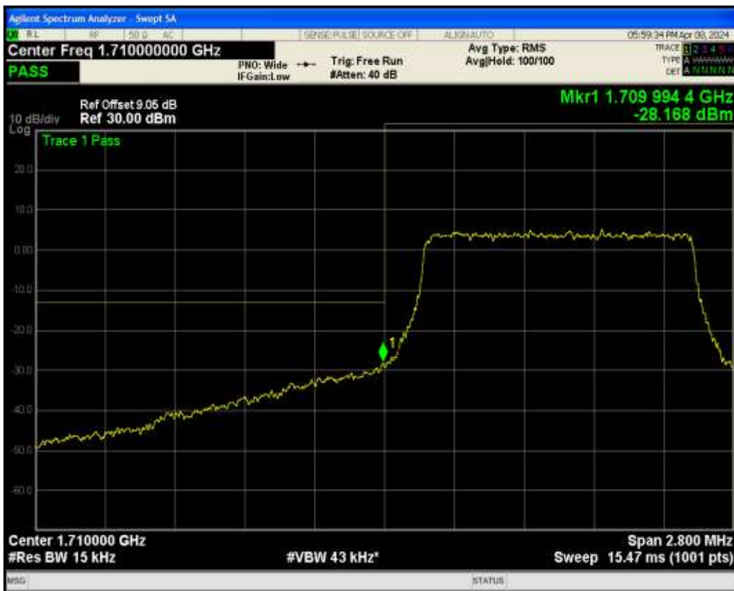
Band66 QPSK BW=1.4MHz Channel=132665 RB Size=6 Position=#0
