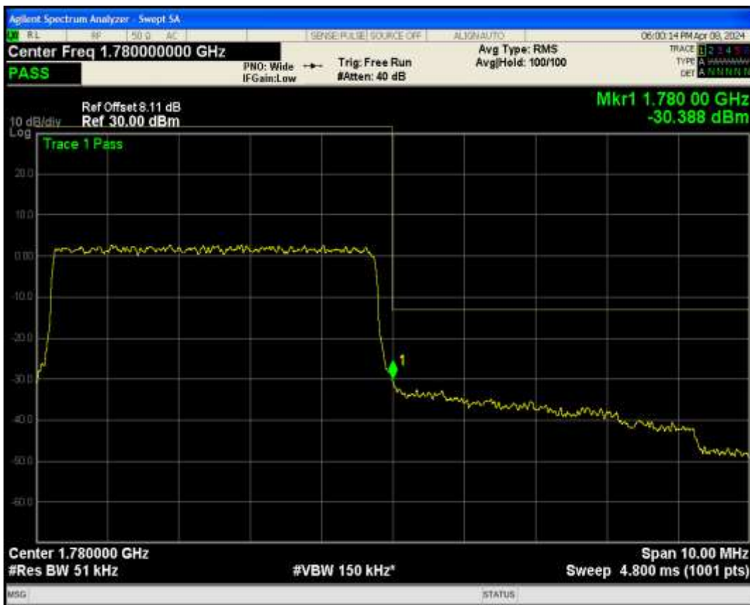
Band66 QAM16 BW=5MHz Channel=132647 RB Size=25 Position=#0
