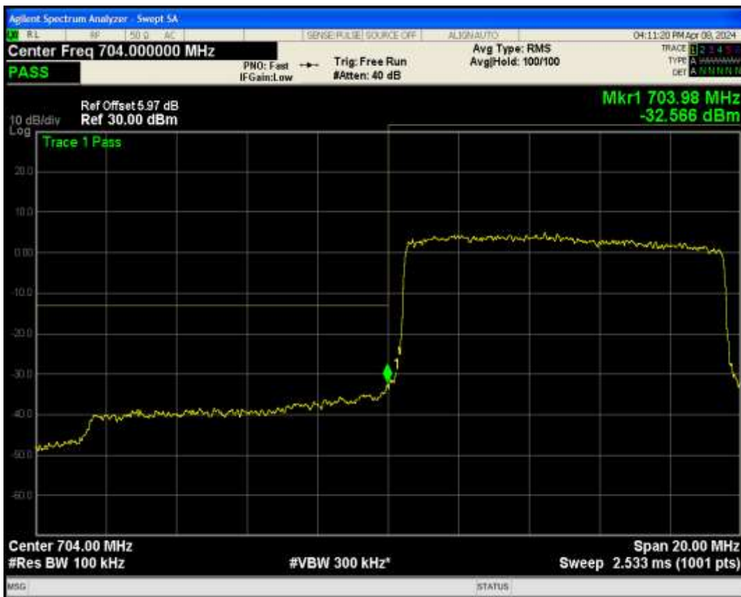
Band17 QAM16 BW=5MHz Channel=23825 RB Size=25 Position=#0
