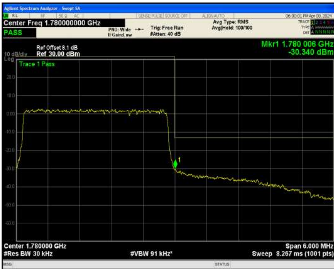
Band66 QPSK BW=5MHz Channel=131997 RB Size=25 Position=#0
