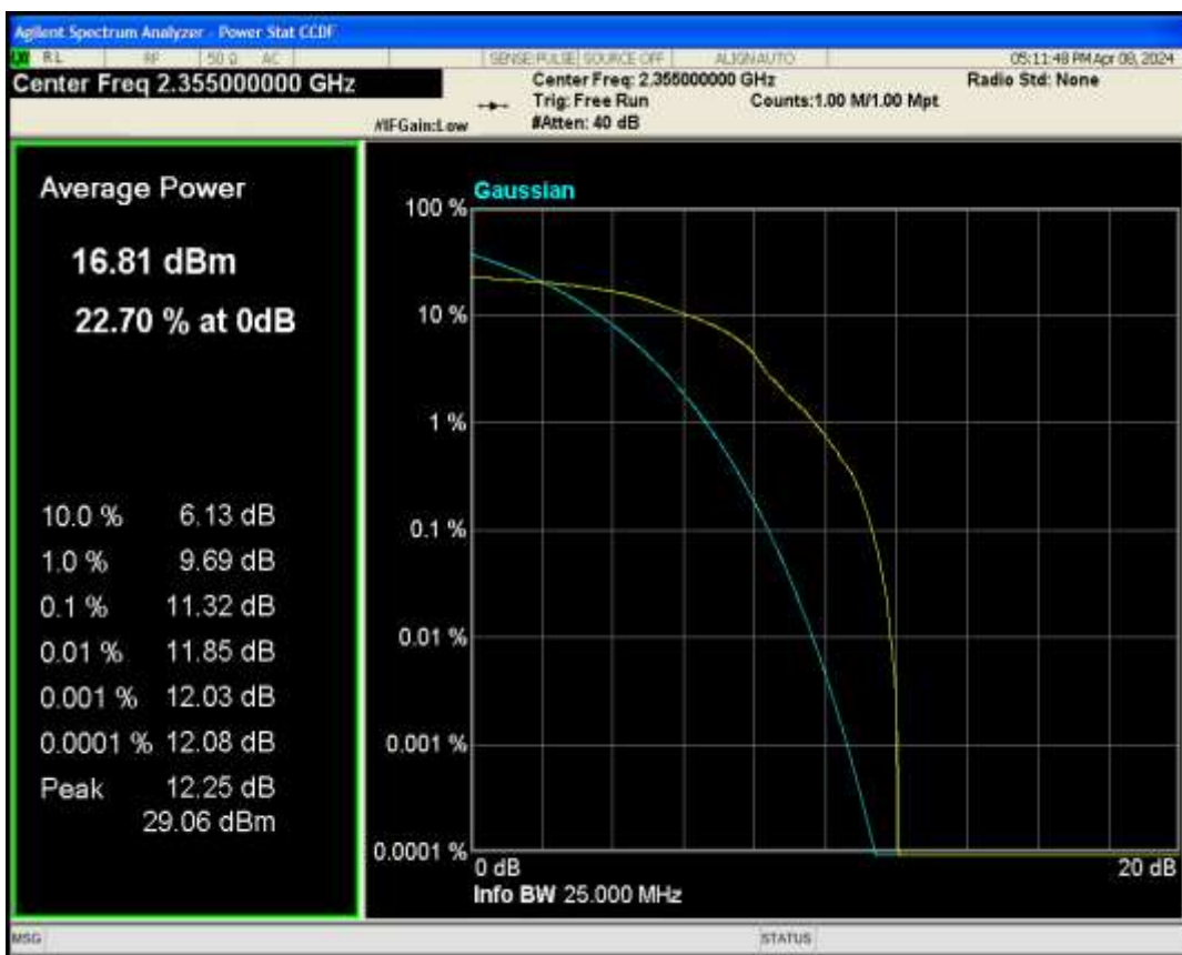
Band40b QPSK BW=10MHz Channel=39200 RB Size=1 Position=#0
