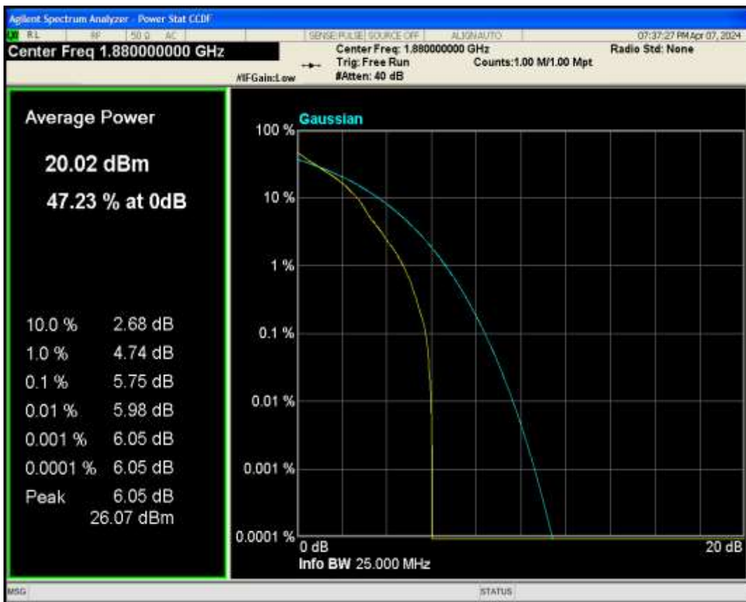
Band2 QAM16 BW=1.4MHz Channel=18900 RB Size=1 Position=#0
