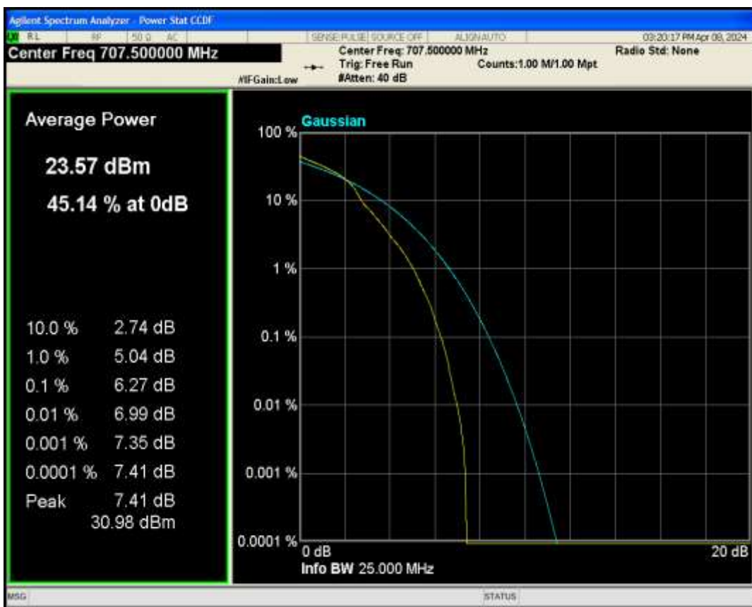
Band12 QPSK BW=10MHz Channel=23095 RB Size=1 Position=#0
