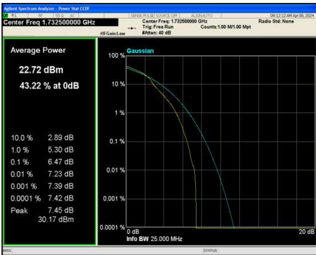
Band4 QPSK BW=10MHz Channel=20175 RB Size=1 Position=#0
