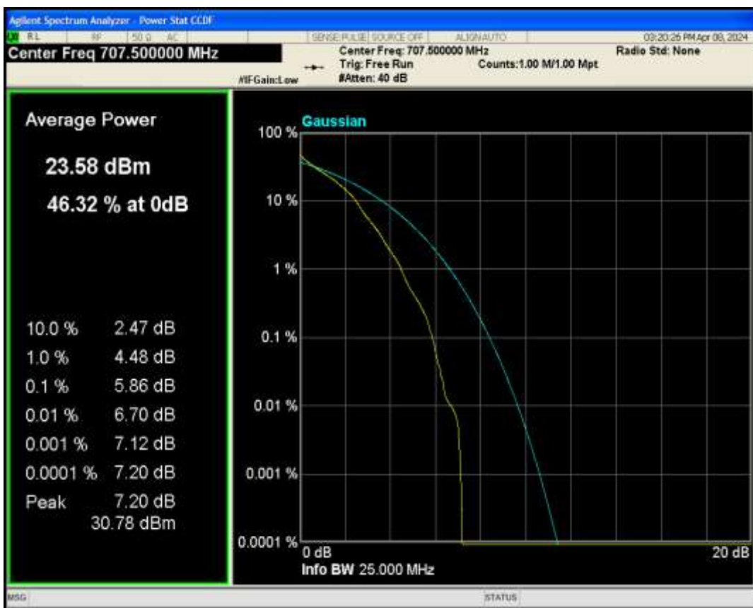
Band12 QAM16 BW=10MHz Channel=23095 RB Size=1 Position=#0
