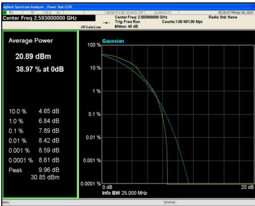
Band41 QPSK BW=20MHz Channel=40620 RB Size=1 Position=#0
