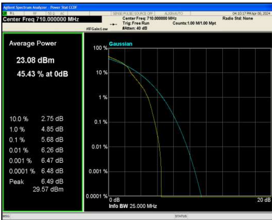
Band17 QAM16 BW=10MHz Channel=23790 RB Size=1 Position=#0
