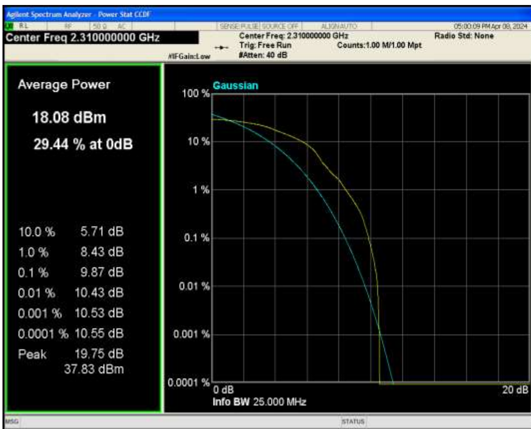
Band40a QPSK BW=10MHz Channel=38750 RB Size=1 Position=#0
