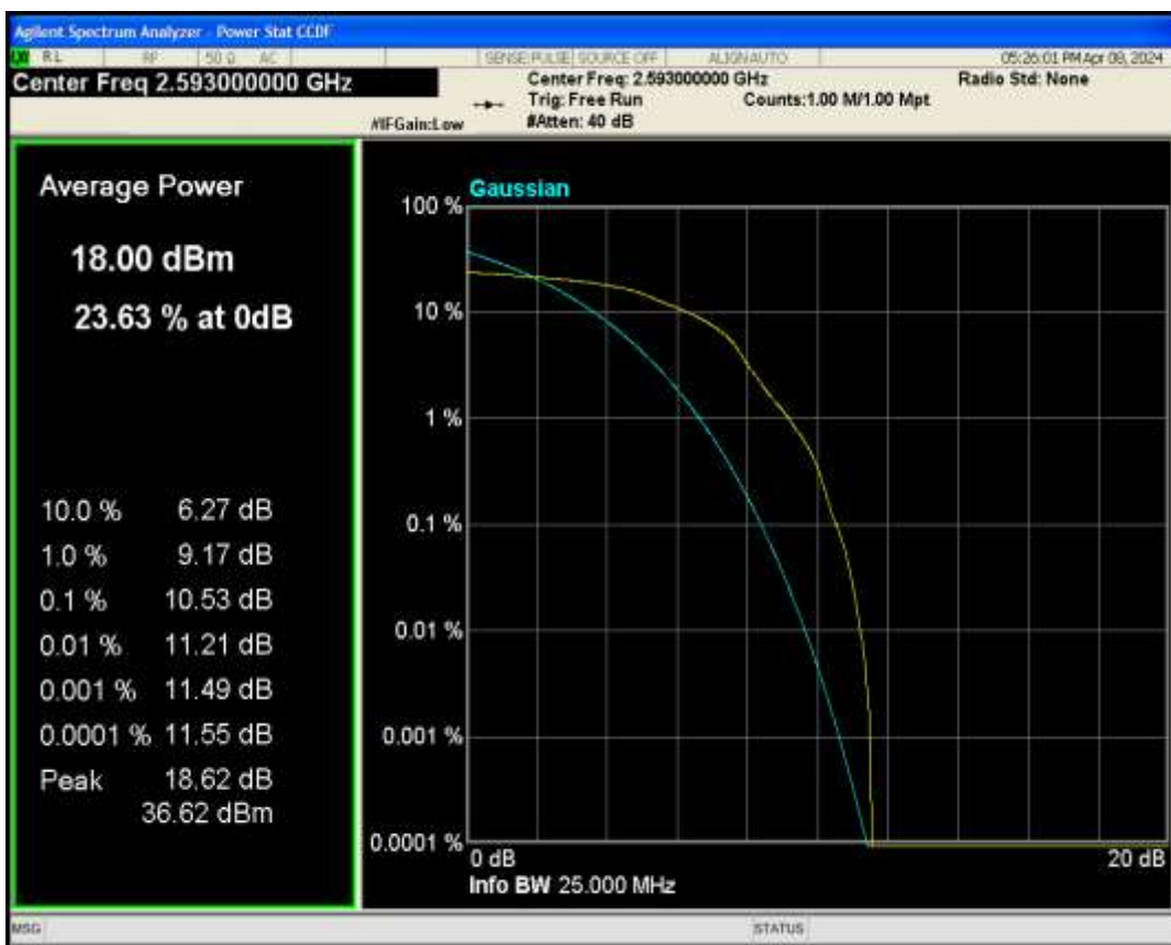
Band41 QPSK BW=15MHz Channel=40620 RB Size=1 Position=#0
