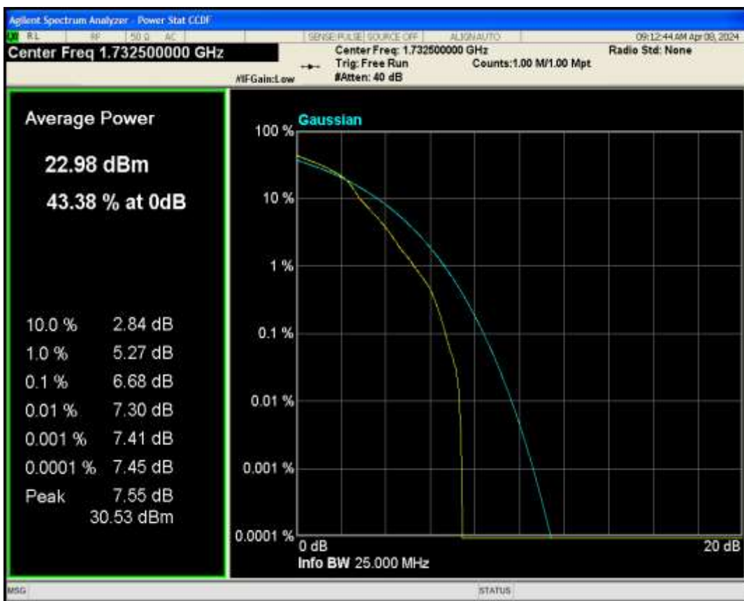
Band4 QPSK BW=20MHz Channel=20175 RB Size=1 Position=#0
