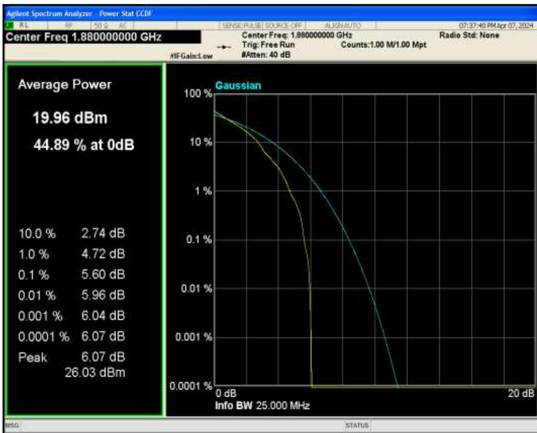
Band2 QAM16 BW=5MHz Channel=18900 RB Size=1 Position=#0
