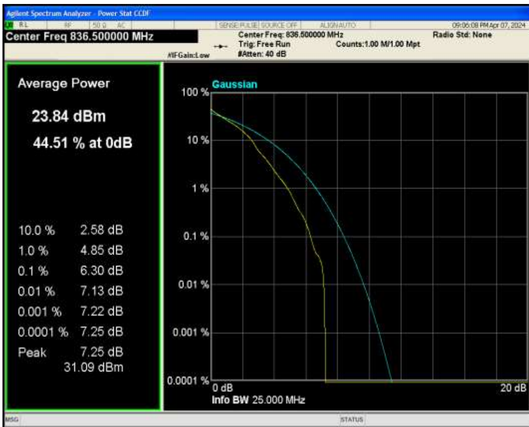
Band5 QAM16 BW=10MHz Channel=20525 RB Size=1 Position=#0
