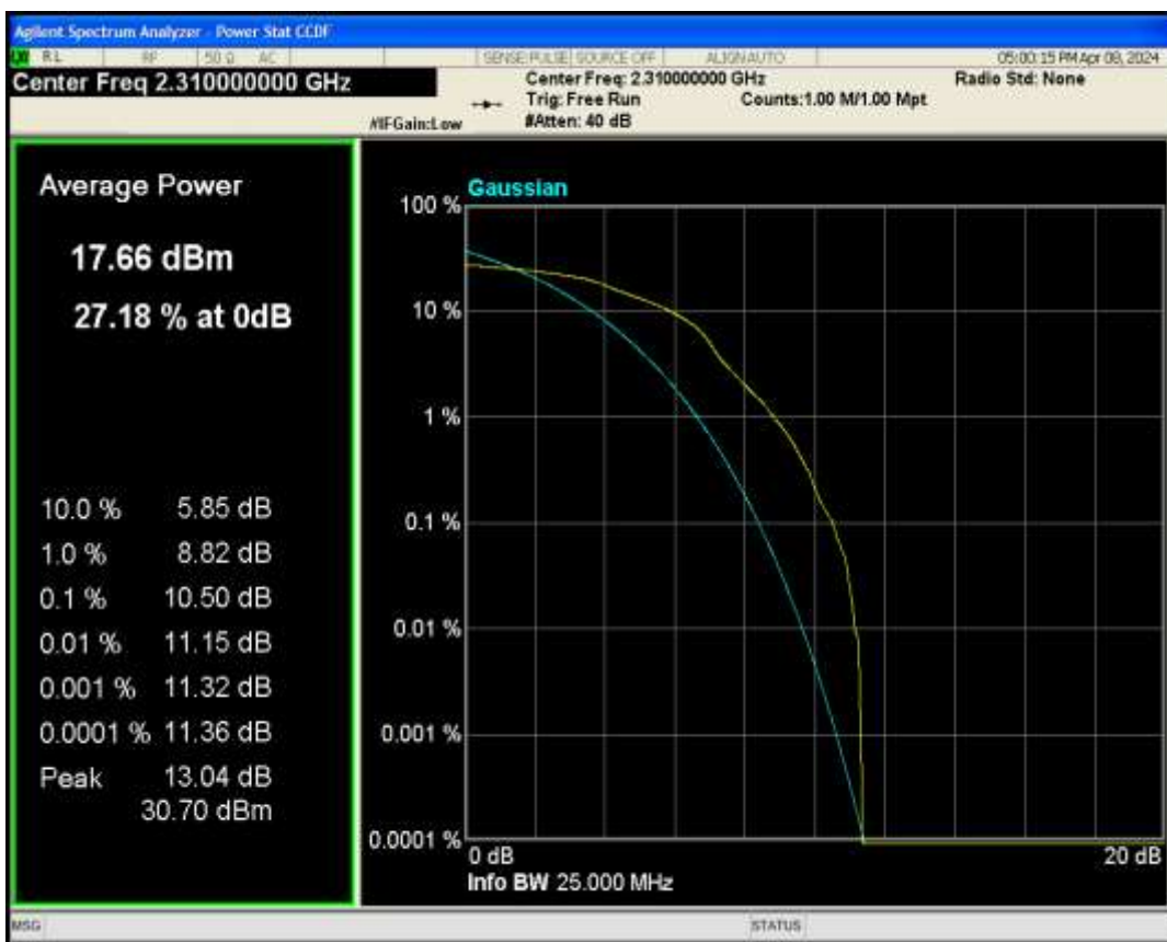
Band40b QPSK BW=5MHz Channel=39200 RB Size=1 Position=#0
