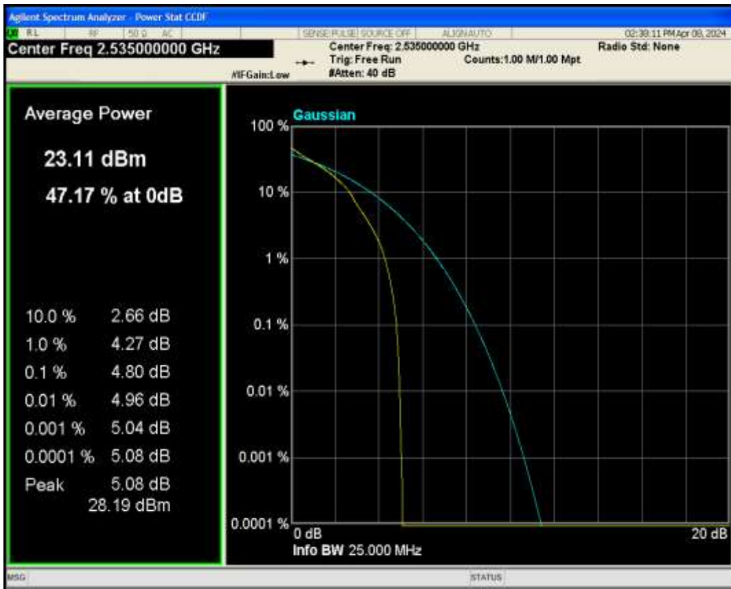
Band7 QAM16 BW=20MHz Channel=21100 RB Size=1 Position=#0
