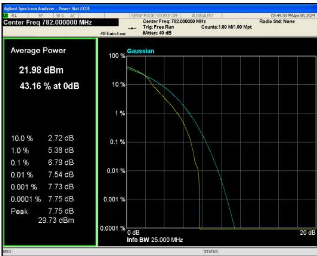
Band13 QAM16 BW=10MHz Channel=23230 RB Size=1 Position=#0
