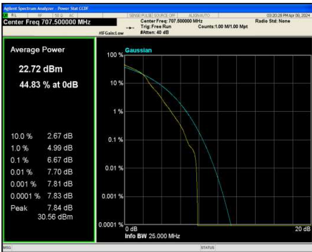
Band13 QPSK BW=5MHz Channel=23230 RB Size=1 Position=#0
