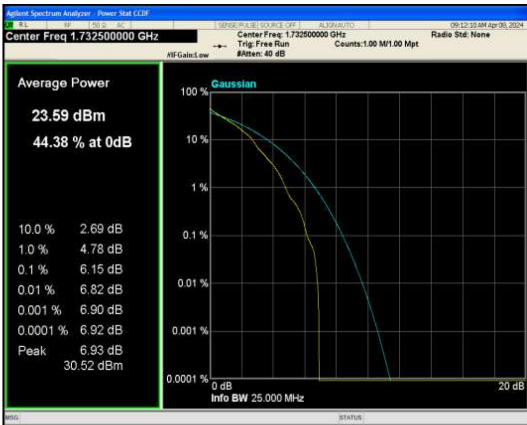
Band4 QAM16 BW=5MHz Channel=20175 RB Size=1 Position=#0
