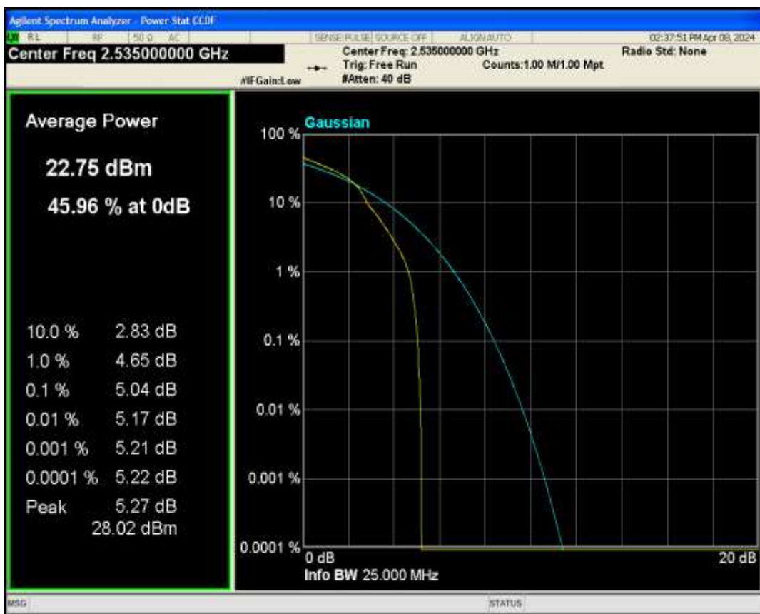
Band7 QAM16 BW=10MHz Channel=21100 RB Size=1 Position=#0
