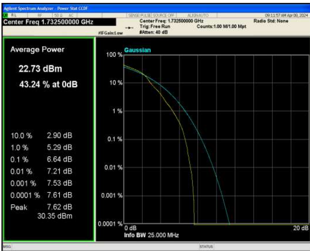
Band4 QPSK BW=5MHz Channel=20175 RB Size=1 Position=#0
