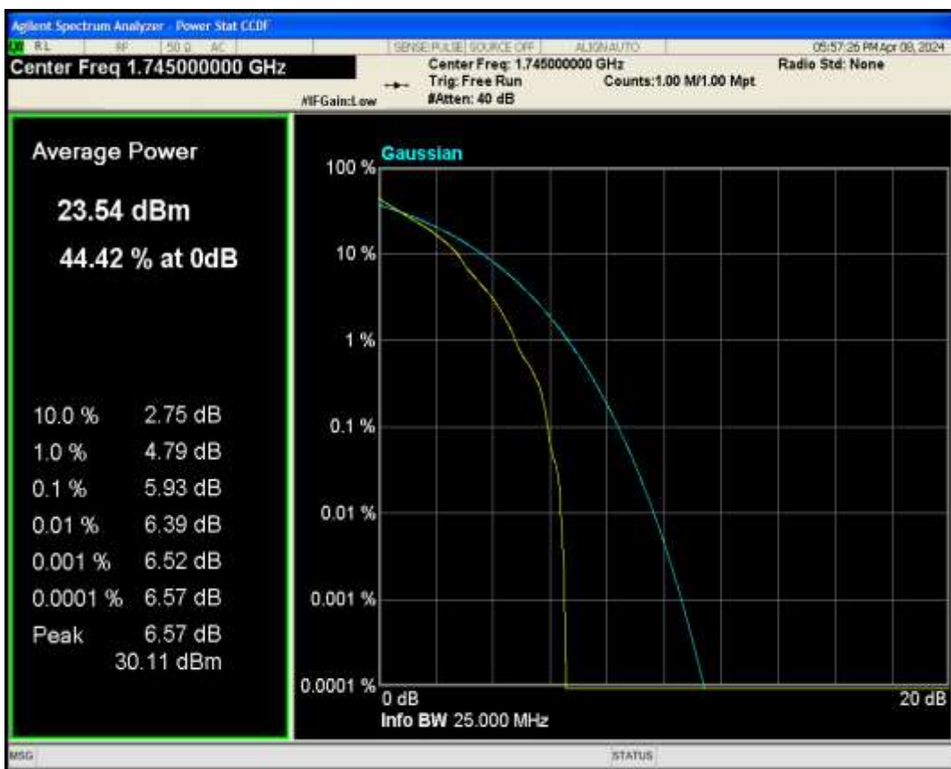
Band66 QAM16 BW=5MHz Channel=132322 RB Size=1 Position=#0
