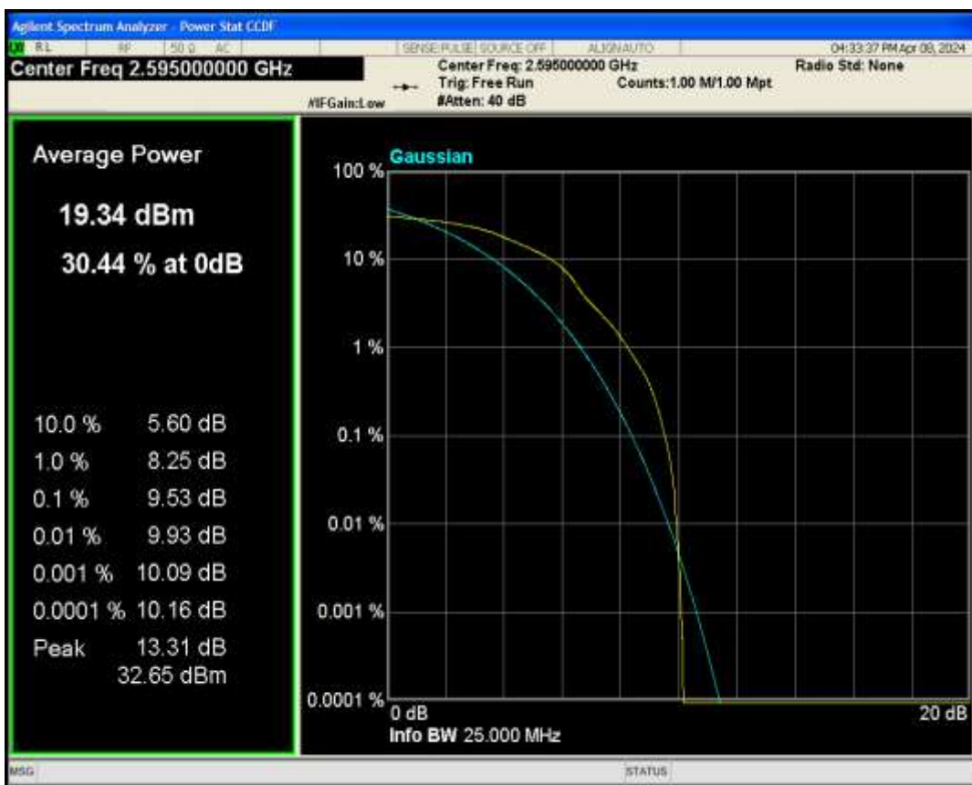
Band38 QPSK BW=10MHz Channel=38000 RB Size=1 Position=#0
