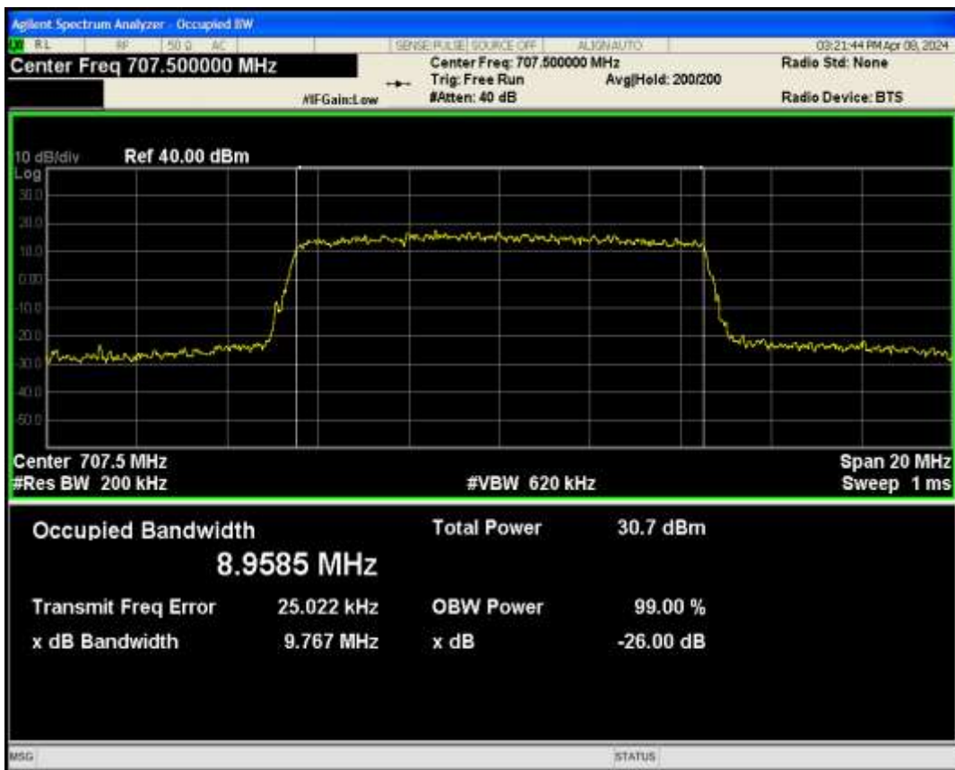
Band13 QPSK BW=5MHz Channel=23230 RB Size=25 Position=#0
