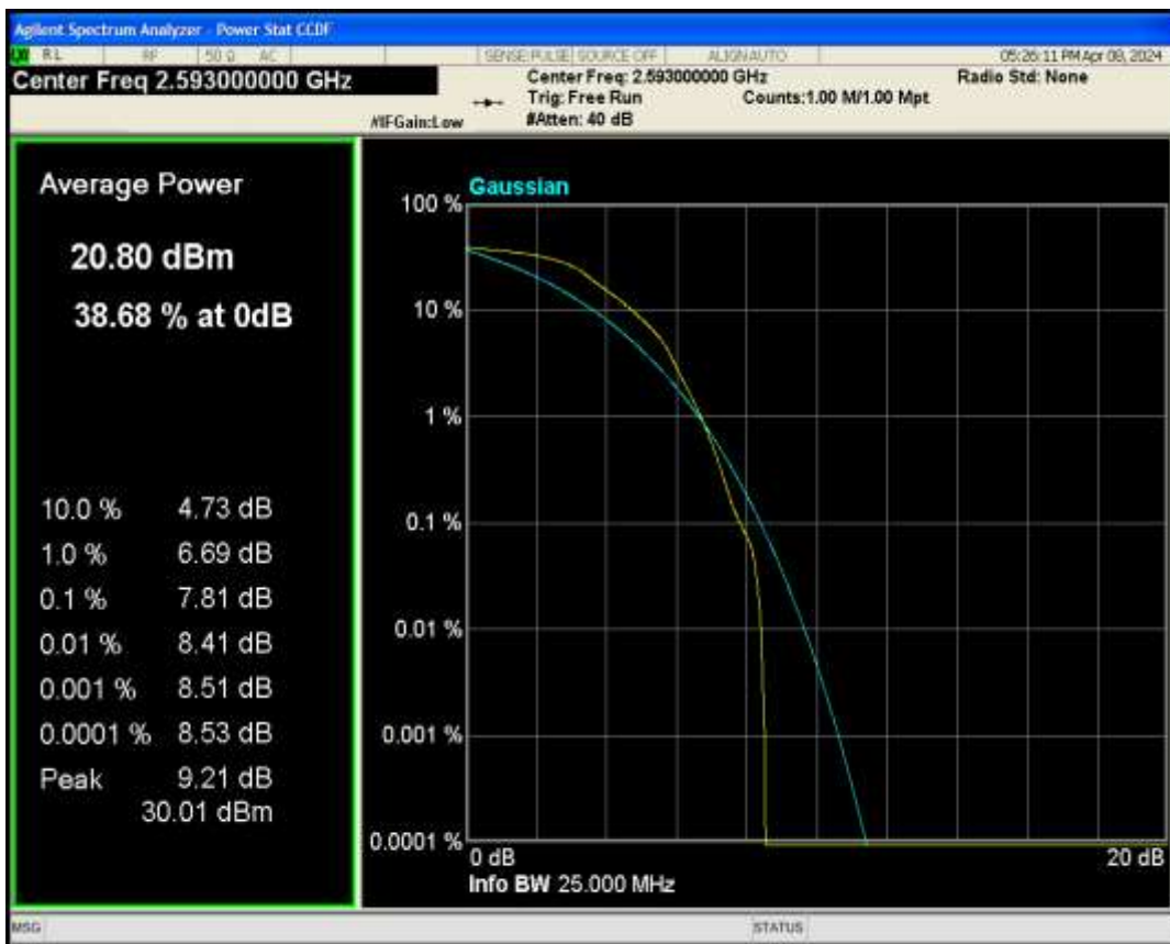
Band41 QAM16 BW=20MHz Channel=40620 RB Size=1 Position=#0
