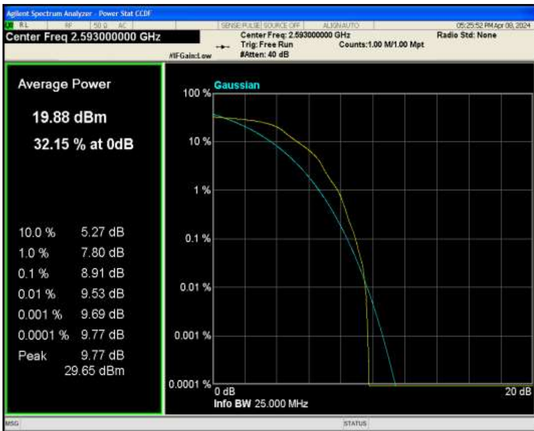
Band41 QAM16 BW=5MHz Channel=40620 RB Size=1 Position=#0
