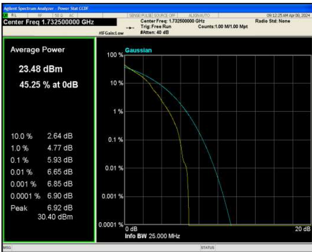
Band4 QAM16 BW=10MHz Channel=20175 RB Size=1 Position=#0
