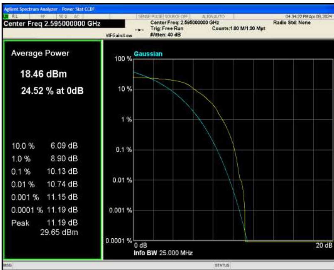
Band38 QAM16 BW=20MHz Channel=38000 RB Size=1 Position=#0
