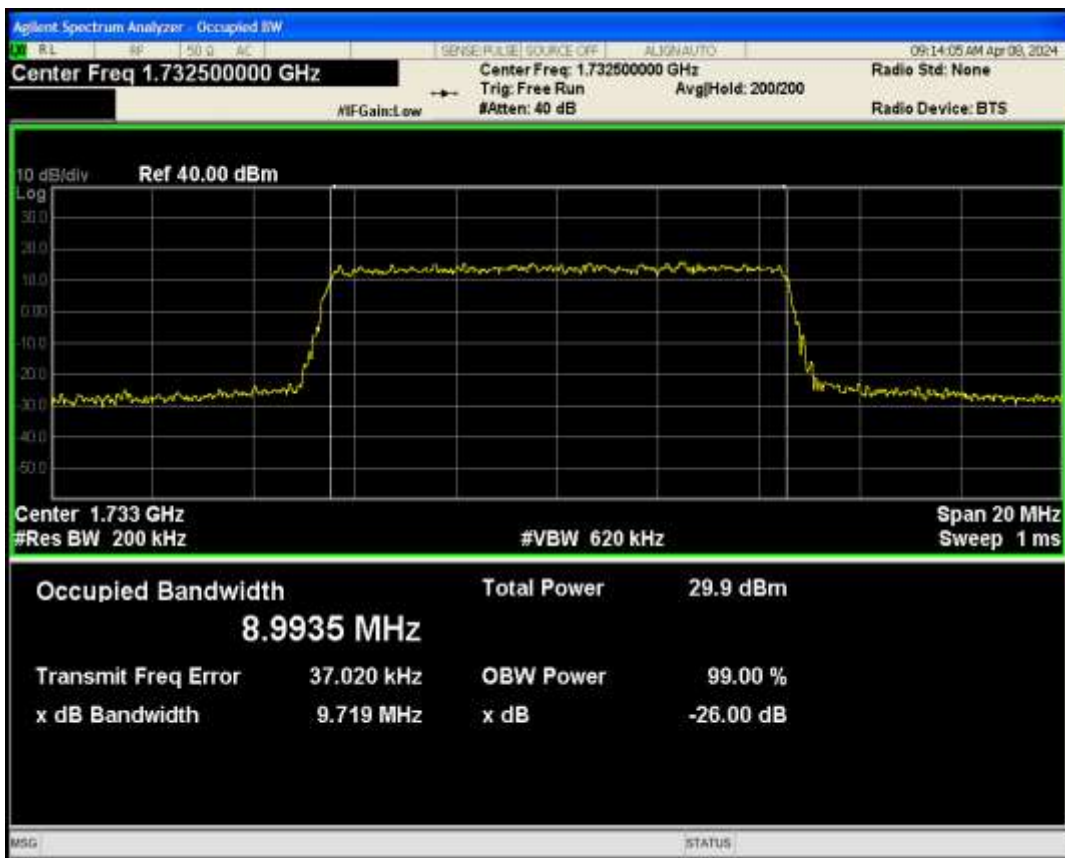
Band4 QPSK BW=15MHz Channel=20175 RB Size=75 Position=#0
