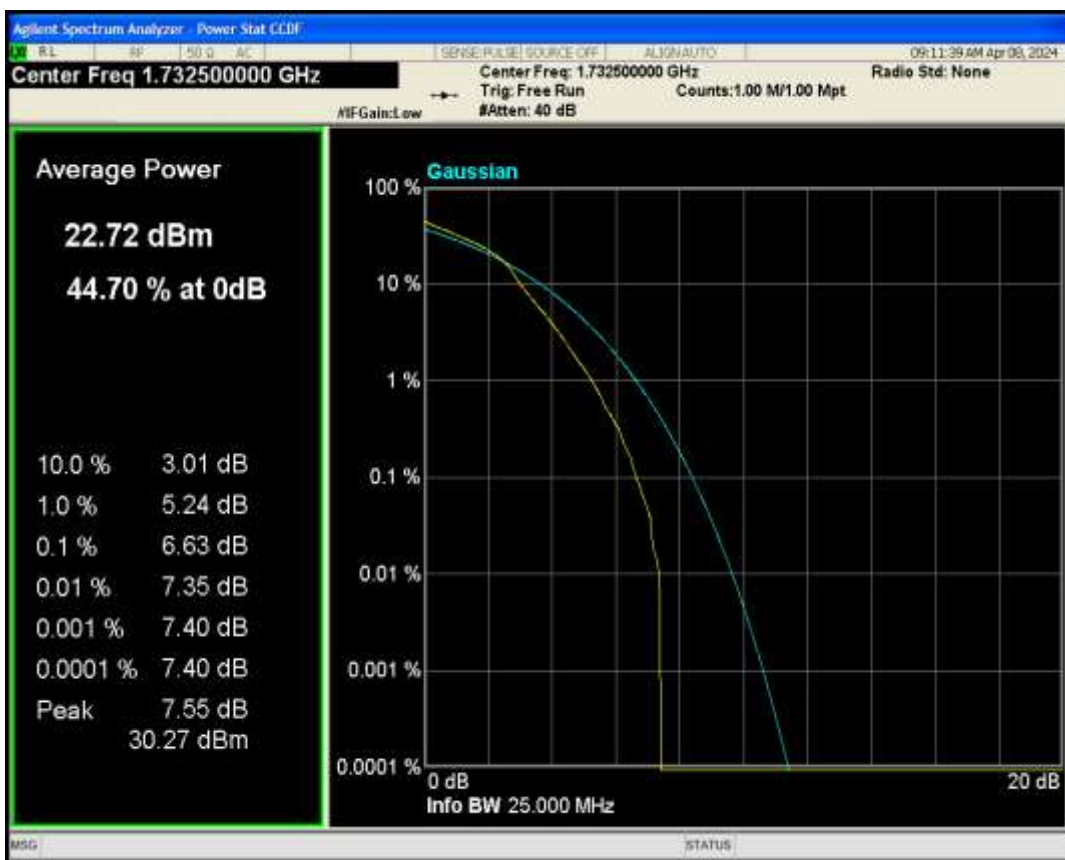
Band4 QPSK BW=3MHz Channel=20175 RB Size=1 Position=#0
