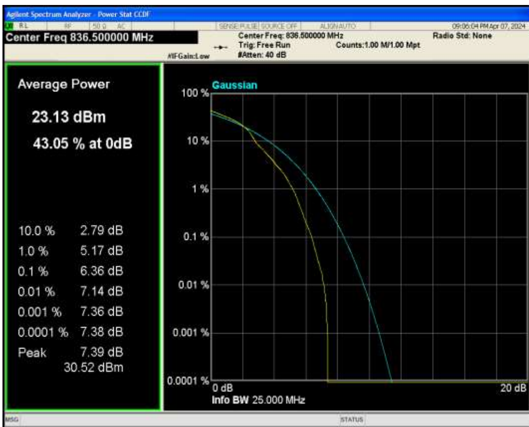
Band5 QPSK BW=10MHz Channel=20525 RB Size=1 Position=#0
