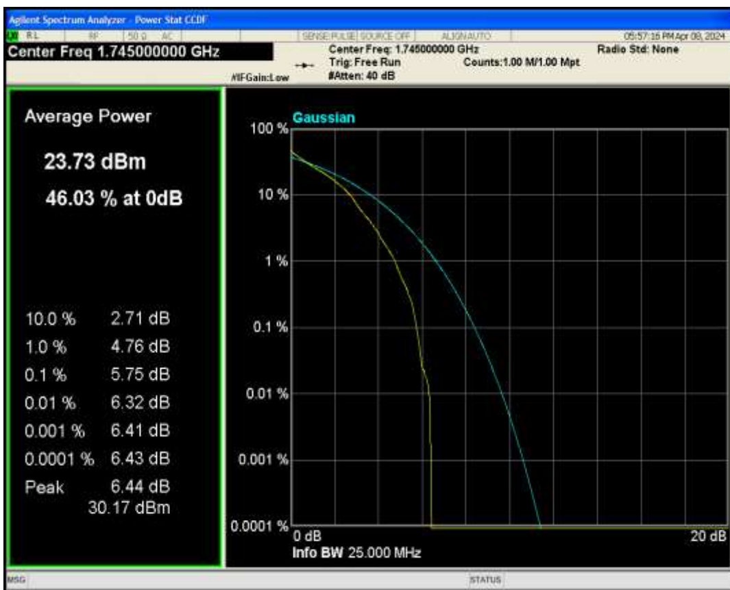
Band66 QAM16 BW=3MHz Channel=132322 RB Size=1 Position=#0
