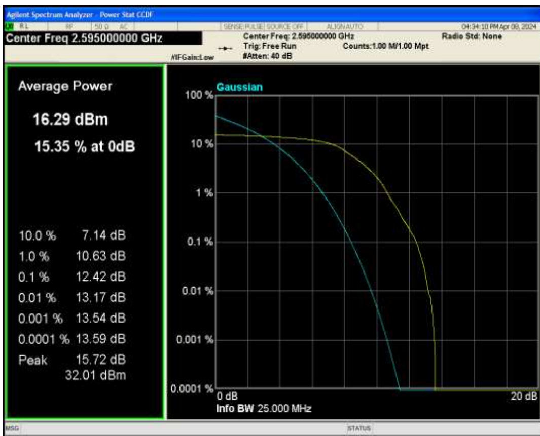
Band38 QAM16 BW=10MHz Channel=38000 RB Size=1 Position=#0
