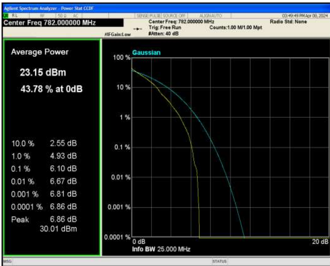
Band13 QAM16 BW=5MHz Channel=23230 RB Size=1 Position=#0
