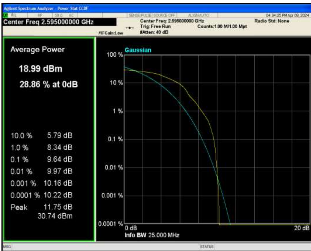
Band4 QPSK BW=1.4MHz Channel=20175 RB Size=1 Position=#0
