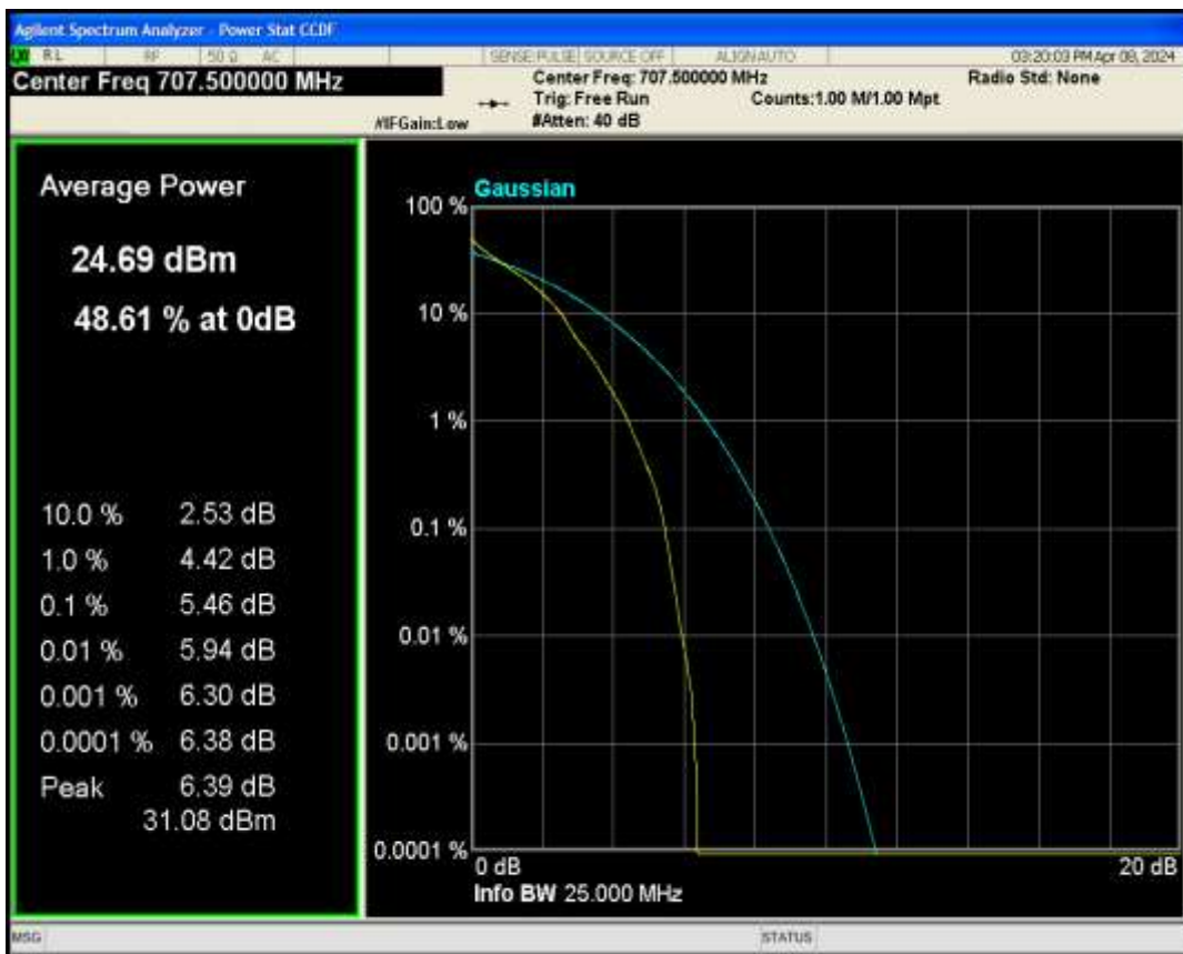
Band12 QPSK BW=5MHz Channel=23095 RB Size=1 Position=#0
