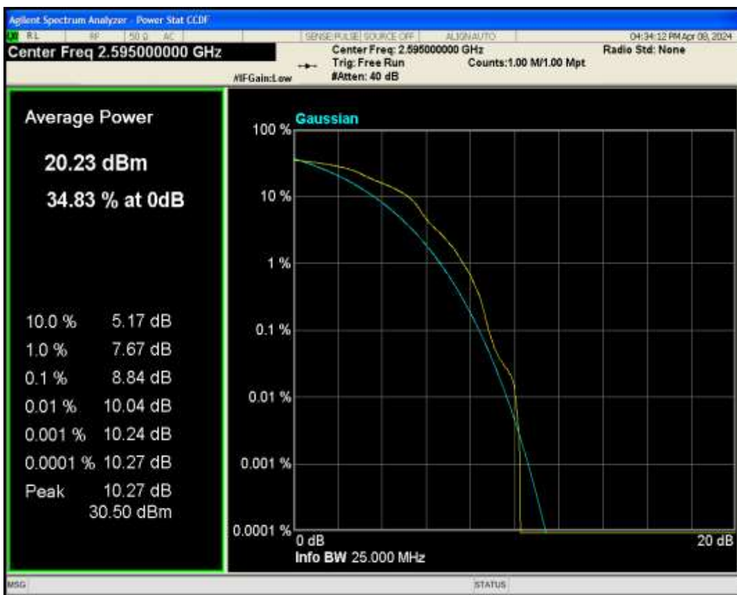
Band38 QPSK BW=15MHz Channel=38000 RB Size=1 Position=#0
