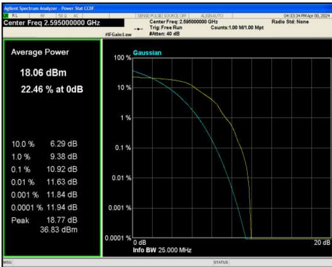
Band38 QAM16 BW=5MHz Channel=38000 RB Size=1 Position=#0
