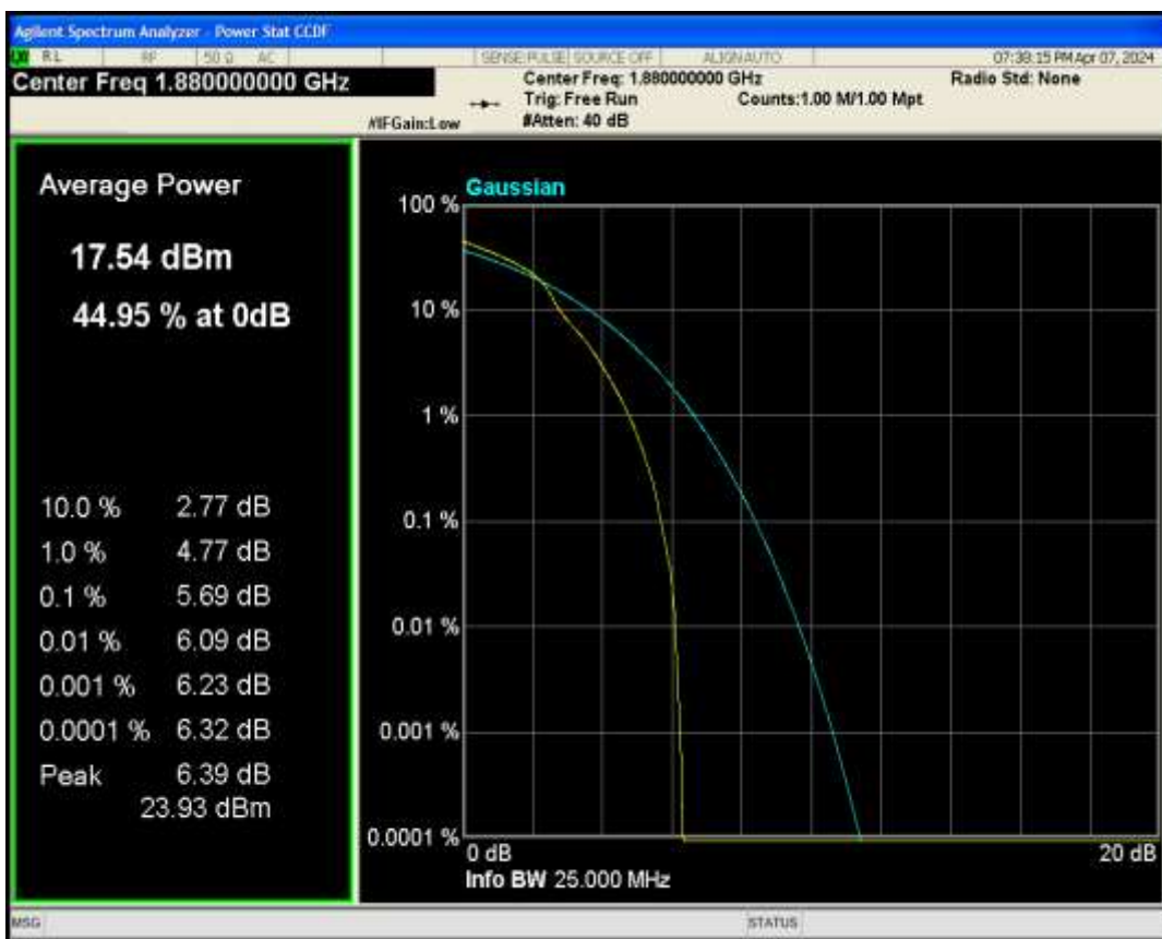
Band38 QPSK BW=5MHz Channel=38000 RB Size=1 Position=#0
