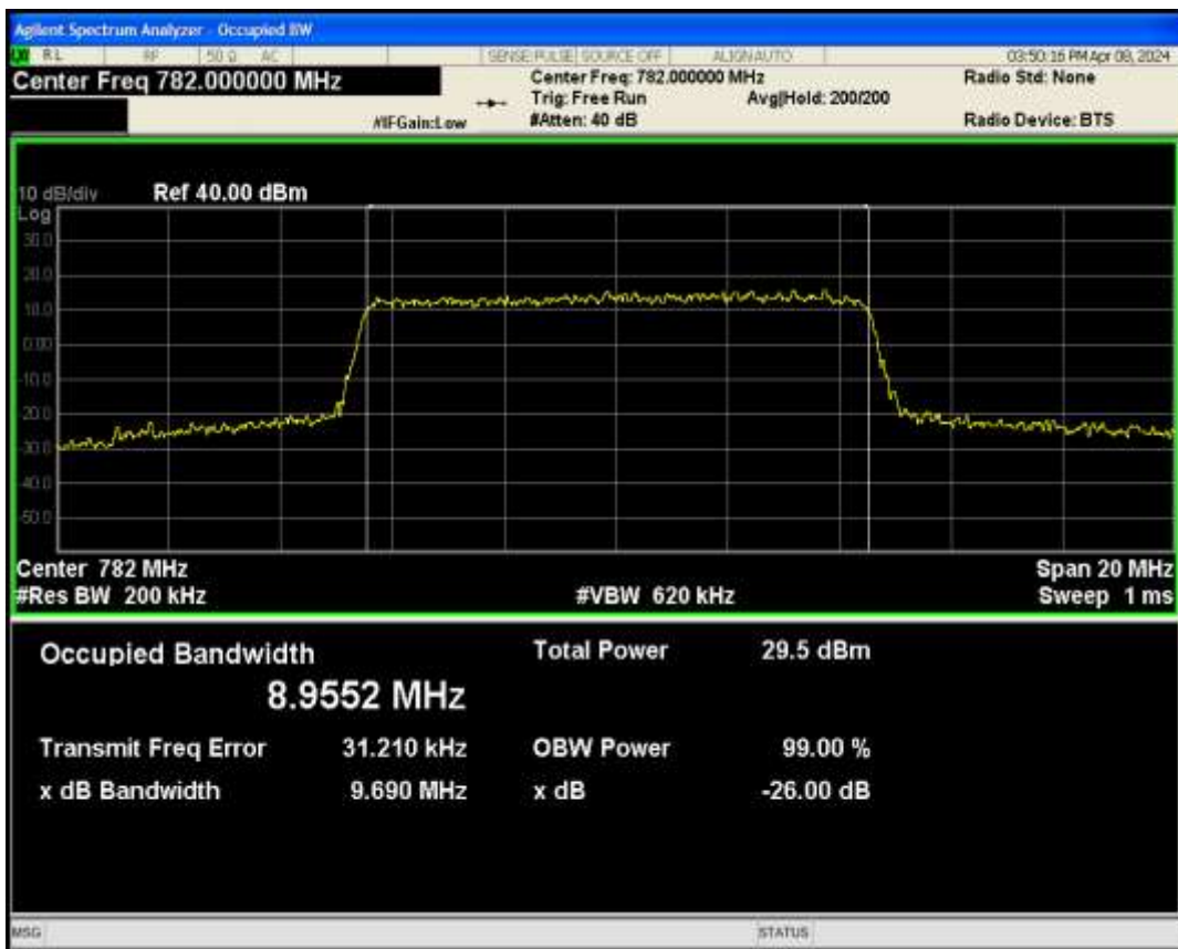
Band17 QPSK BW=5MHz Channel=23790 RB Size=25 Position=#0
