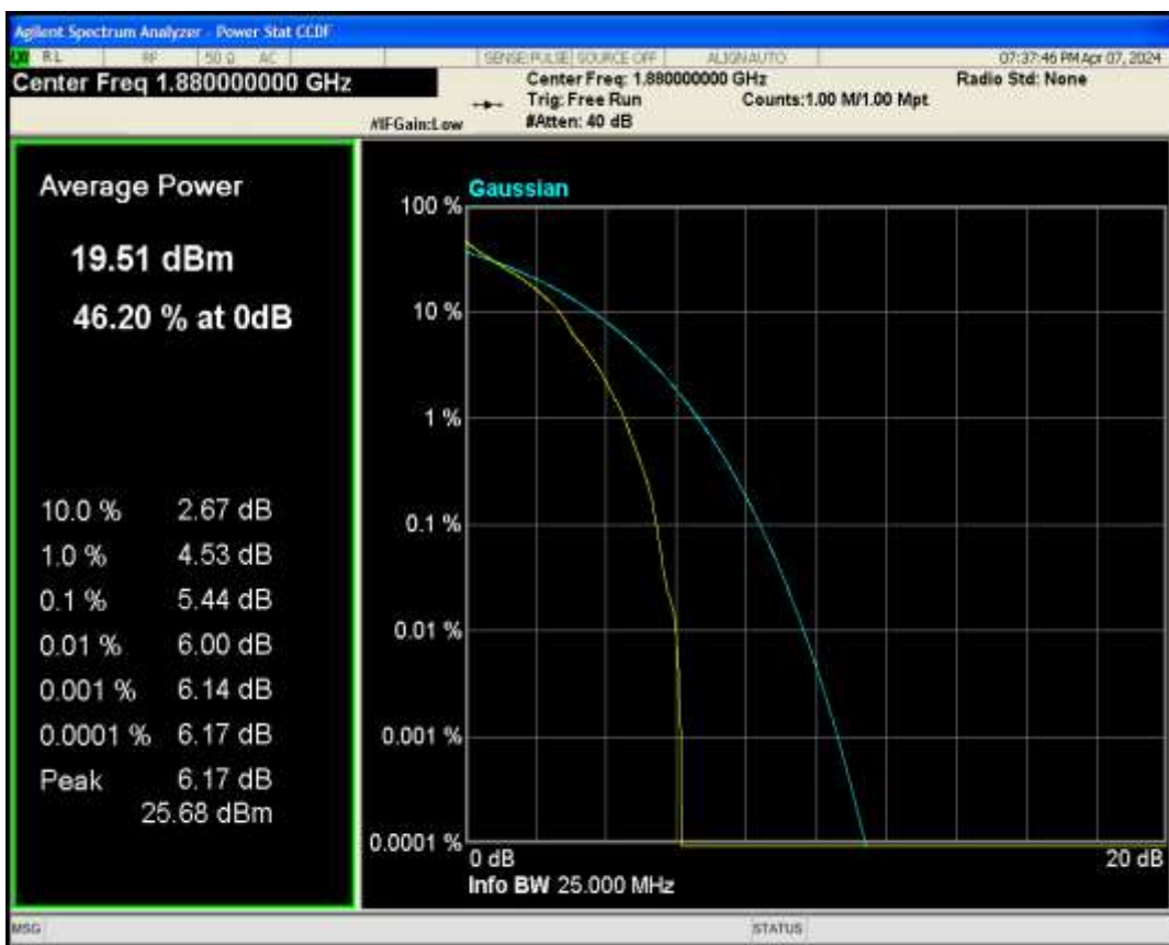
Band2 QAM16 BW=10MHz Channel=18900 RB Size=1 Position=#0
