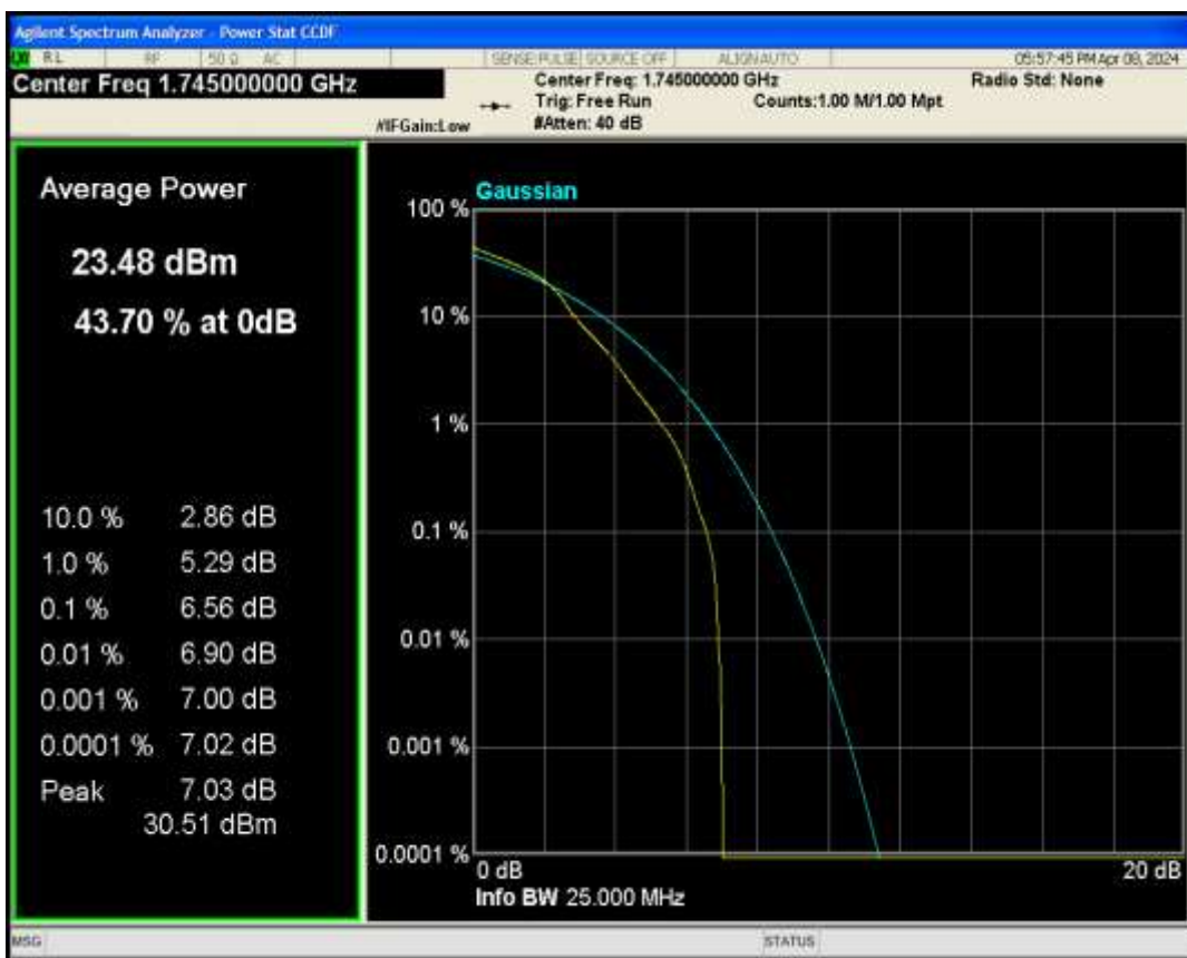
Band66 QPSK BW=20MHz Channel=132322 RB Size=1 Position=#0
