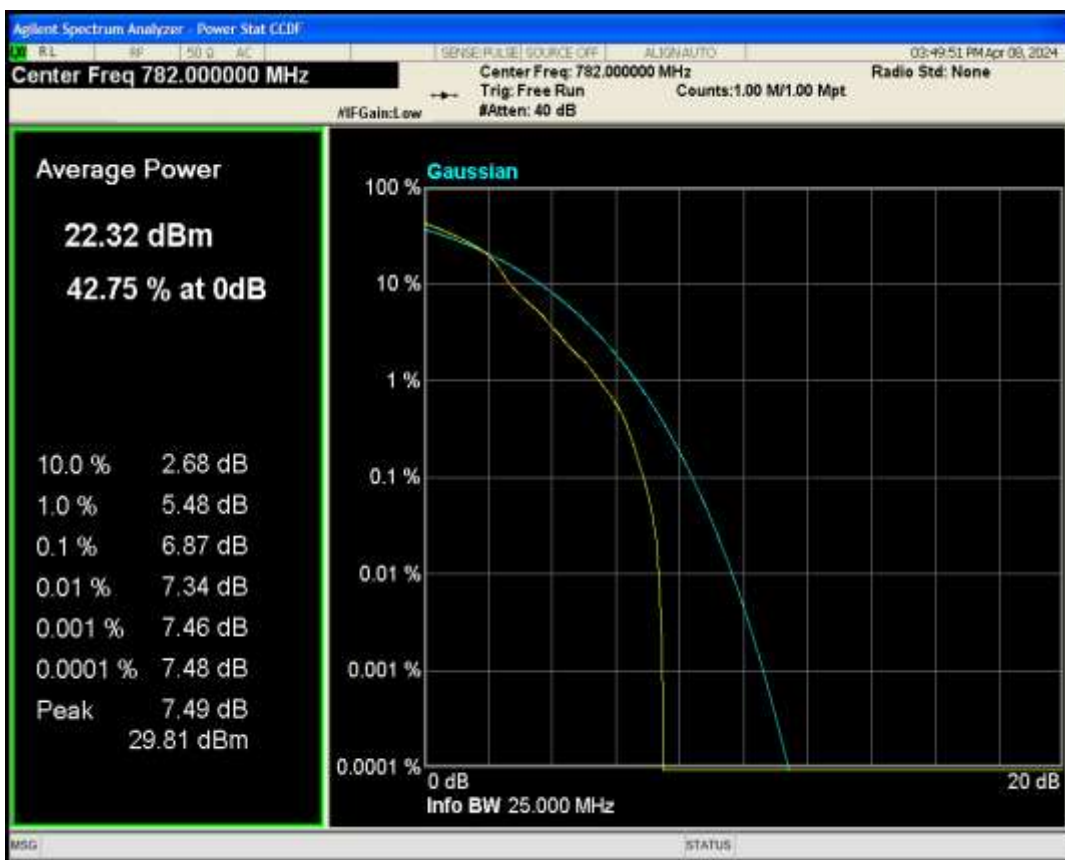
Band17 QPSK BW=5MHz Channel=23790 RB Size=1 Position=#0
