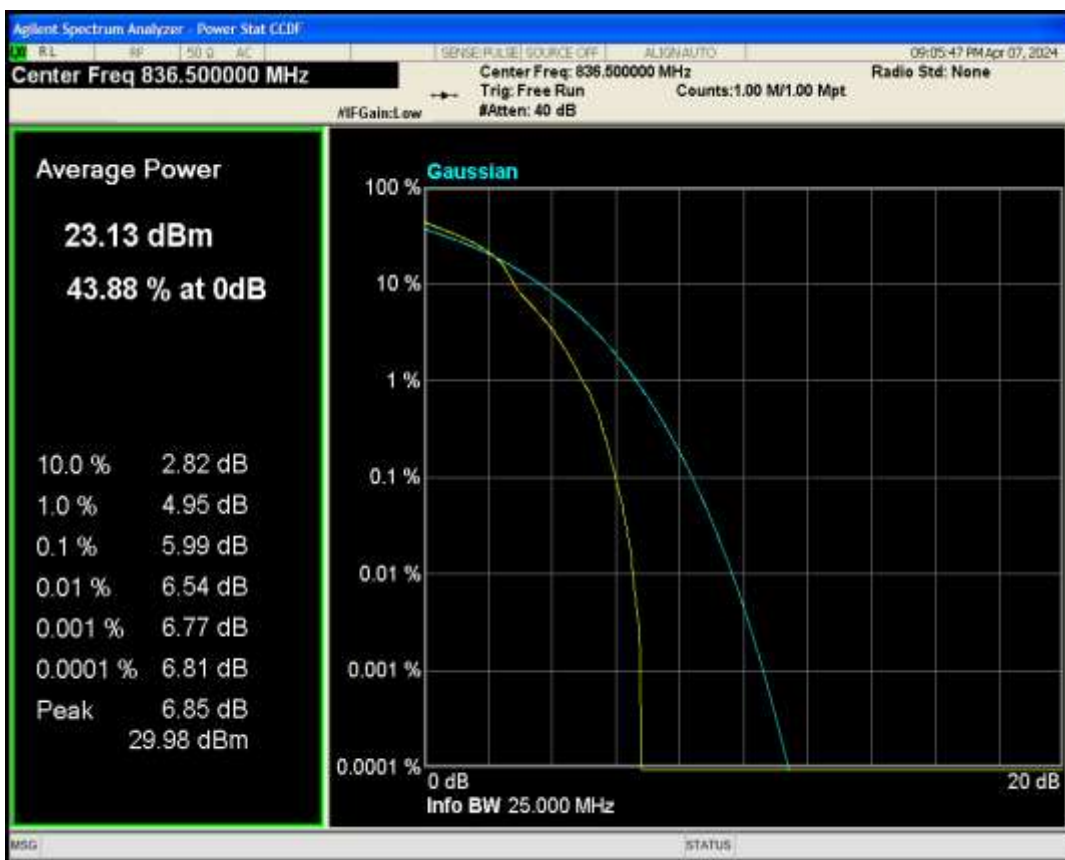
Band5 QPSK BW=3MHz Channel=20525 RB Size=1 Position=#0
