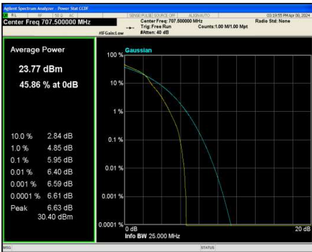
Band12 QPSK BW=3MHz Channel=23095 RB Size=1 Position=#0
