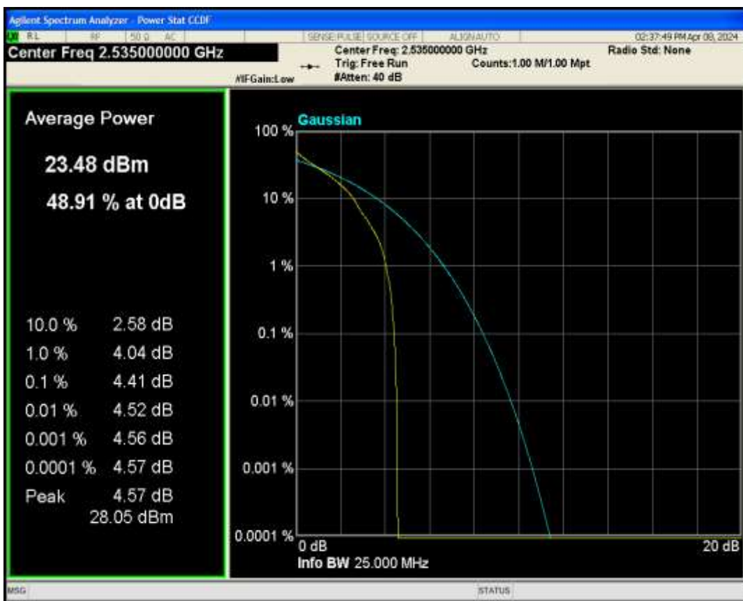
Band7 QAM16 BW=5MHz Channel=21100 RB Size=1 Position=#0
