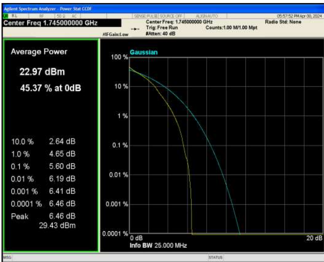
Band66 QAM16 BW=20MHz Channel=132322 RB Size=1 Position=#0
