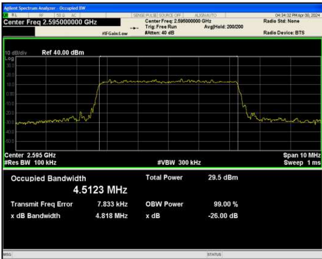
Band38 QPSK BW=10MHz Channel=38000 RB Size=50 Position=#0
