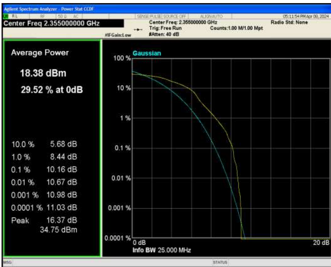
Band41 QPSK BW=5MHz Channel=40620 RB Size=1 Position=#0
