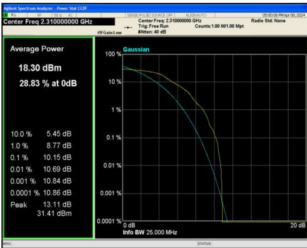
Band40a QAM16 BW=5MHz Channel=38750 RB Size=1 Position=#0
