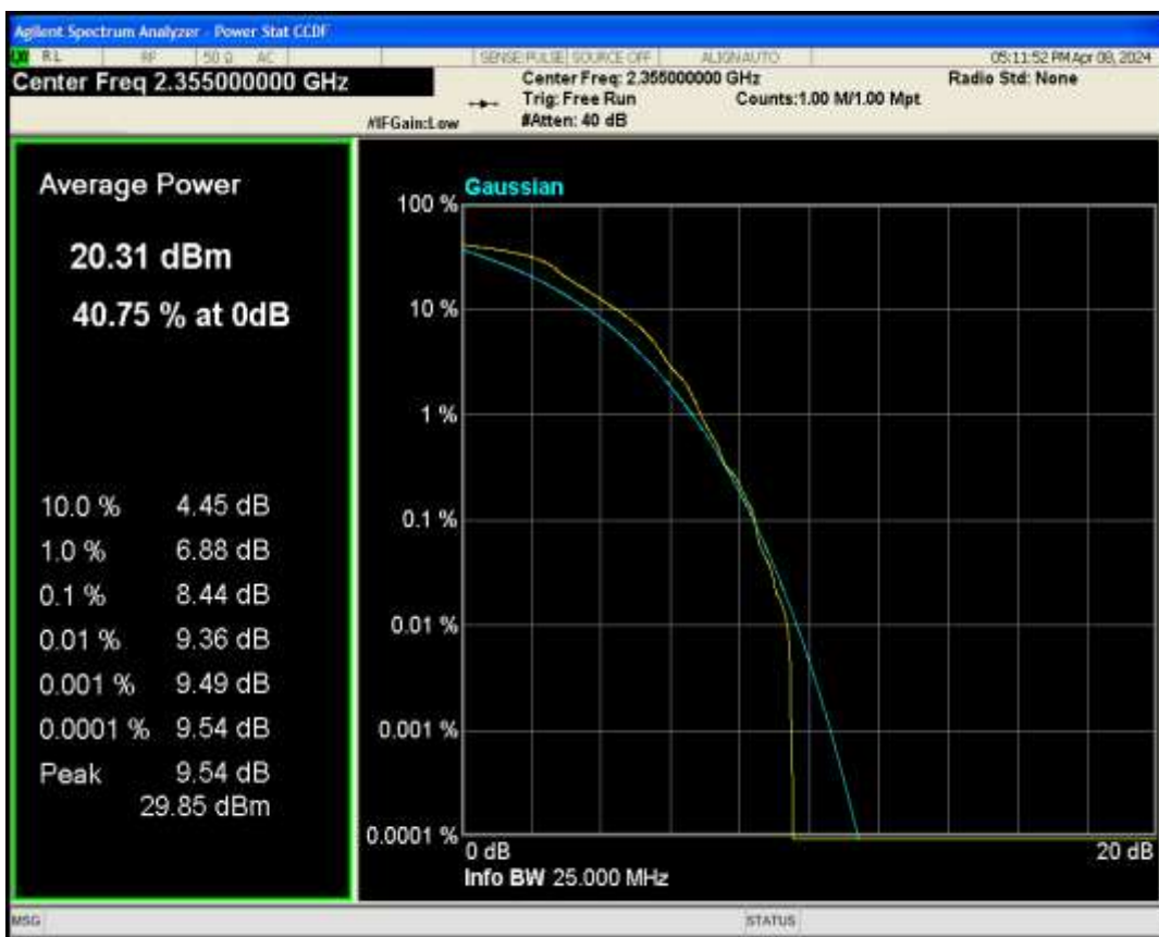
Band40b QAM16 BW=10MHz Channel=39200 RB Size=1 Position=#0
