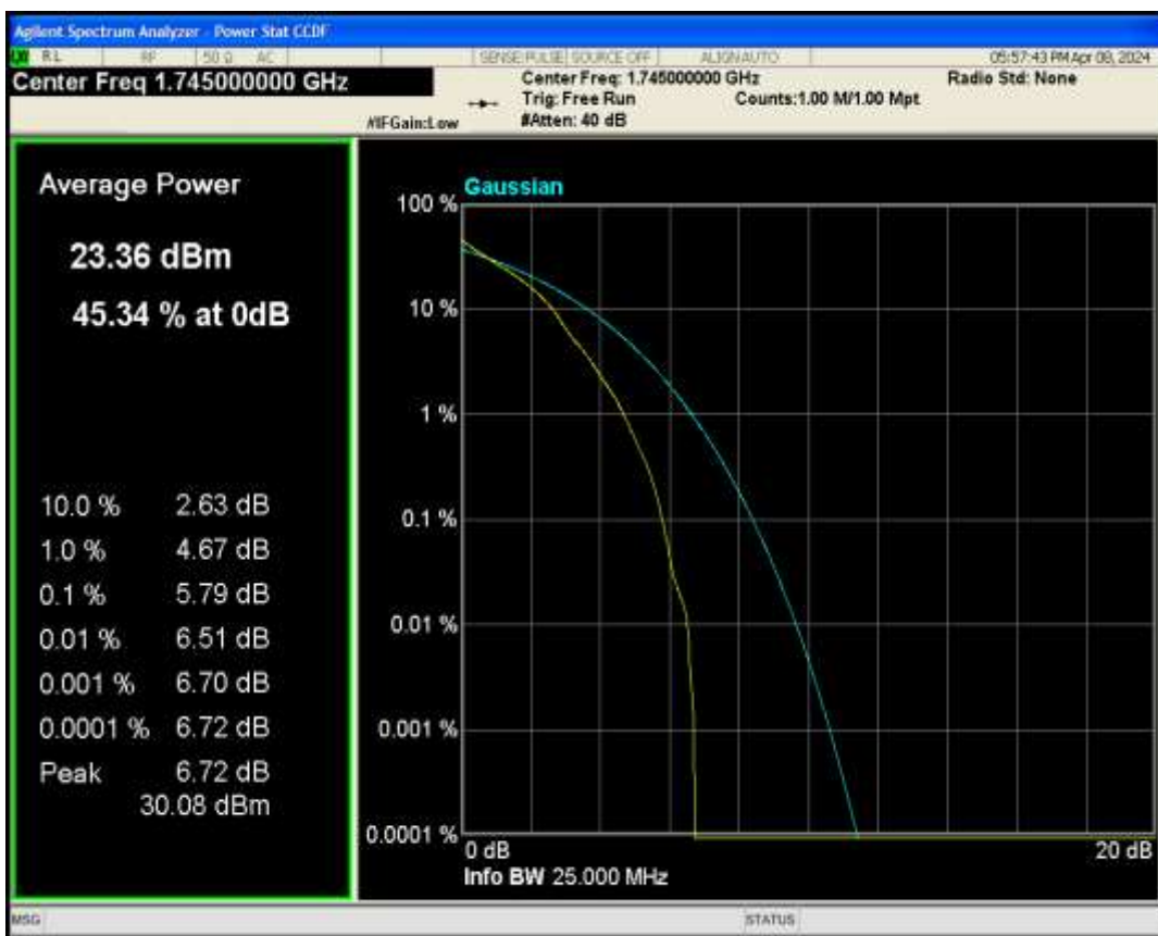
Band66 QAM16 BW=15MHz Channel=132322 RB Size=1 Position=#0
