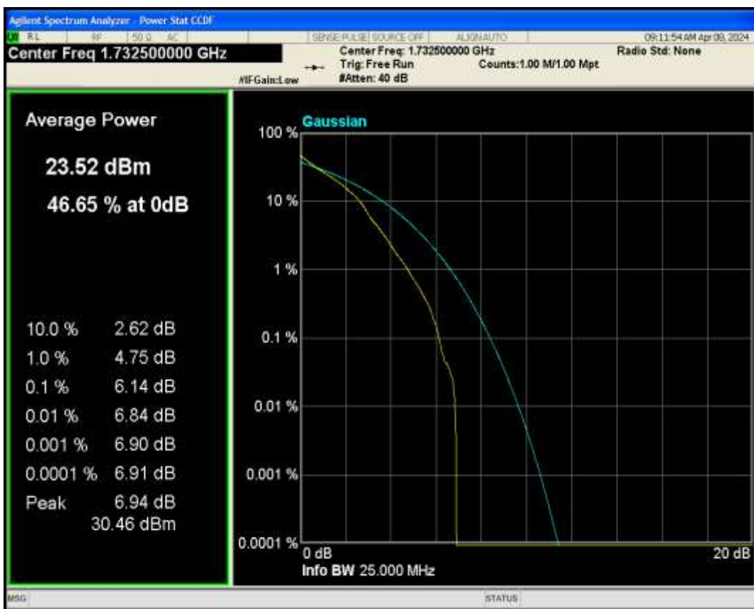
Band4 QAM16 BW=3MHz Channel=20175 RB Size=1 Position=#0
