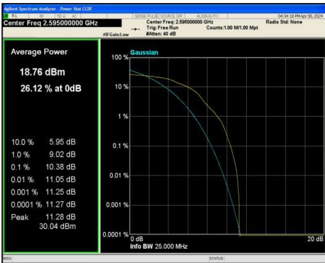
Band38 QPSK BW=20MHz Channel=38000 RB Size=1 Position=#0
