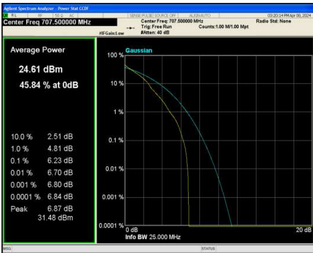
Band12 QAM16 BW=3MHz Channel=23095 RB Size=1 Position=#0
