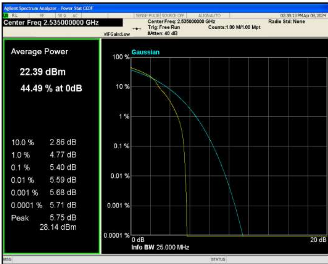
Band7 QAM16 BW=20MHz Channel=21100 RB Size=1 Position=#0
