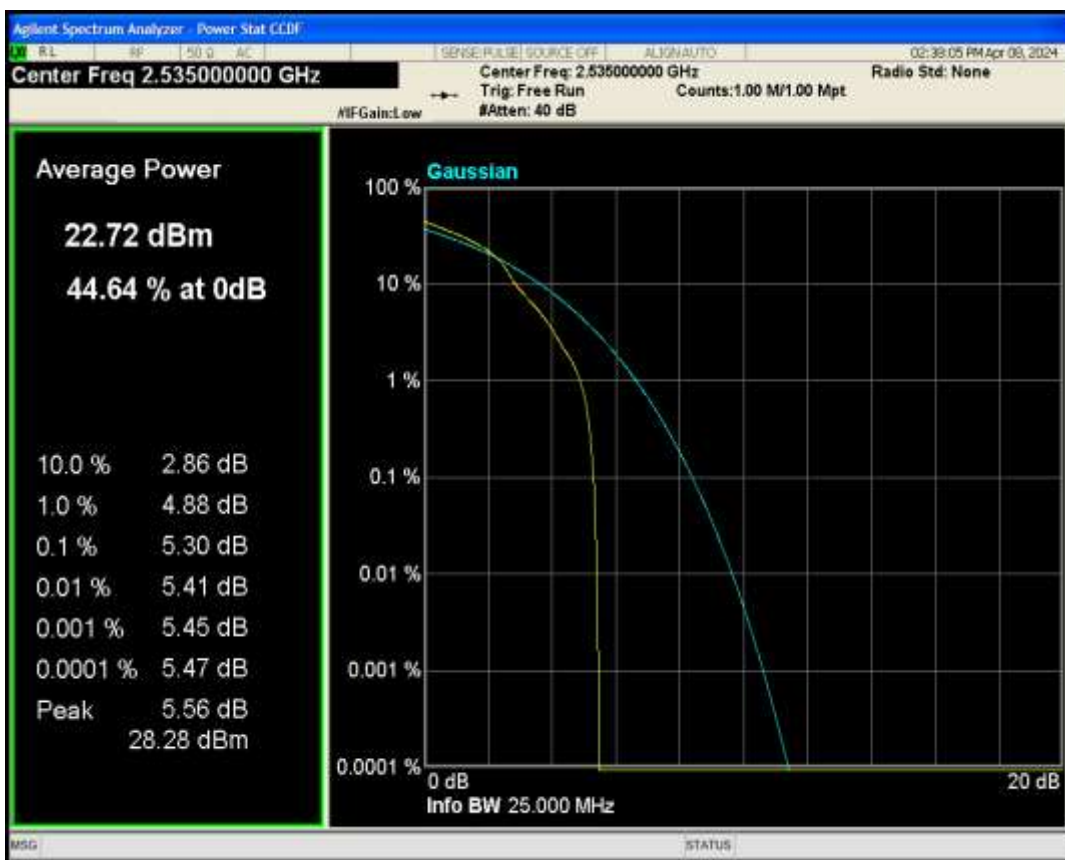
Band7 QPSK BW=20MHz Channel=21100 RB Size=1 Position=#0
