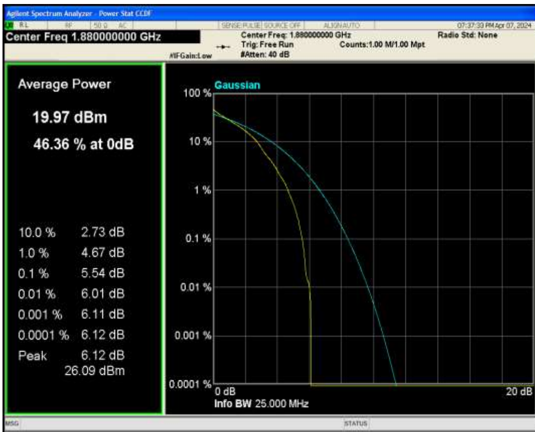
Band2 QAM16 BW=3MHz Channel=18900 RB Size=1 Position=#0
