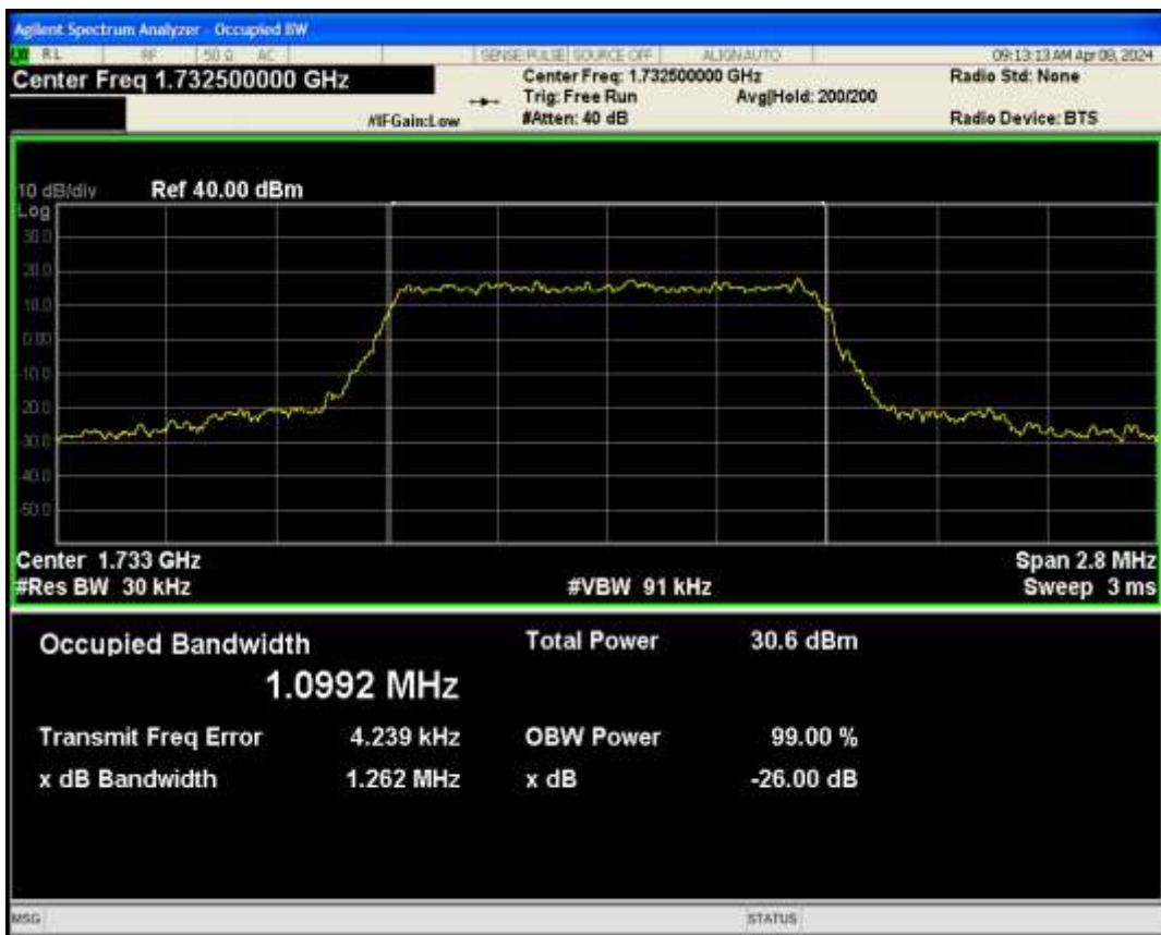
Band4 QAM16 BW=1.4MHz Channel=20175 RB Size=6 Position=#0
