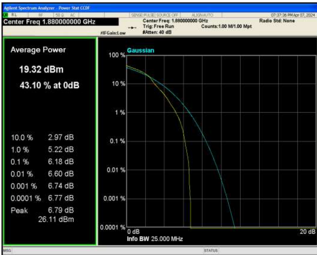
Band2 QPSK BW=5MHz Channel=18900 RB Size=1 Position=#0
