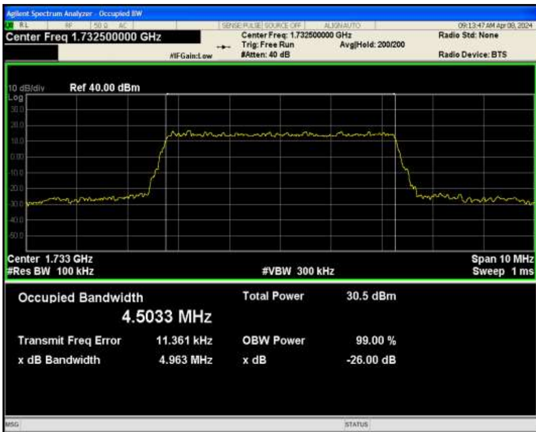
Band4 QAM16 BW=5MHz Channel=20175 RB Size=25 Position=#0
