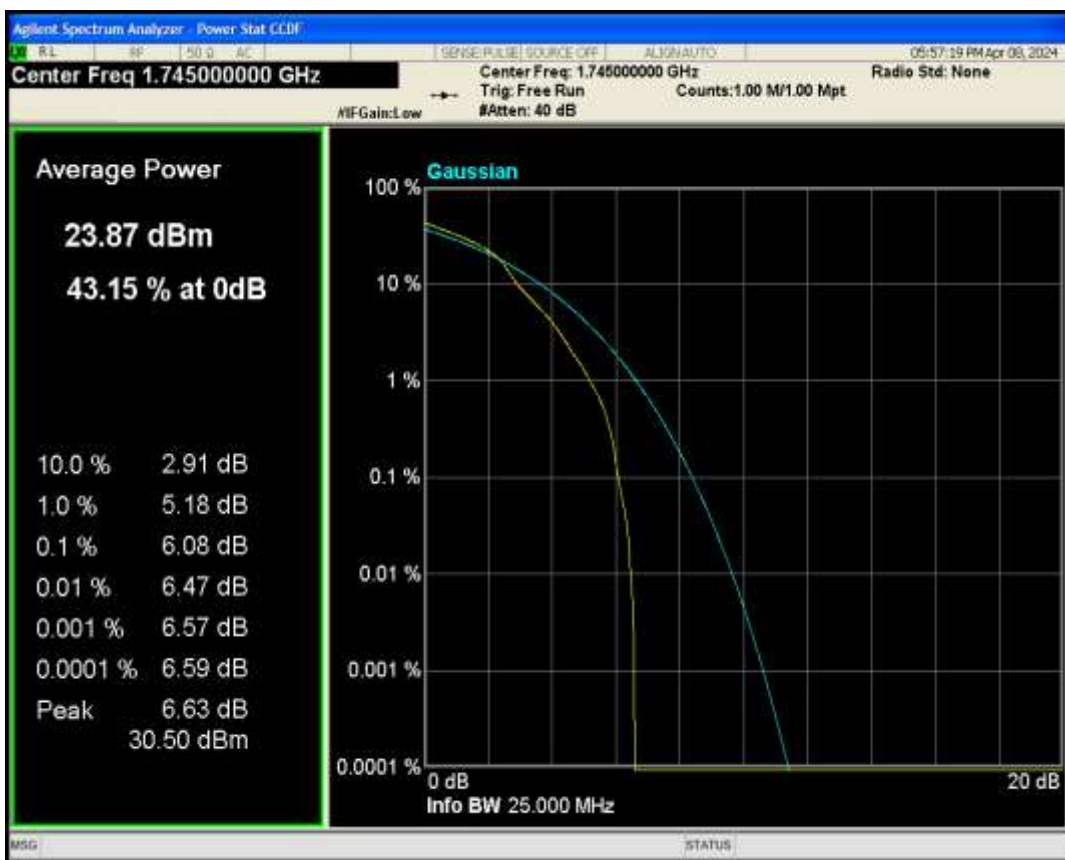
Band66 QPSK BW=5MHz Channel=132322 RB Size=1 Position=#0
