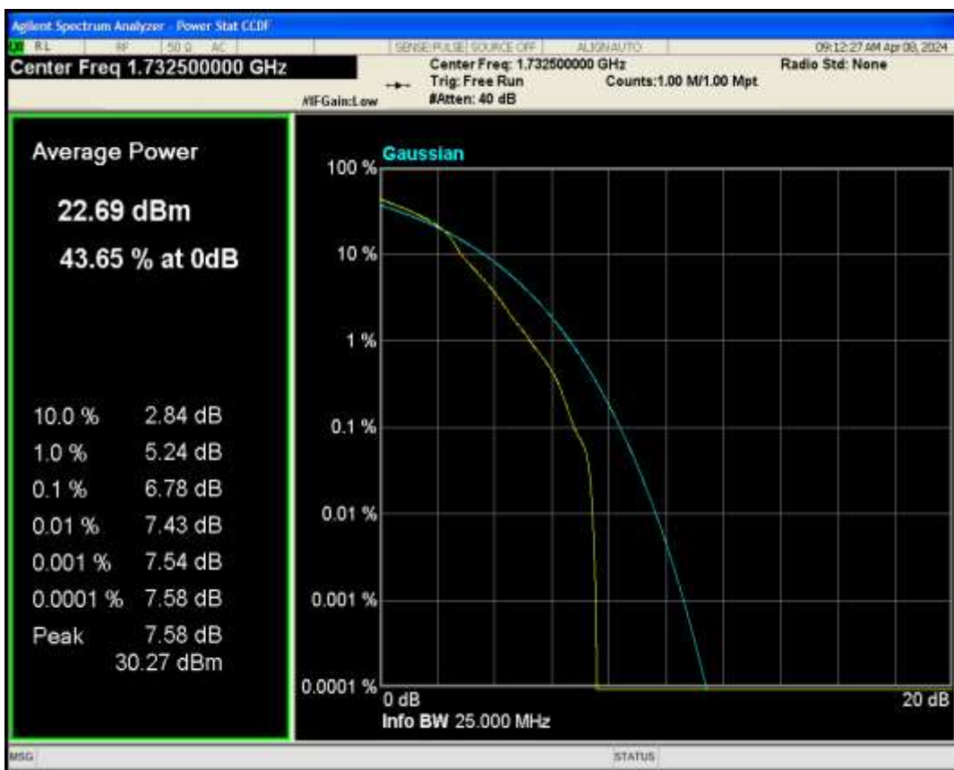
Band4 QPSK BW=15MHz Channel=20175 RB Size=1 Position=#0
