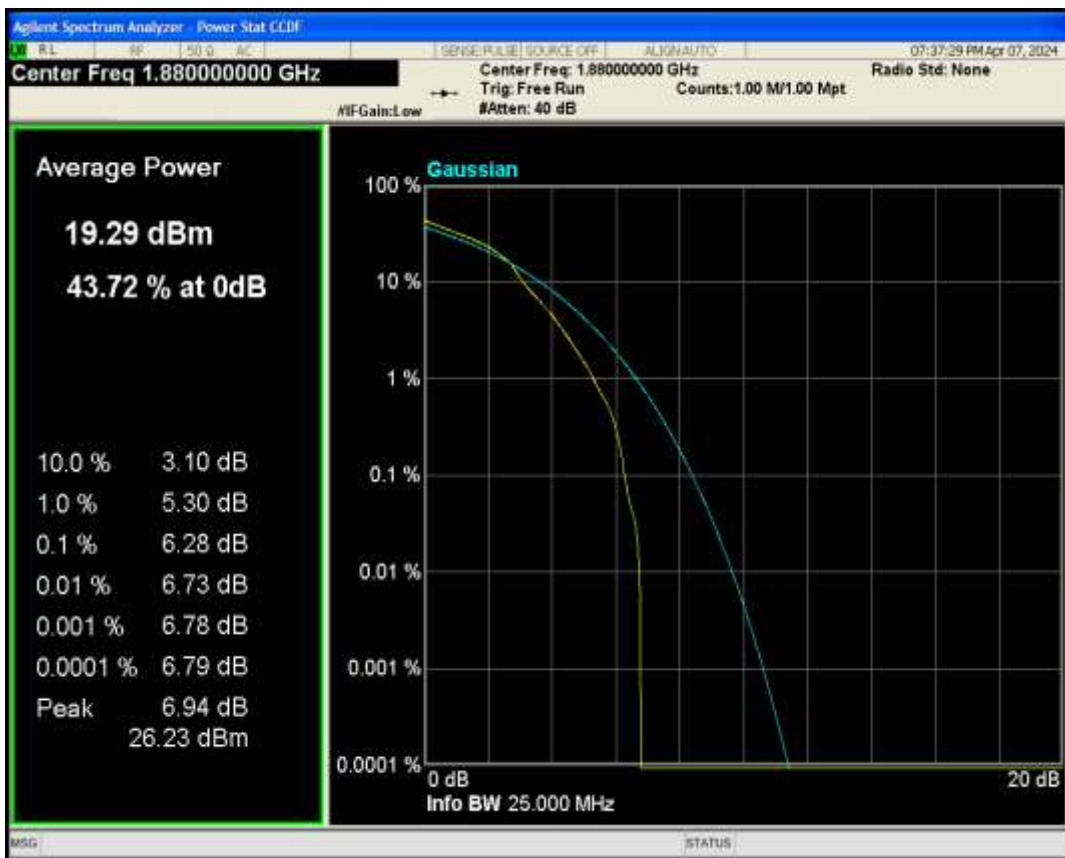
Band2 QPSK BW=3MHz Channel=18900 RB Size=1 Position=#0
