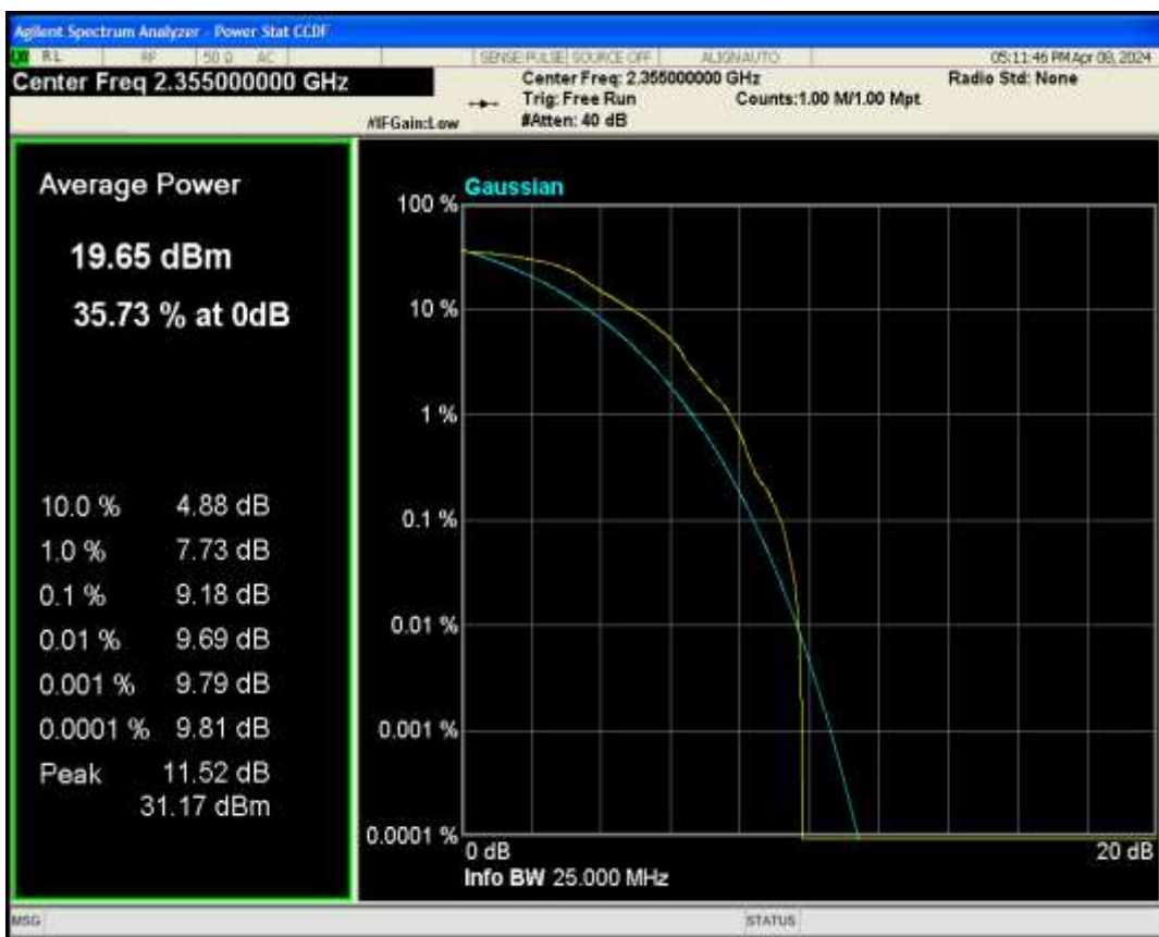
Band40b QAM16 BW=5MHz Channel=39200 RB Size=1 Position=#0
