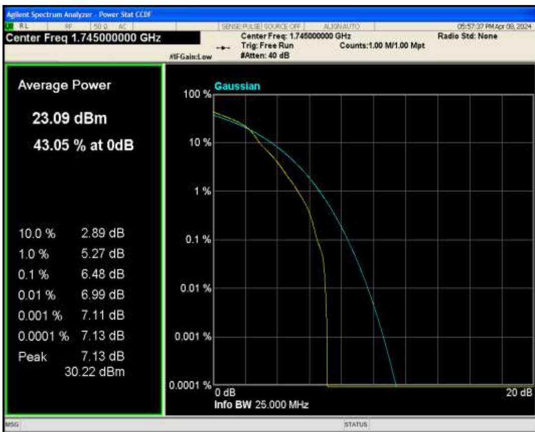
Band66 QPSK BW=15MHz Channel=132322 RB Size=1 Position=#0
