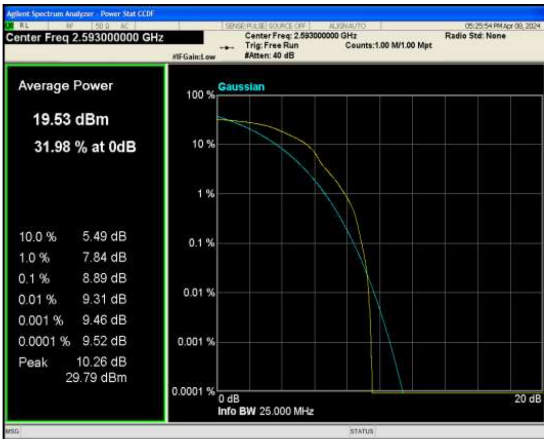
Band41 QPSK BW=10MHz Channel=40620 RB Size=1 Position=#0
