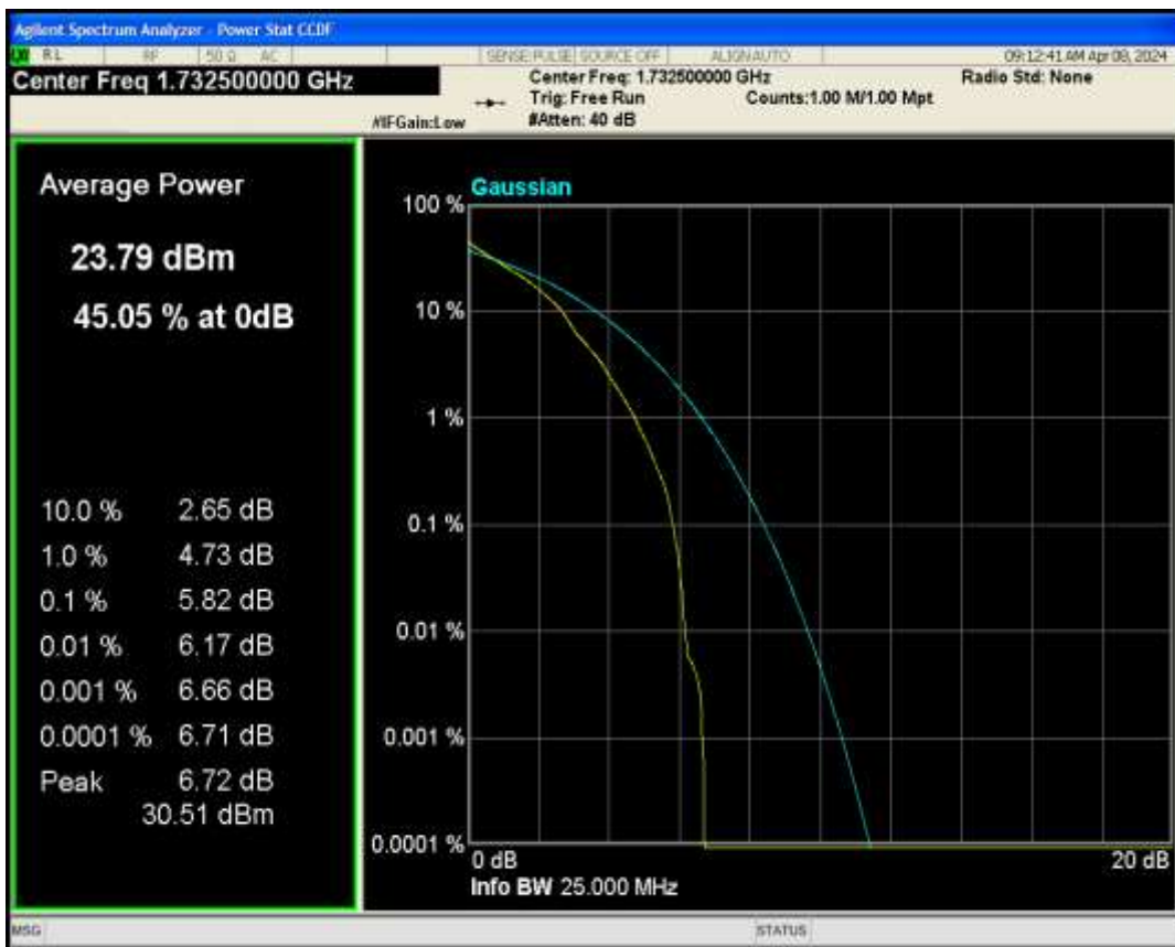
Band4 QAM16 BW=15MHz Channel=20175 RB Size=1 Position=#0
