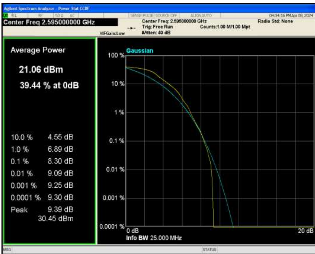
Band38 QAM16 BW=15MHz Channel=38000 RB Size=1 Position=#0
