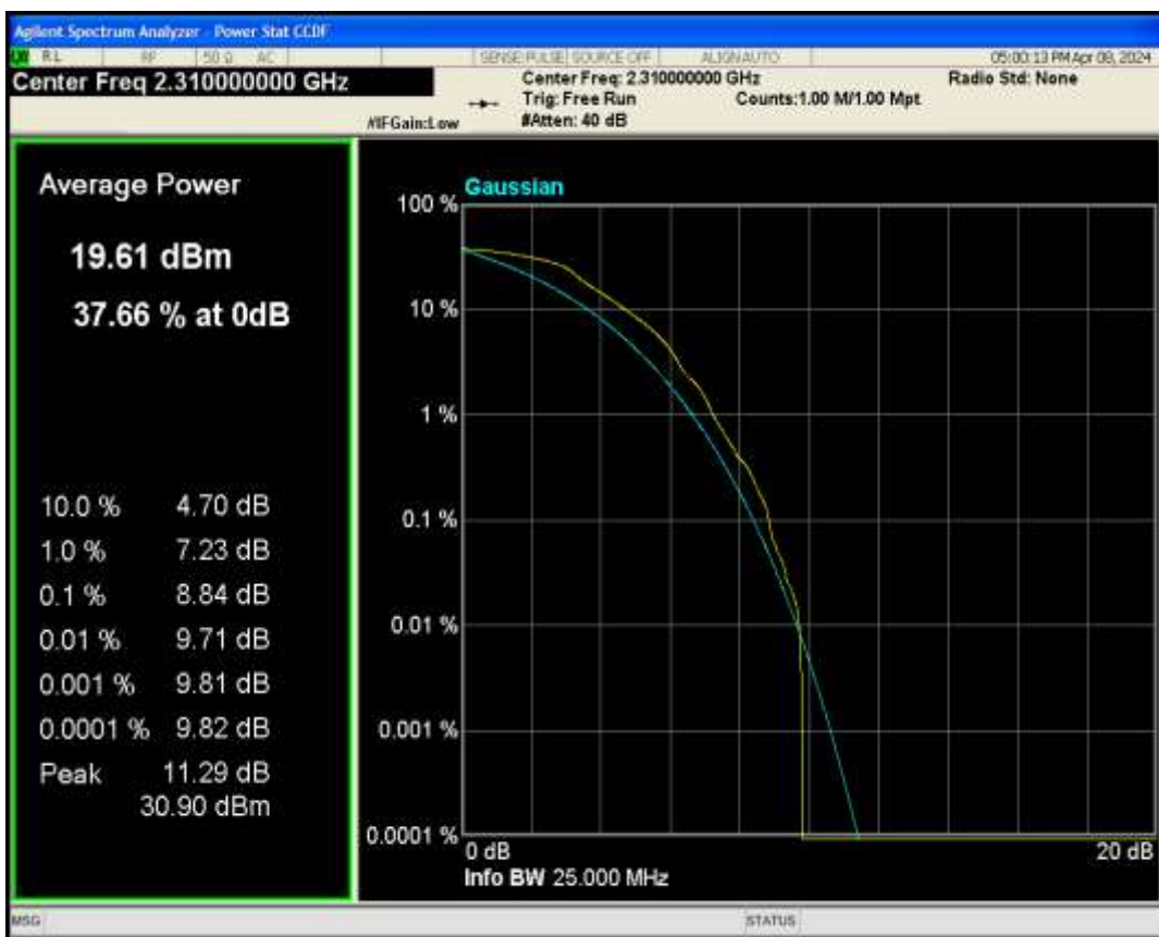
Band40a QAM16 BW=10MHz Channel=38750 RB Size=1 Position=#0
