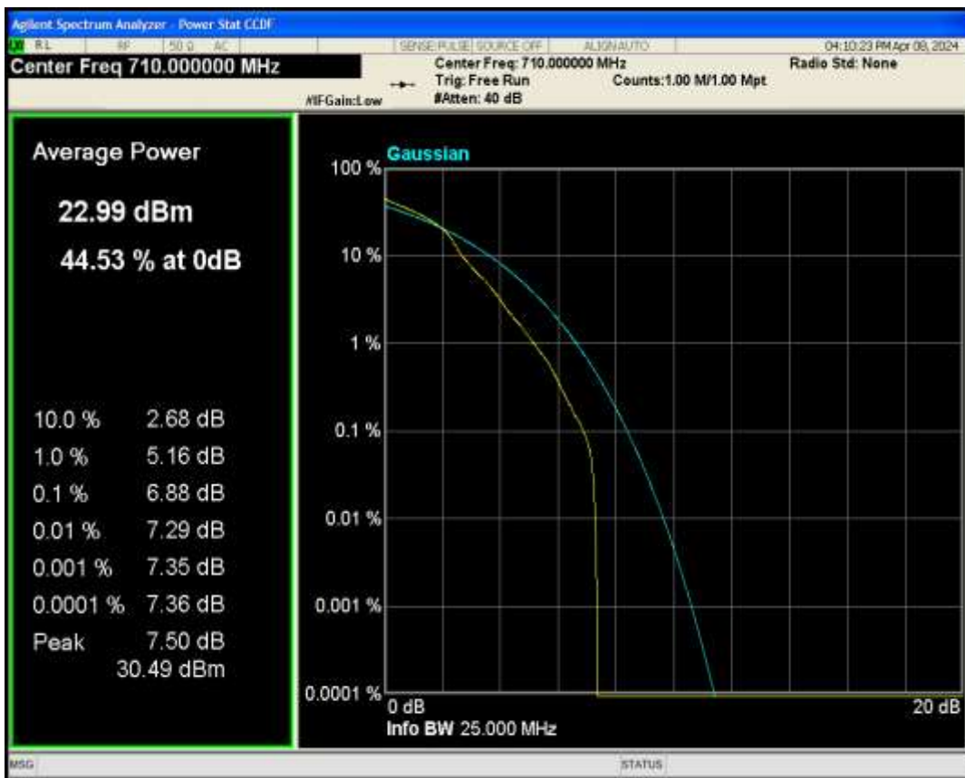
Band17 QPSK BW=10MHz Channel=23790 RB Size=1 Position=#0
