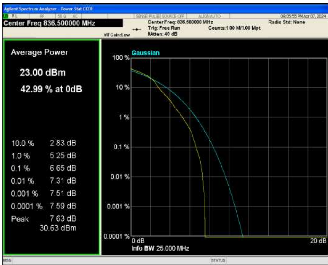
Band5 QPSK BW=5MHz Channel=20525 RB Size=1 Position=#0
