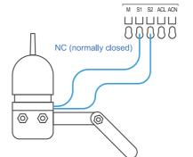
wires into the S1 and S2 terminal slots.
