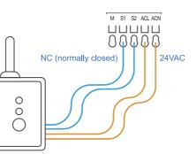
Insert the normally closed and common (1) Insert the normally closed and common wires into the S1 and S2 terminal slots. (2) Insert the 24VAC leads into the ACL and ACN terminal slots.
