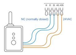
Insert the normally closed and common wires into the S1 and S2 terminal slots.
