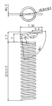
Material : steel Wire Diameter:0.5±0.1mm Number of turns:18.5 Length:20±0.5 mm
