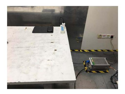
Photos of Radiation Emission Measurement
