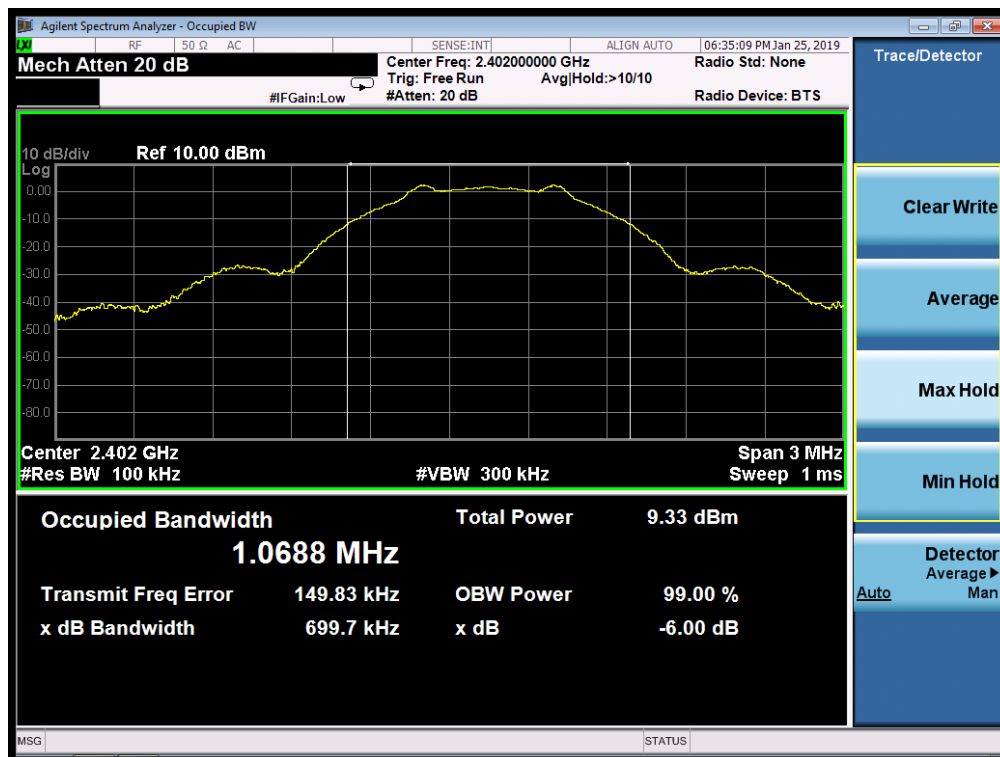
TEST PLOT OF BANDWIDTH FOR LOW CHANNEL
