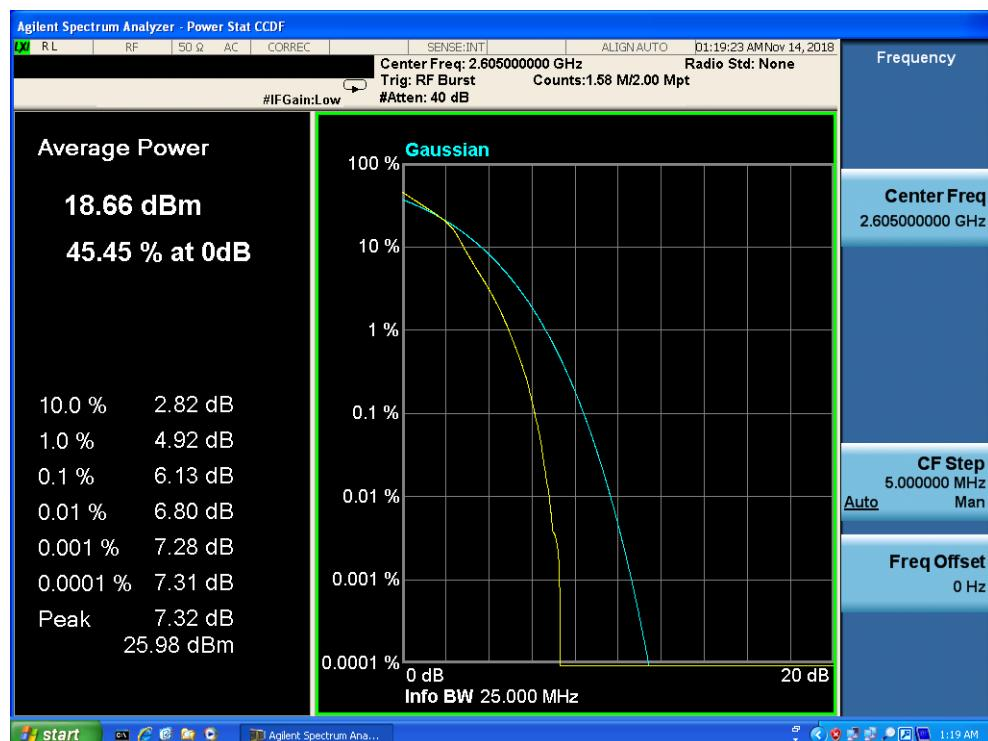
Band 41, UL Channel 40740, UL Frequency 2605.0, BW 10.0, NO. RB 1, RB POS. Low, QPSK
