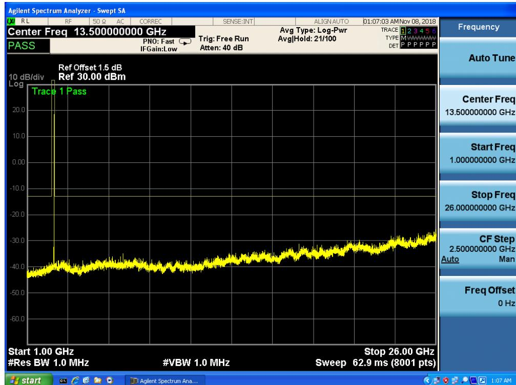
Band 41, UL Channel 41215, UL Frequency 2652.5, BW 5.0, NO. RB 25, RB POS. Low, 16-QAM
