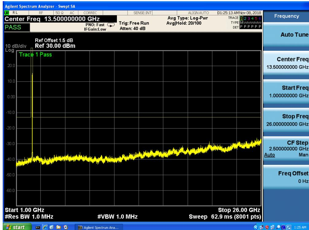
Band 41, UL Channel 41165, UL Frequency 2647.5, BW 15.0, NO. RB 75, RB POS. Low, 16-QAM
