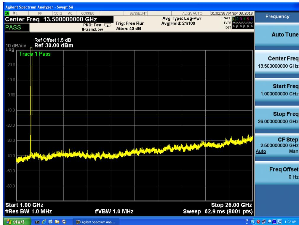
Band 41, UL Channel 40265, UL Frequency 2557.5, BW 5.0, NO. RB 25, RB POS. Low, 16-QAM
