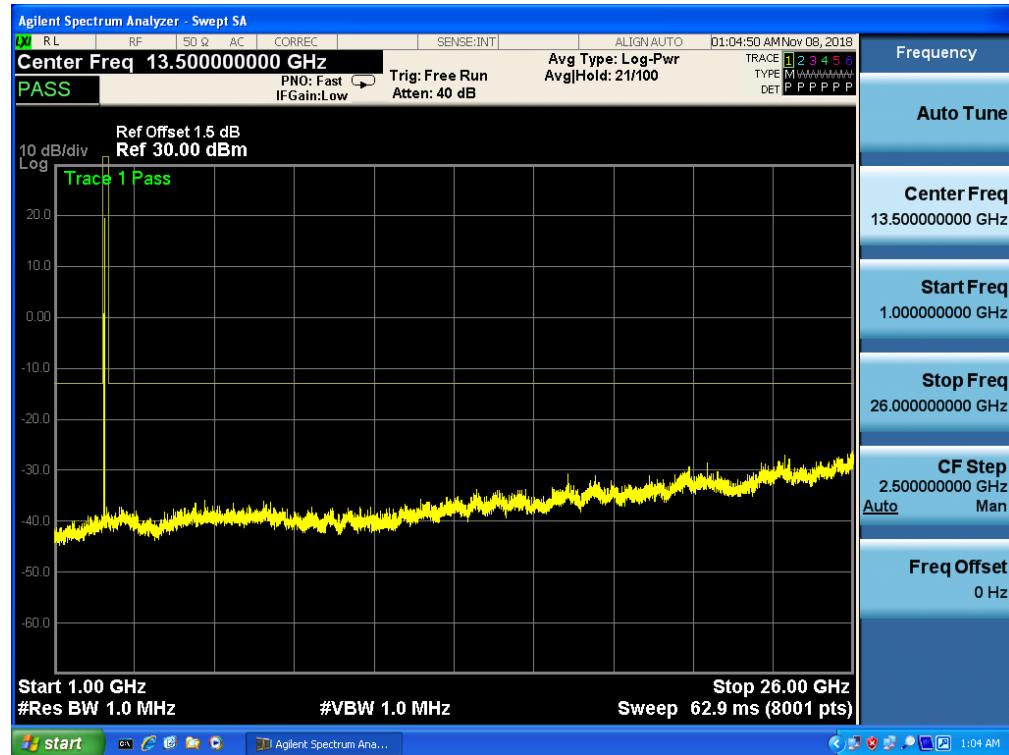
Band 41, UL Channel 41215, UL Frequency 2652.5, BW 5.0, NO. RB 25, RB POS. Low, QPSK
