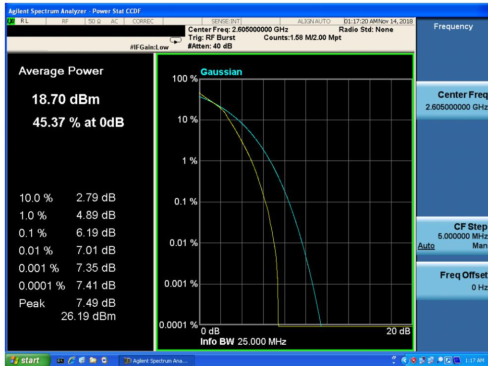
Band 41, UL Channel 40740, UL Frequency 2605.0, BW 15.0, NO. RB 1, RB POS. Low, QPSK
