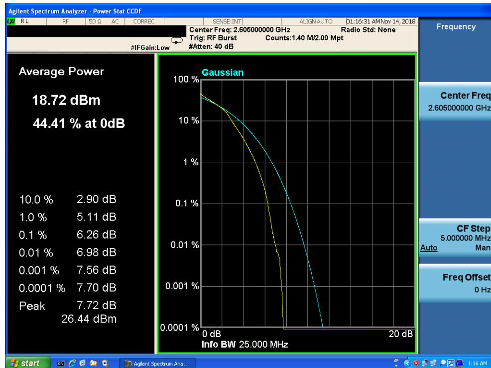
Band 41, UL Channel 40740, UL Frequency 2605.0, BW 20.0, NO. RB 1, RB POS. Low, QPSK
