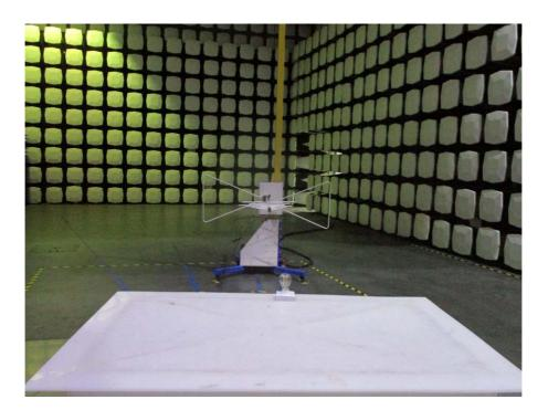
1.3 Radiated Spurious Emissions Test Setup
