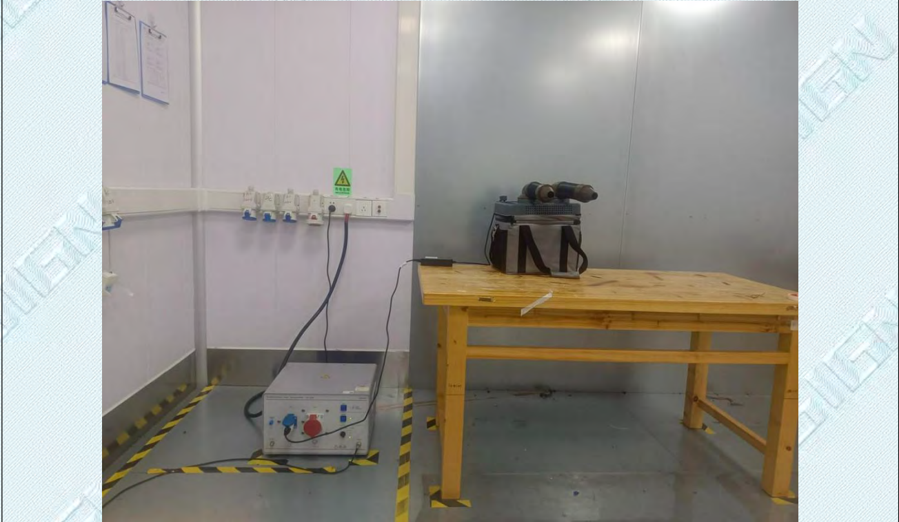
Conducted Emission at AC power line
