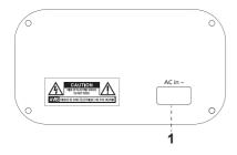
1 AC IN: Connect the AC cable to get power supply.
