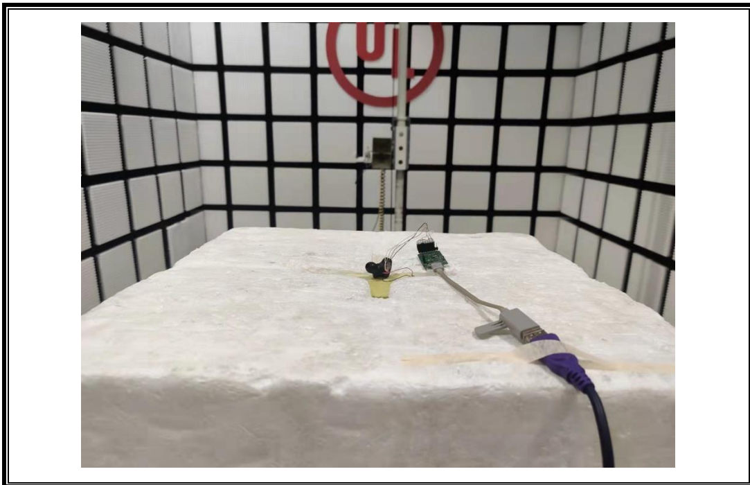
POWERLINE CONDUCTED EMISSIONS MEASUREMENT SETUP
