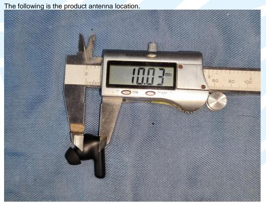
The minimum contact distance is 10.03 mm. So, the 10 mm separation distance applies.
