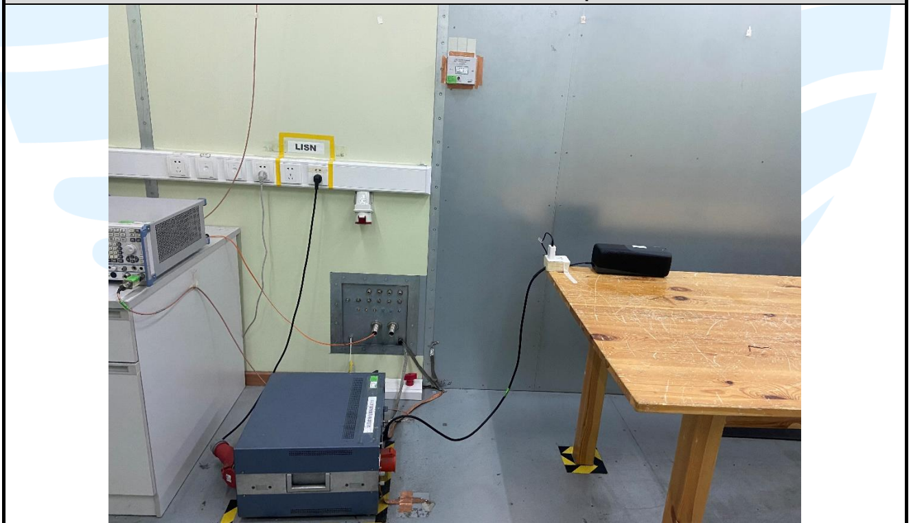
Conducted Emission Test Setup
