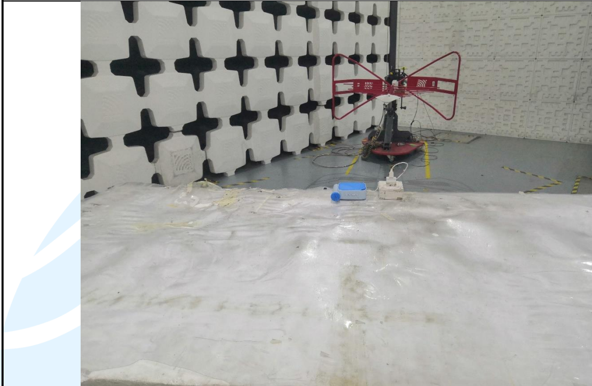
Radiated emission Test Setup (30 MHz~1 GHz)
