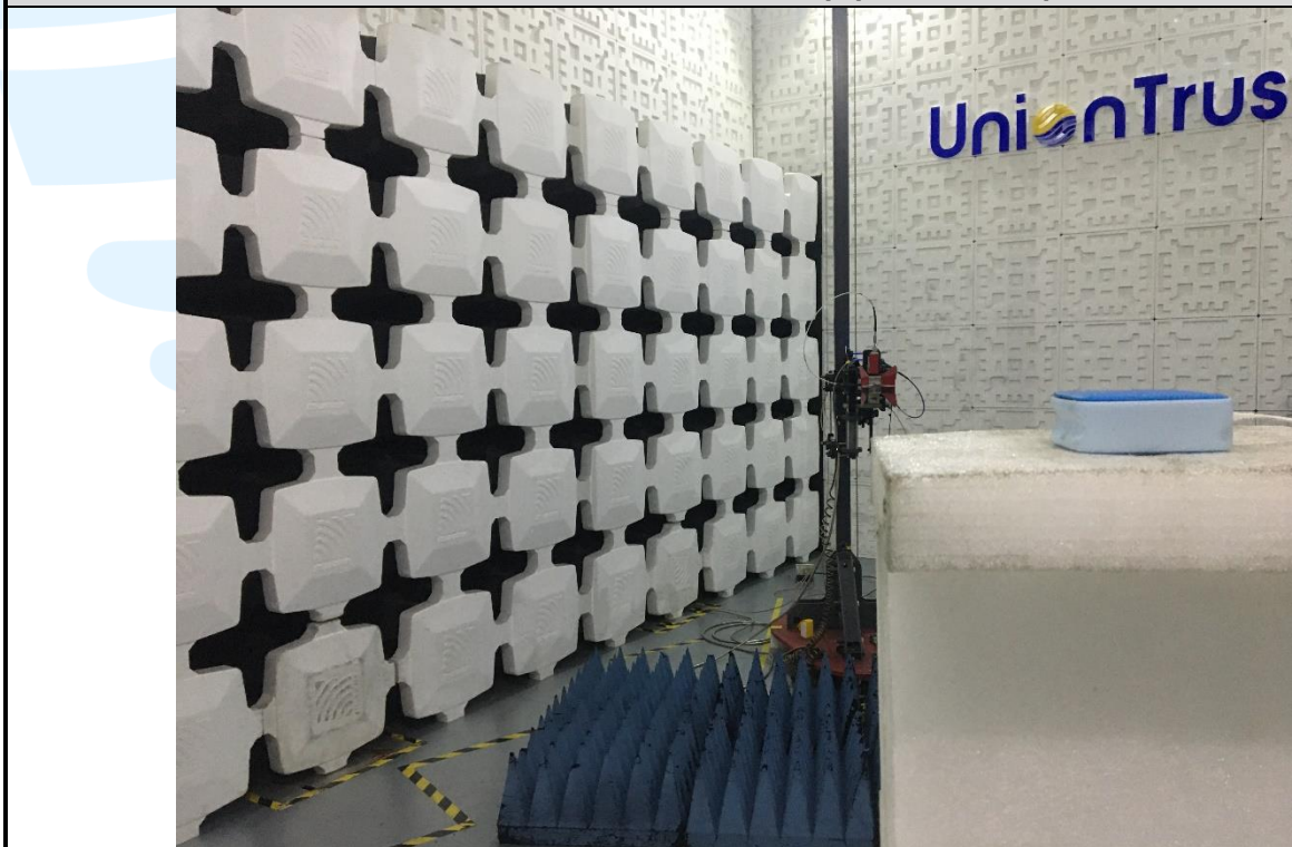
Radiated emission Test Setup (Above 1 GHz)
