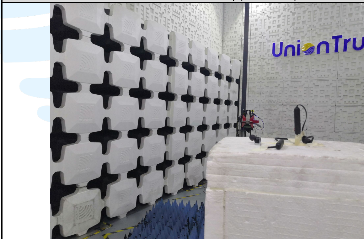
Radiated emission Test Setup (Above 1 GHz)
