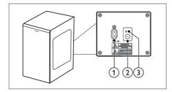
(1) AC~ socket Connect to the power supply.
