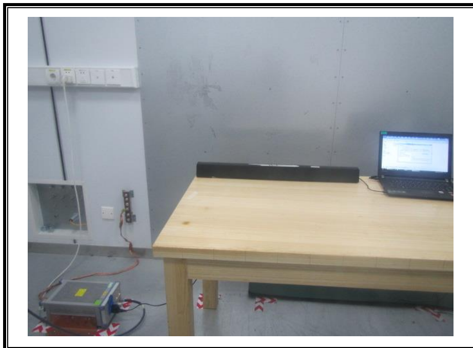
POWERLINE CONDUCTED EMISSIONS MEASUREMENT SETUP
