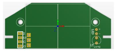
Power on,O pin after a low-level lasts for 1 minute, it becomes high-level. If the environment illumination below  $15\pm3$  Lux and there are something moving in it's detection range, then the O pin becomes low-level for 5 minutes. During this 5 minutes, if the module redetects a motion, it also lasts 5 minutes else the O pin turns to high level after 5 minutes.
