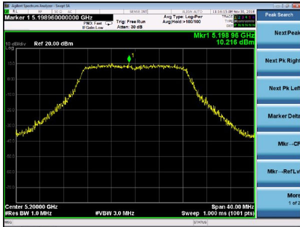
ANTA (5200 MHz) PSD plot on channel 01
