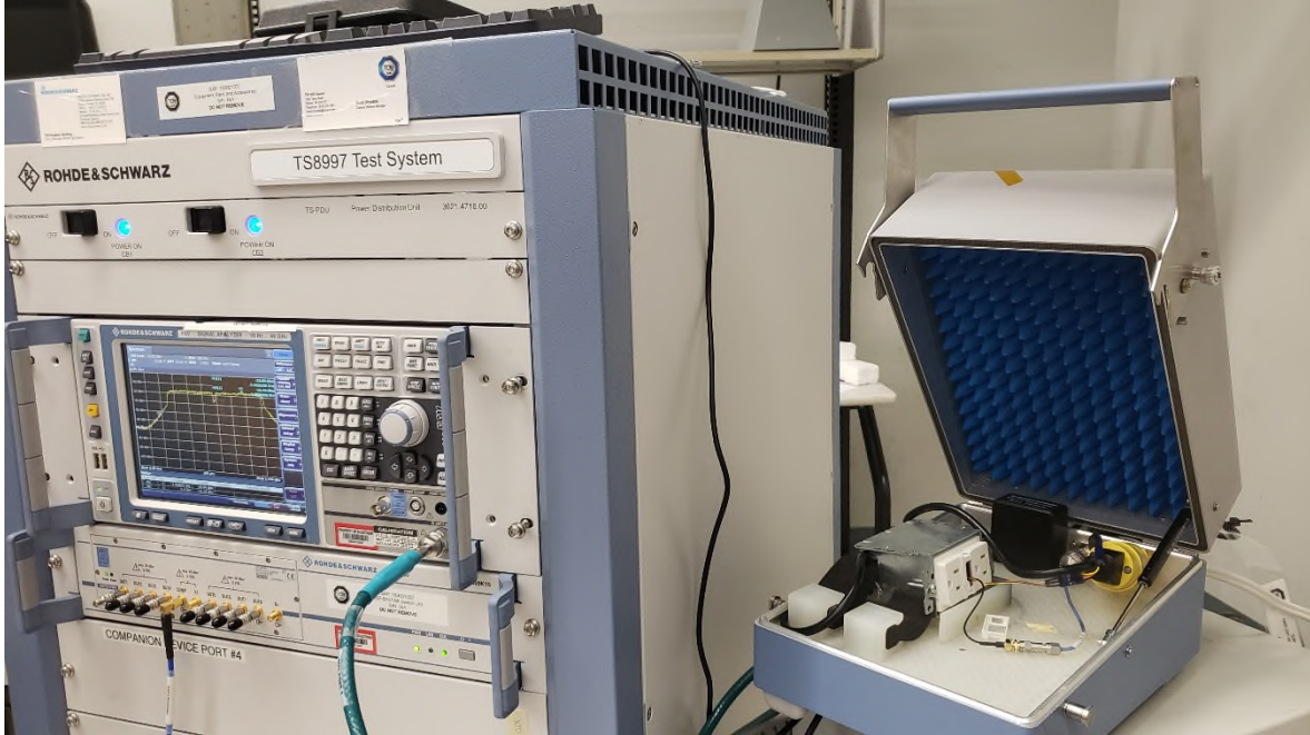
Figure 5 – Antenna port conducted emissions
