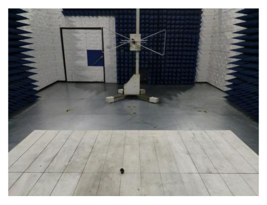
RADIATED EMISSION TEST SETUP ABOVE 1GHZ
