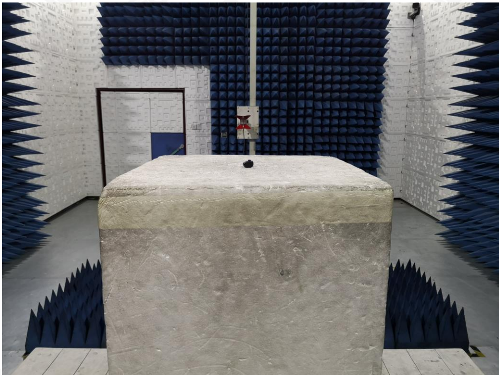
RADIATED EMISSION TEST SETUP ABOVE 1GHZ
