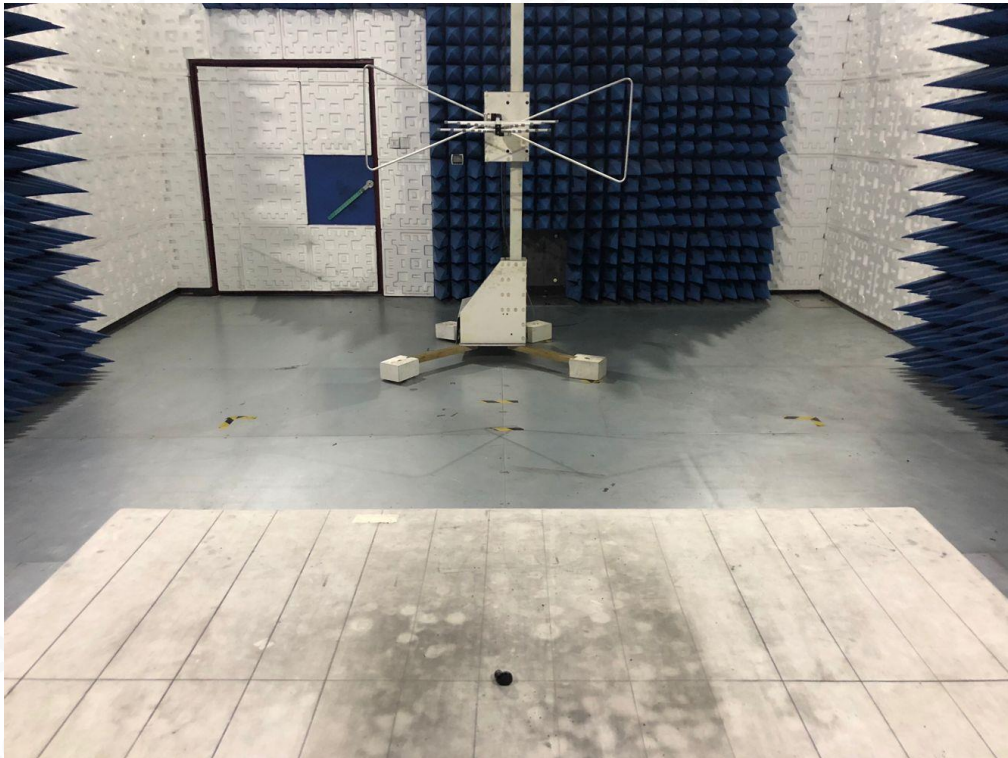
RADIATED EMISSION TEST SETUP ABOVE 1GHZ
