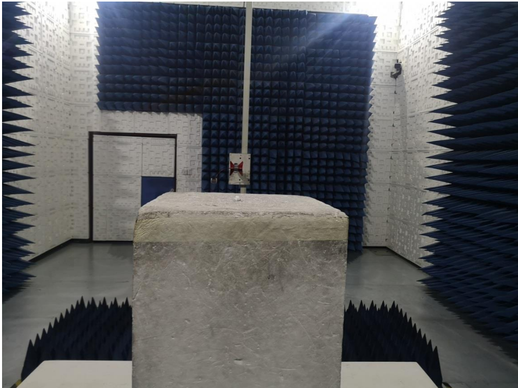
RADIATED EMISSION TEST SETUP ABOVE 1GHz
