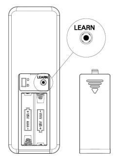
Please note that the transmitter can learn in multiple receiver, when doing learning process please make sure not learn in other receiver. Suggest to separate power switches of fans in 2 meter range.
