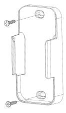
Installation of Transmitter Wall Mount Holder with two screws
