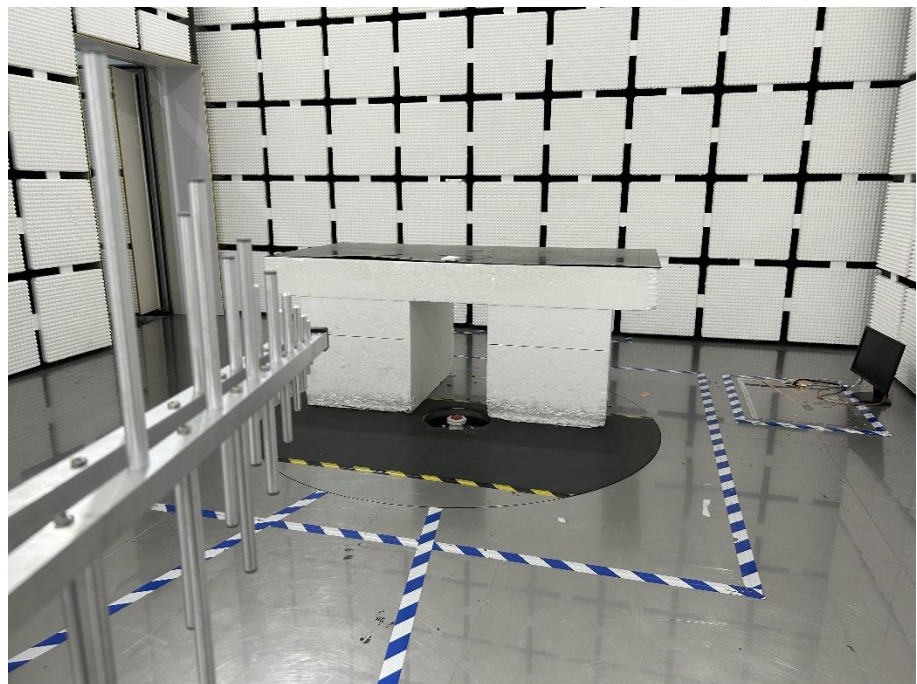
Radiation Emission Test Setup (30MHz to 1GHz)
