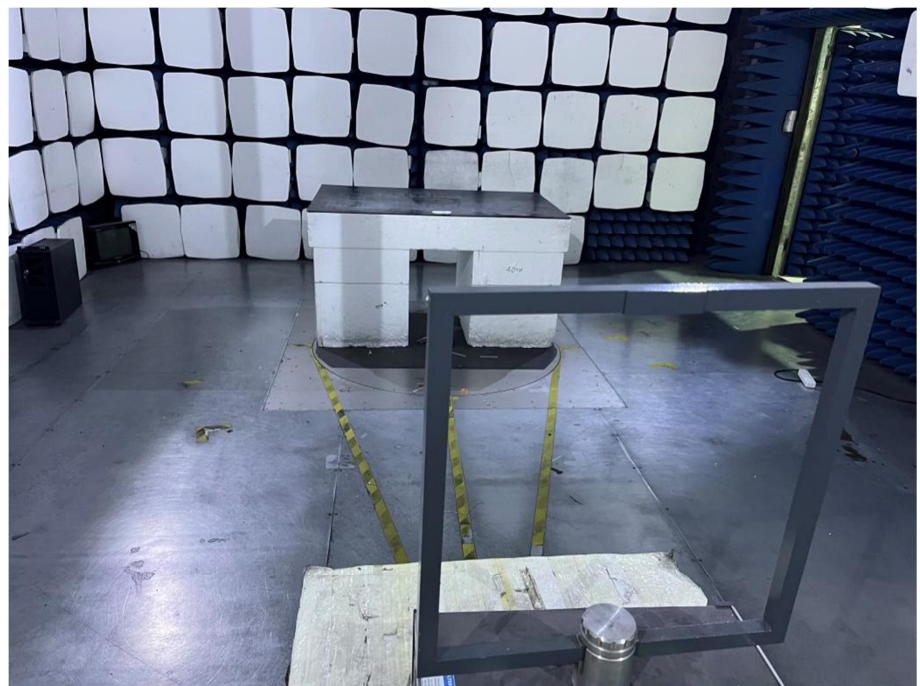
Radiation Emission Test Setup (Below 30MHz)
