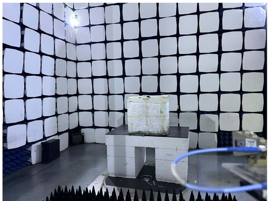
Radiation Emission Test Setup (Above 18GHz)
