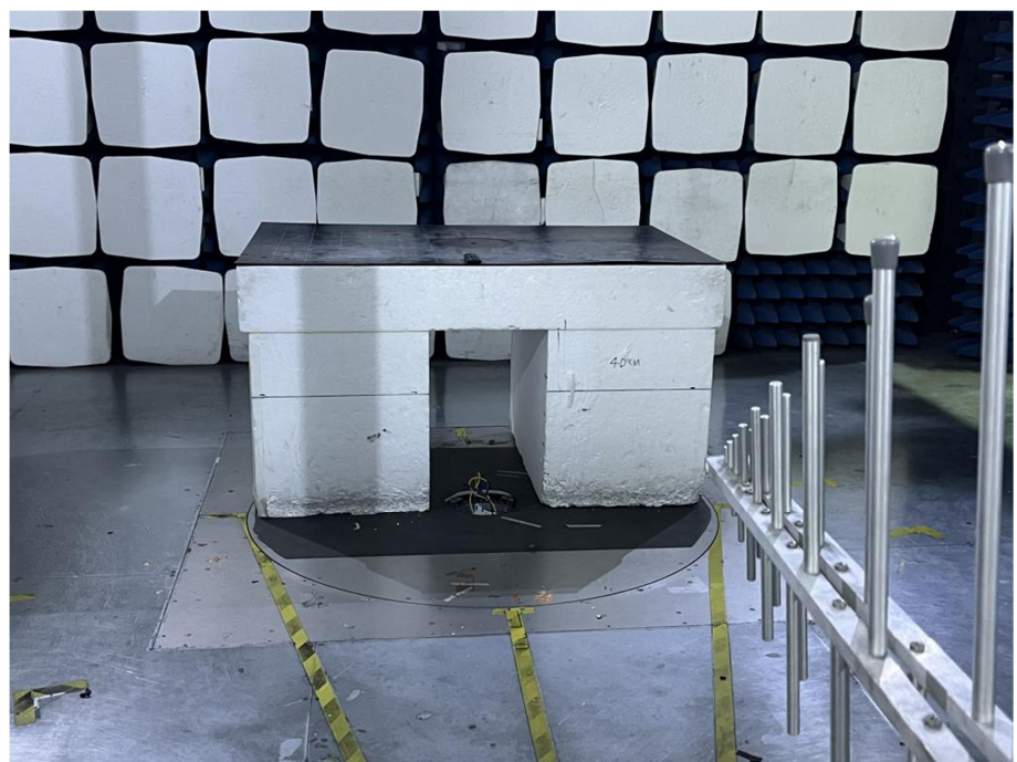
Radiation Emission Test Setup (30MHz to 1GHz)
