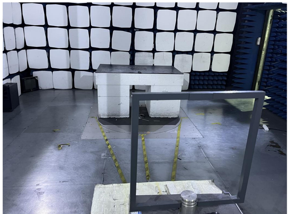
Radiation Emission Test Setup (Below 30MHz)
