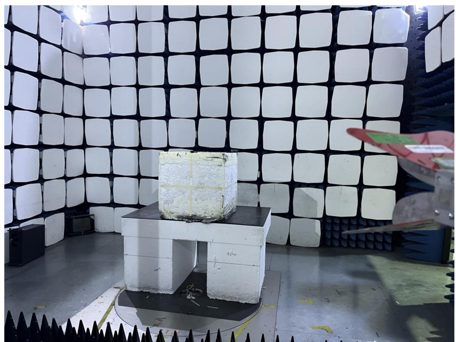
Radiation Emission Test Setup (1GHz to 18GHz)
