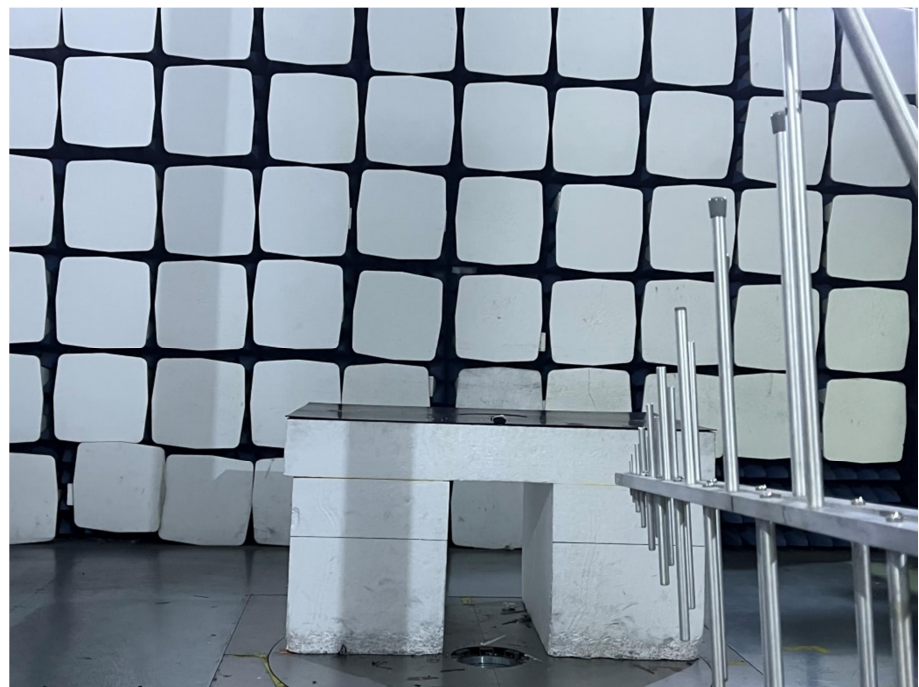
Radiation Emission Test Setup (30MHz to 1GHz)
