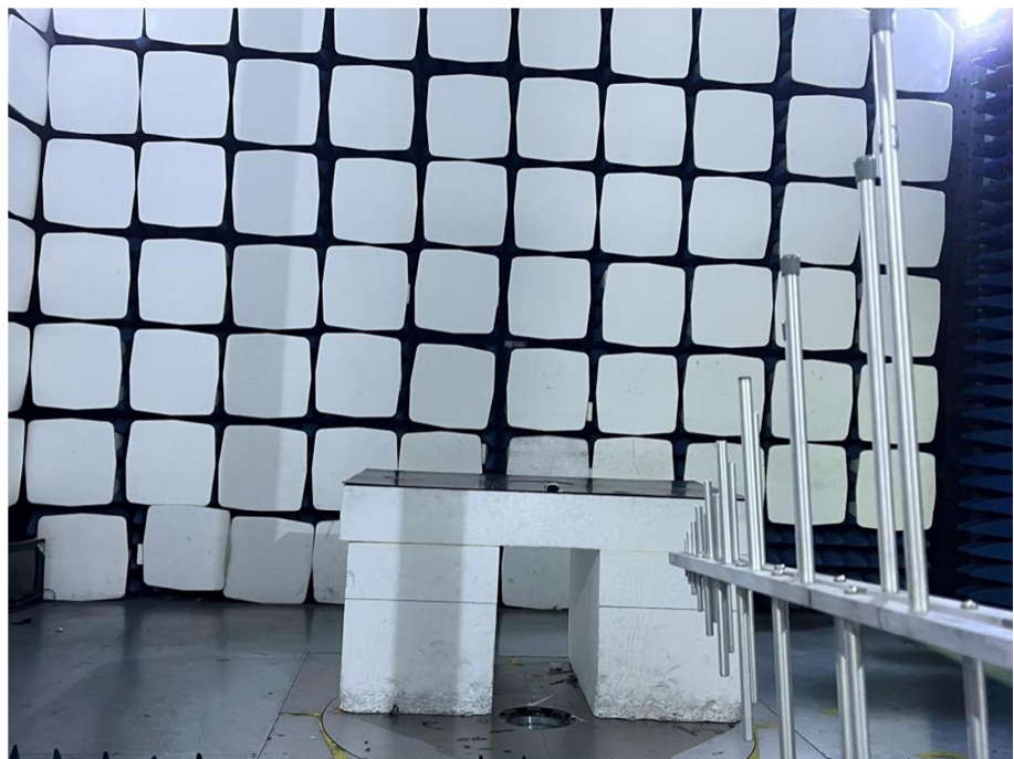
Radiation Emission Test Setup (30MHz to 1GHz)
