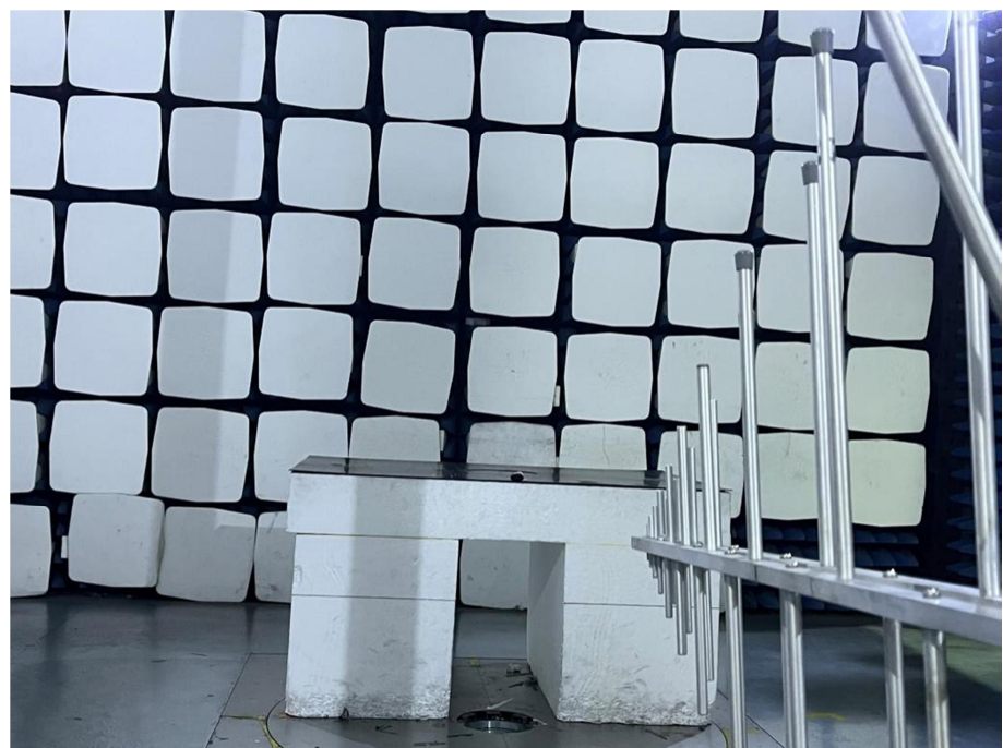
Radiation Emission Test Setup (30MHz to 1GHz)
