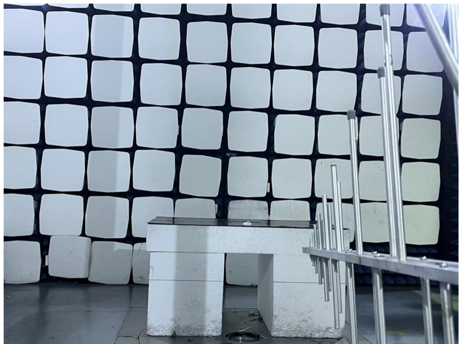
Radiation Emission Test Setup (30MHz to 1GHz)
