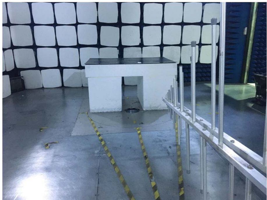
Radiation Emission Test Setup (30MHz to 1GHz)
