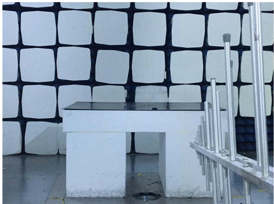
Radiation Emission Test Setup (30MHz to 1GHz)
