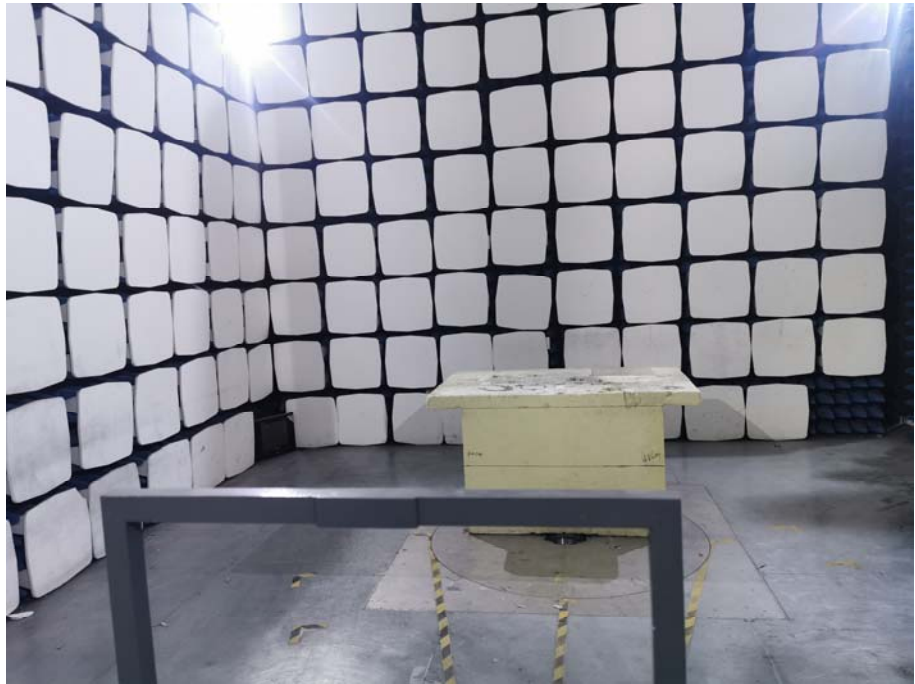
Radiation Emission Test Setup (Below 30MHz)
