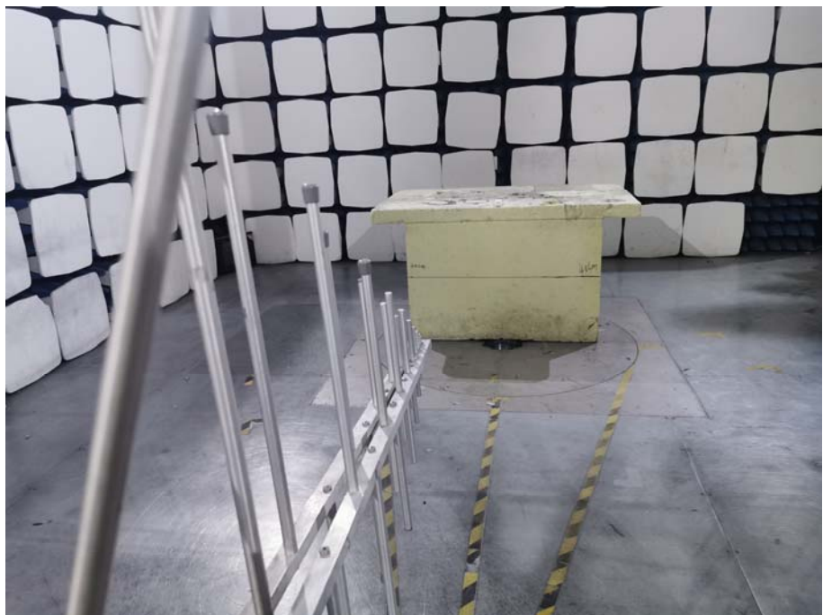
Radiation Emission Test Setup (30MHz to 1GHz)
