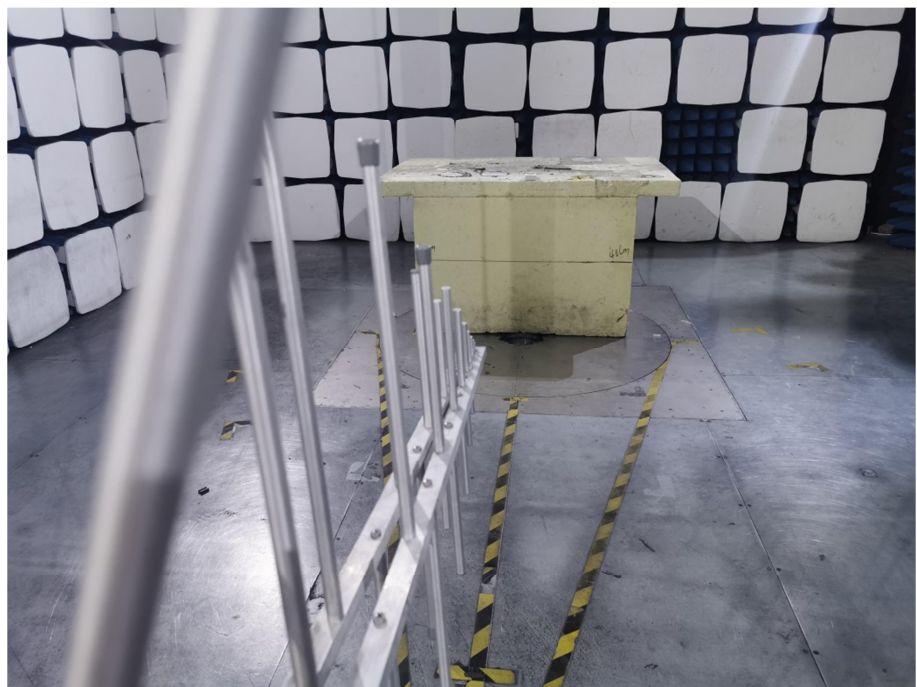
Radiation Emission Test Setup (30MHz to 1GHz)
