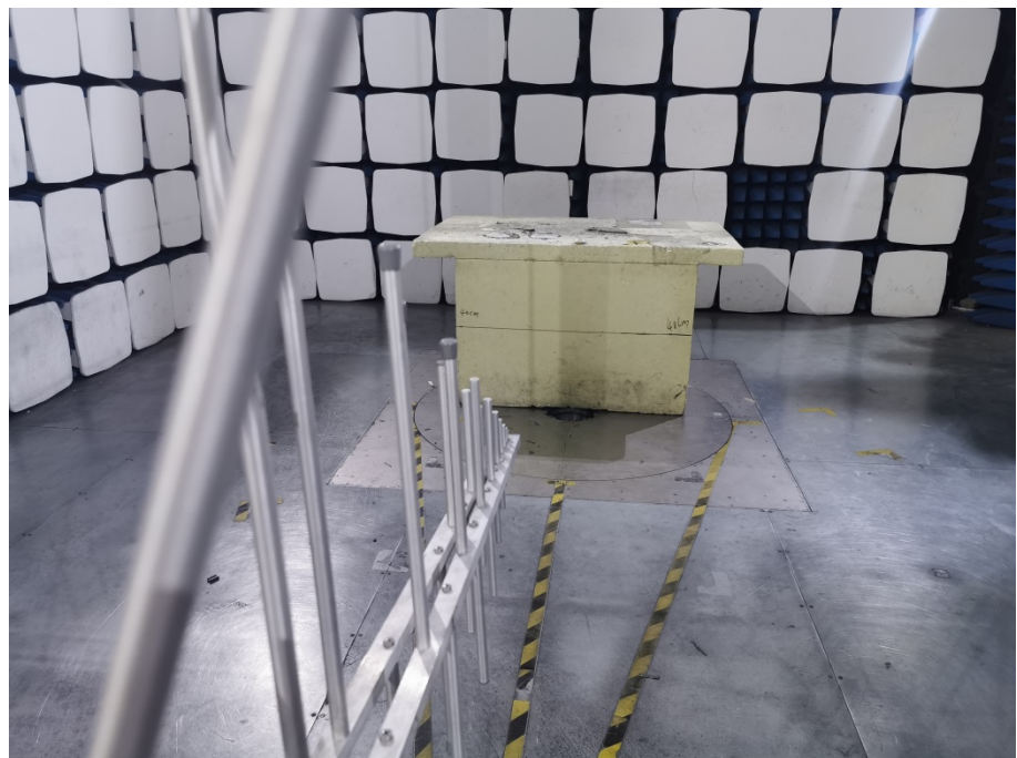
Radiation Emission Test Setup (30MHz to 1GHz)
