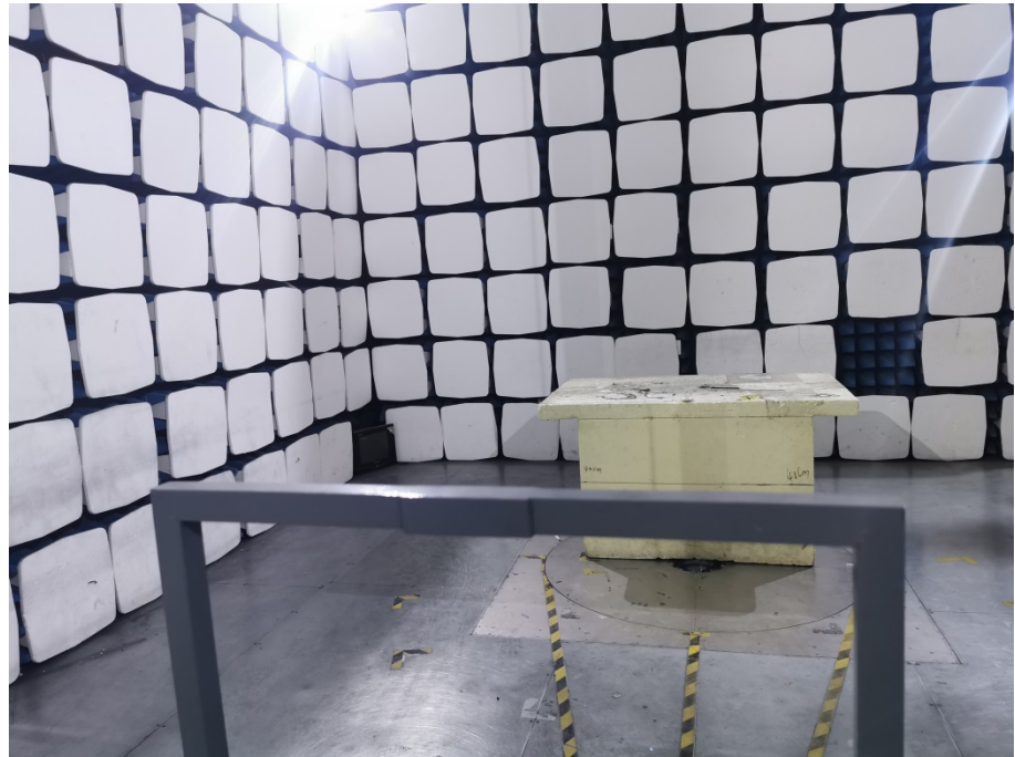
Radiation Emission Test Setup (Below 30MHz)
