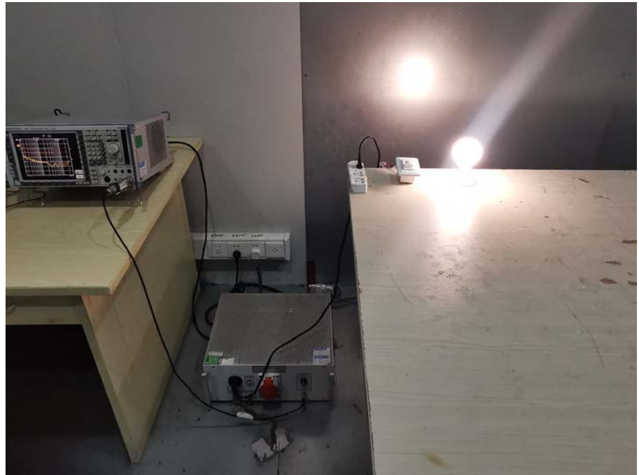
Conducted Emission Test Setup
