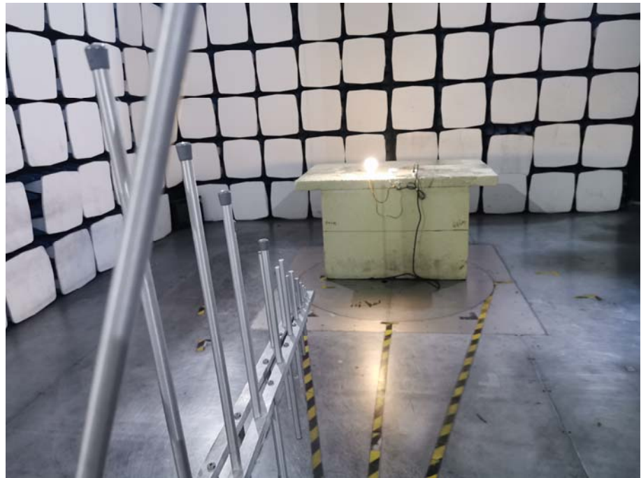
Radiation Emission Test Setup (30MHz to 1GHz)
