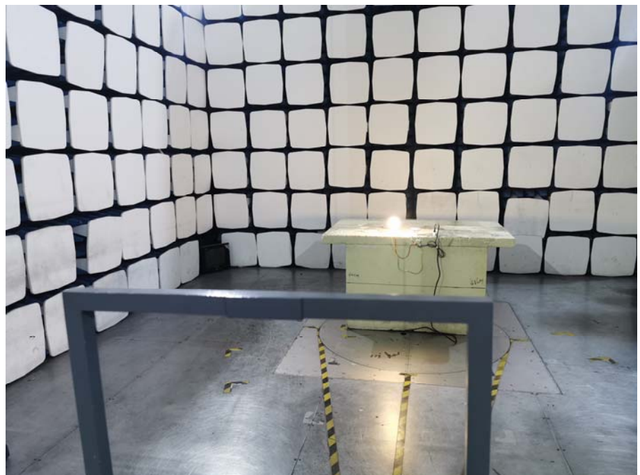
Radiation Emission Test Setup (Below 30MHz)
